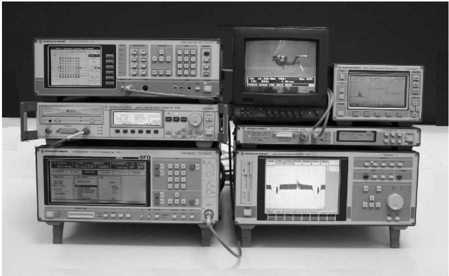
Fig. 21.33. DVB-T transmission link with MPEG-2 test generator DVRG (center left), DVB-T test transmitter SFQ (bottom left), DVB-T test receiver EFA (top left), MPEG-2 test decoder DVMD (center right) and TV monitor, video analyzer VSA and “601” analyzer VCA (Rohde&Schwarz).
