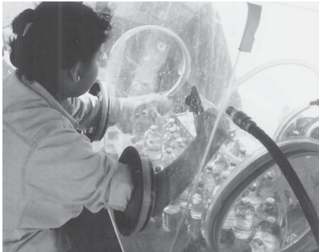
Figure 13.3. Portable hoods are used to collect groundwater for evaluation of bacteria and water quality; Keka C. Biswas is placing groundwater collected under anaerobic conditions in anaerobic bottles (photograph provided by Larry Barton).
