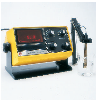
A pH meter showing that the pH of 0.1 M \text{NH}_4\text{Cl} is 5.13.
