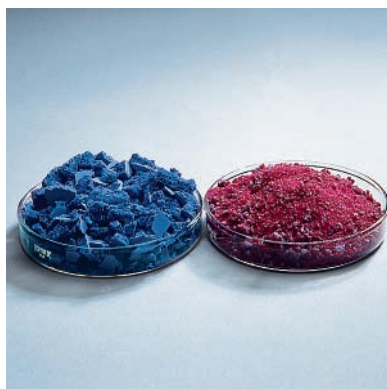
Blue anhydrous cobalt(II) chloride and pink hydrated cobalt(II) chloride. Since the reaction CoCl_2(s) + 6H_2O(g) \longrightarrow CoCl_2 \cdot 6H_2O(s) is shifted to the right by water vapor, CoCl_2 is often used in novelty devices to detect humidity.
