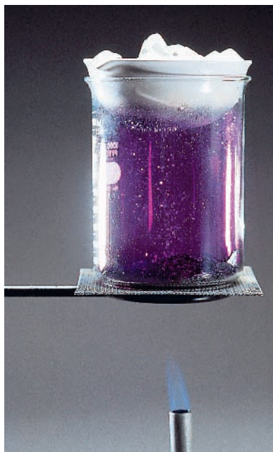
Iodine being heated, causing it to sublime onto an evaporating dish cooled by ice.
