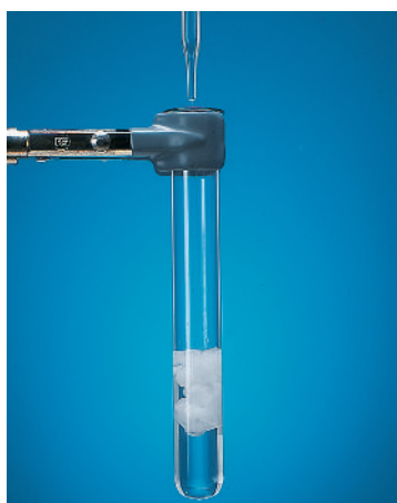
When KI(aq) is added to a solution containing 1.0 \times 10^{-4} M Cu^+ and 2.0 \times 10^{-3} M Pb^{2+} , white CuI(s) precipitates first.
