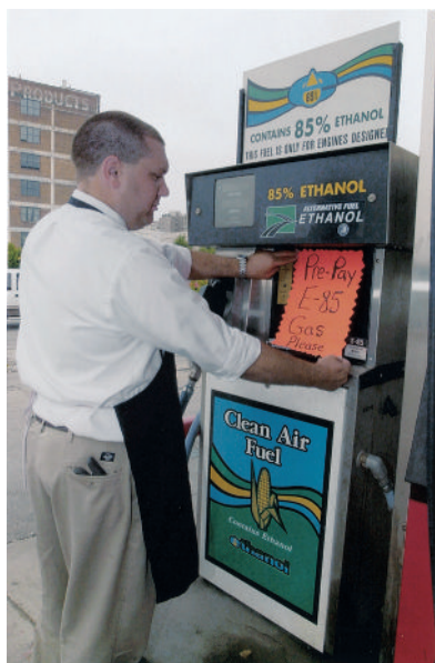
A fuel consisting of 85% ethanol and 15% gasoline is now widely available in the United States.
