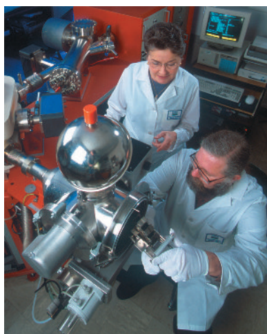
Chemists using a mass spectrometer to analyze for copper in blood plasma.
