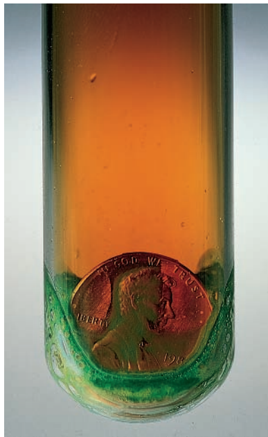
A copper penny reacts with nitric acid to produce NO gas, which is immediately oxidized in air to give reddish brown NO 2 .
