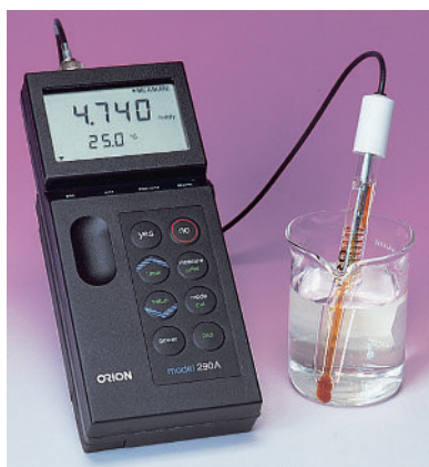
A digital pH meter shows the pH of the buffered solution to be 4.74.
