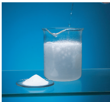
Hydrochloric acid reacts with solid sodium hydrogen carbonate to produce gaseous carbon dioxide.
