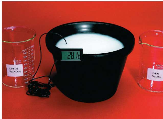
When barium nitrate and sodium sulfate are mixed in an insulated container, they form a white solid \text{BaSO}_4 (barium sulfate), and the temperature changes to 28.1^\circ\text{C} .
