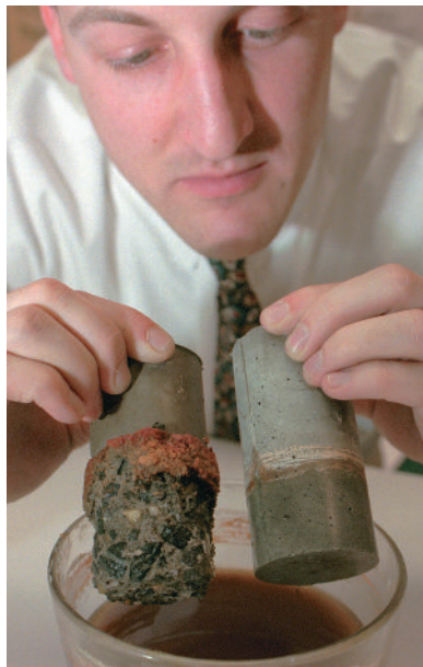
A Drexel University chemist shows that a new form of concrete called ZeoTech (on the right) can withstand soaking in sulfuric acid for 30 days.
