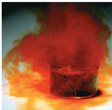
Reddish brown nitrogen dioxide gas streaming from a flask where copper is reacting with concentrated nitric acid.
