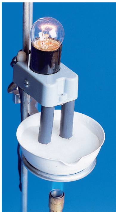
Molten NaCl conducts an electric current, indicating the presence of mobile \text{Na}^+ and \text{Cl}^- ions.
