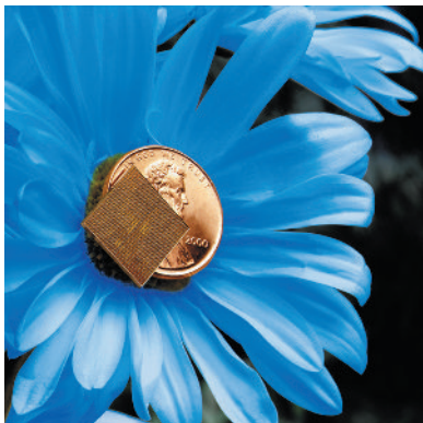
A new IBM microchip featuring silicon on a "blanket" of insulating material to protect it from temperature changes.
