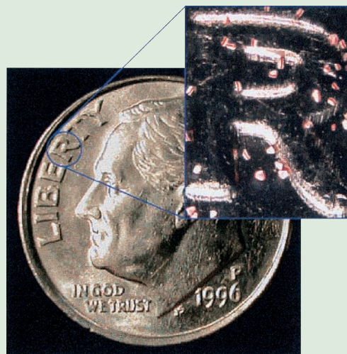
The multilayered plastic particles of Microtaggants (left) can produce over 37 million unique codes that can be used to identify substances. The tiny size of the taggants is shown (right) compared to the "R" on a dime.
