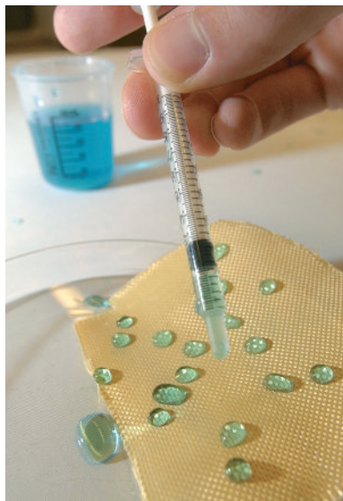
Colored water drops are shown beading on Kevlar fabric treated with a nanoscale water-resistant coating.
