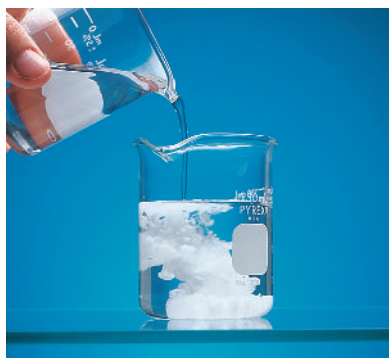
When a solution of \text{NaCl}(aq) is added to a solution of \text{AgNO}_3 , the white solid AgCl forms.
