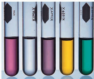
(from left to right) Aqueous solutions containing the metal ions \text{Co}^{2+} , \text{Mn}^{2+} , \text{Cr}^{3+} , \text{Fe}^{3+} , and \text{Ni}^{2+} .
