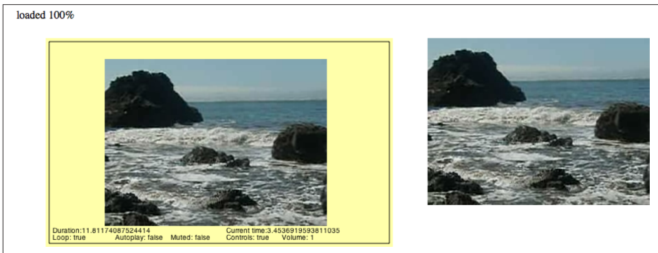
Figure 6-7. Video on the canvas with properties displayed and <video> embed
