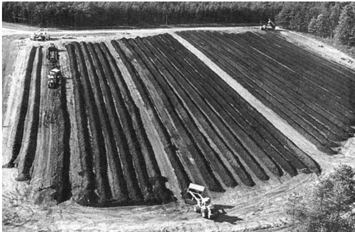
Figure 12.4 Composting. Conventional windrow process. From Benedict et al. (1988). (Courtesy of Noyes Data Corp. and W. D. Burge.)
