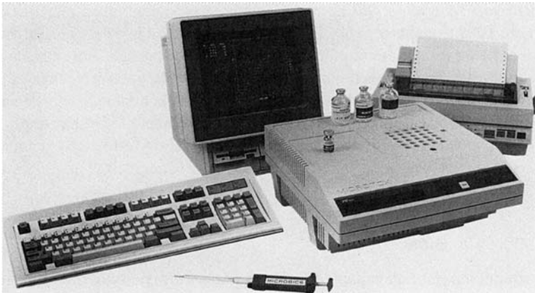
Figure 20.2 Microtox model 500 toxicity analyzer. (Courtesy of A. Bulich, Microbics Corp., Carlsbad, CA.)
