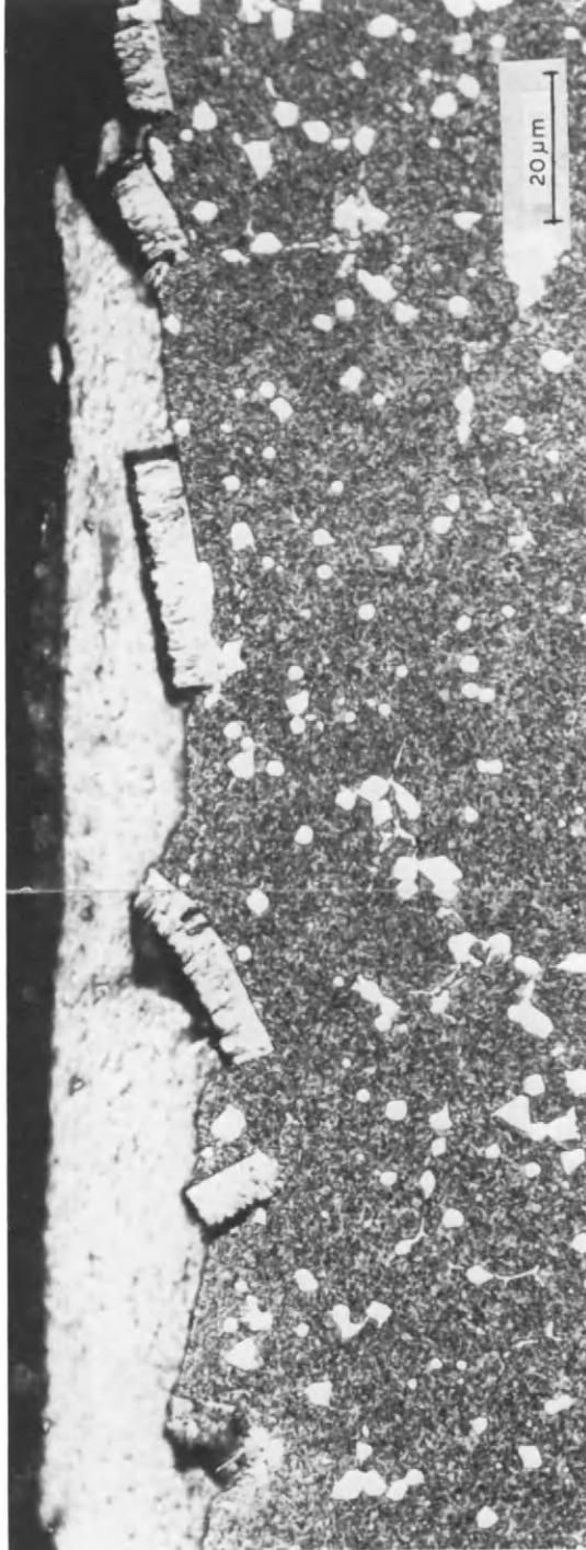
Figure 6.28 Section through rake face of CVD-coated high speed steel tool after cutting steel at high speed. Coating broke when the substrate deformed
