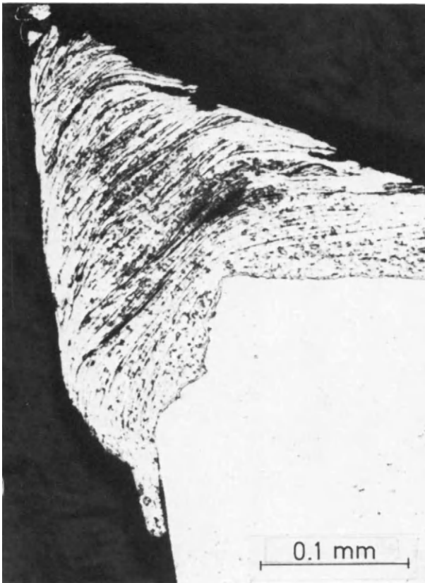
Figure 6.19 Section through cutting edge of high speed steel tool after cutting steel at relatively low speed, showing attrition wear. (After Wright and Trent 12 )
