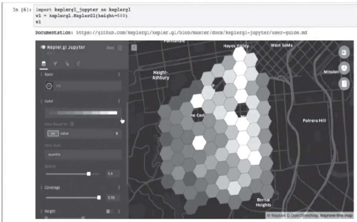
Figure 17-12: The KeplerGL interface for customizing maps works in JupyterLab (courtesy of KeplerGL).
