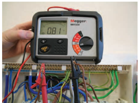
Ends of phase conductor
