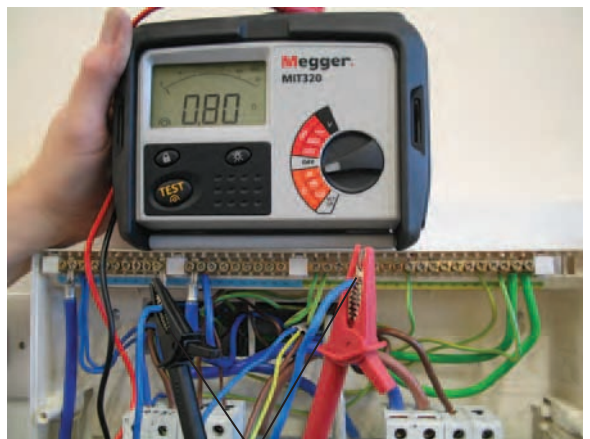
Ends of neutral conductor
