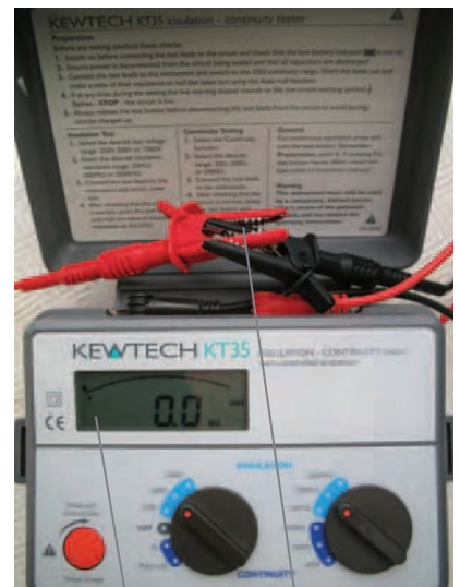
Closed circuit Leads connected
