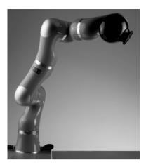
Fig. 1.30. The KUKA LWR robot (courtesy of KUKA Roboter GmbH)
