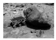
Fig. 1.35. The Sojourner rover was deployed by the Pathfinder lander and explored  $250 \text{ m}^2$  of Martian soil in 1997 (courtesy of NASA)
