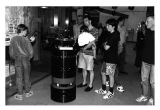
Fig. 1.38. Rhino, employing the synchro-drive mobile base B21 by Real World Interface, was one of the first robots for museum guided tours (courtesy of Deutsches Museum Bonn)
