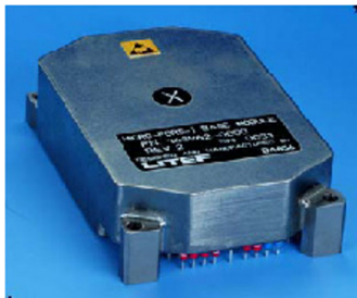
Figure 8.32: Fiber-optic gyroscope and tetrahedron gyro assembly.
