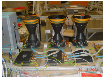
Figure 5.12: Star trackers in CryoSat FlatSat. © Astrium
