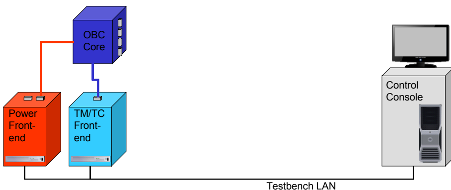
Figure 3.20: STB for HW / SW compatibility tests.
