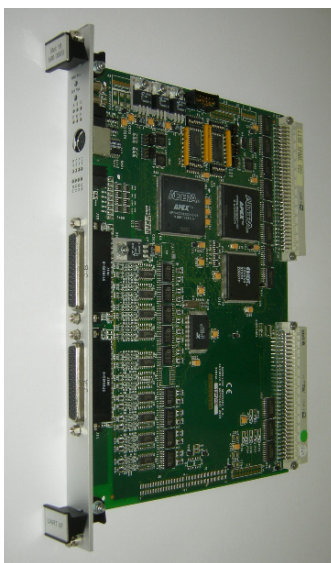
Figure 4.11: Example for a Simulator-Frontend interface card. Photo © Astrium
