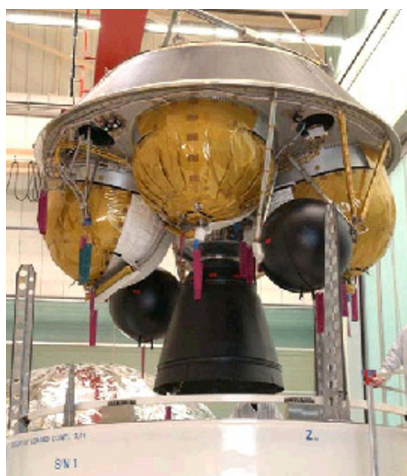
Figure 1.3: Ariane 5 upper stage L10. © ESA
