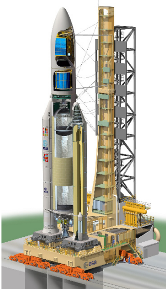
Figure 1.1: Cutaway of an Ariane 5 rocket. © ESA
