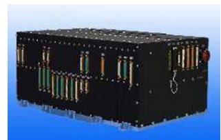
Figure 5.29: Power Control and Distribution Unit. © Astrium
