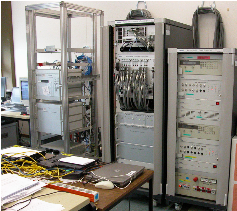
Figure 3.25: System testbed (Aeolus project). © Astrium
