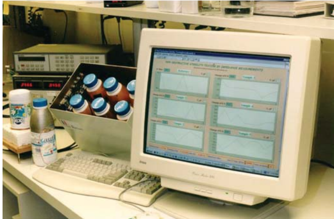
Figure 4.11 Testing system to perform microbiological experiments for non-invasive conductivity measurements of UHF milk in plastic bottles. Each bottle is equipped with a pair of external electrodes
