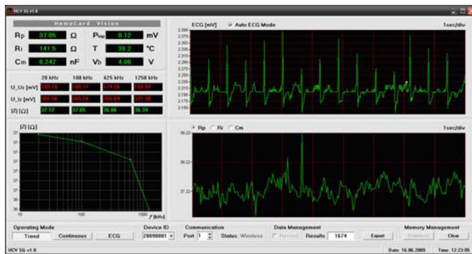
Figure 4.24 HemoCard Vision blood analysis-system: data plotted on the computer screen. Reproduced by permission of Martil Instruments B.V
