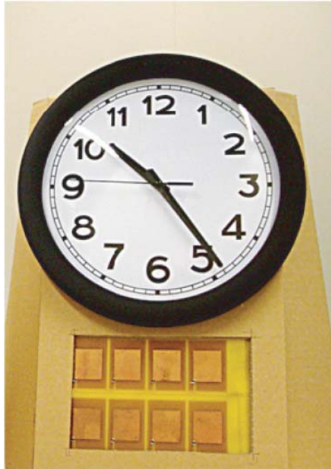
Figure 9.23 Wirelessly-powered wall clock employing eight rectenna elements with voltage doubler rectifying circuits [79, 80]. Reproduced by permission of Wiley
