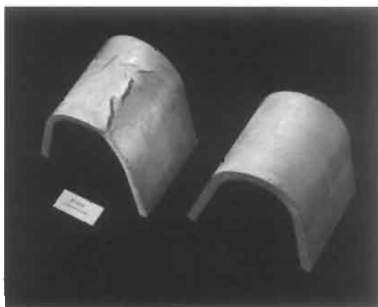
Figure 9.19 Plates 10 mm thick cast in 99.5Al subjected to three-point bend (a) filled at an ingate speed greater than 0.5 \text{ ms}^{-1} and (b) less than 0.5 \text{ ms}^{-1} (courtesy Runyoro 1995).
