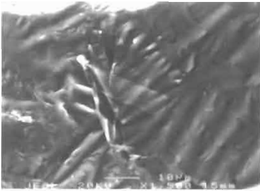
Figure 5.39 SEM image of an iron-rich particle nucleated on the underside of a thin alumina film imaged by (a) secondary electrons and (b) back-scattered electrons (Cao 2000).
