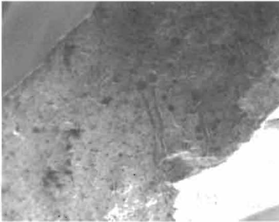
Figure 2.34 SEM image of a fracture surface of a zinc pressure die cast component revealing a bubble with an open trail (Divandari 2000).
