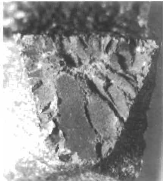
Figure 5.46 Plate fracture in the feeder neck of a ductile iron casting (Karsay 1980).
