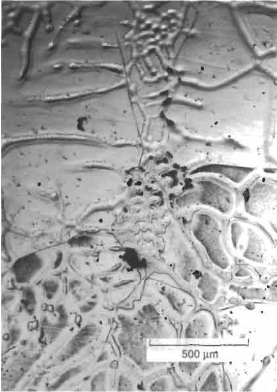
Figure 5.25 Micrograph of Al-0.2Cu alloy showing porosity and interdendritic segregation. Some grain boundary migration during cooling is clear. (Electropolished in perchloric and acetic acid solution and etched in ferric chloride. Dark areas are etch pitted.)
