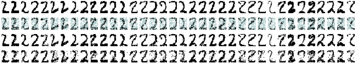
Figure 9.18: Learning digits (from Simon Lucas’ algoval system) using a Markov network. Top row: the 36 training examples. Each example is a binary image on 18 \times 14 pixels. Second row: the training data with 50% missing pixels (grey represents a missing pixel). Third row: Reconstructions from the missing data using a thin-junction-tree MN with maximum clique size 15. Bottom row: Reconstructions using a thin-junction-tree Boltzmann machine with maximum clique size 15, trained using efficient IPF.
