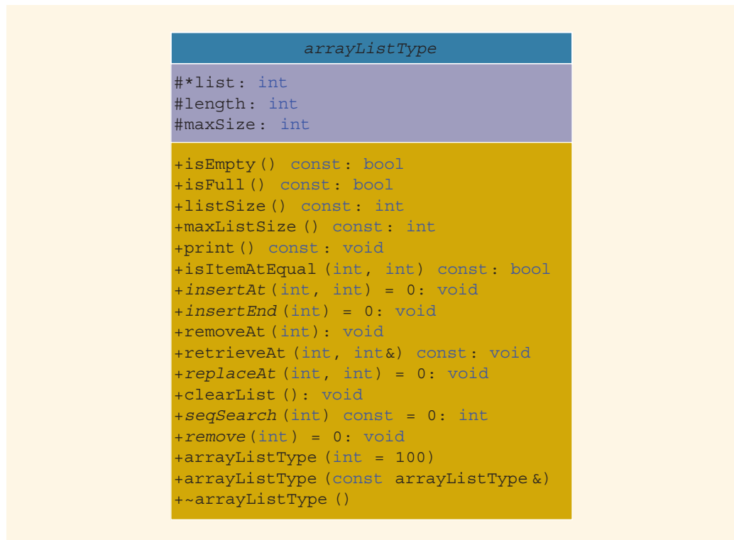
FIGURE 12-22 UML diagram of the class arrayListType
