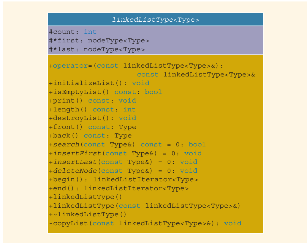
FIGURE 16-20 UML class diagram of the class linkedListType
