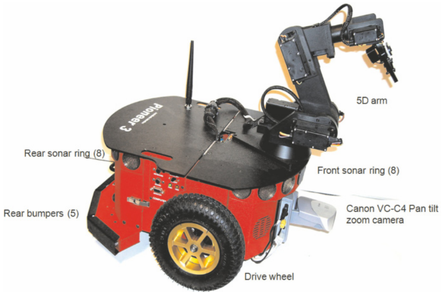
Fig. 1.4 Pioneer P3-DX sensors and actuators, alternative configuration
