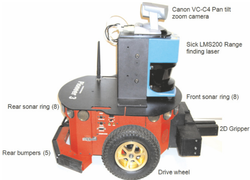
Fig. 1.3 Pioneer P3-DX sensors and actuators
