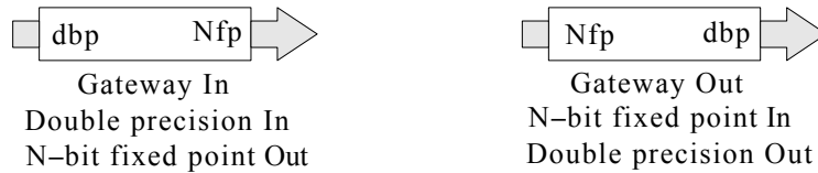
Figure 11.54. Symbols for conversion from double to N-bit fixed point and vice versa
