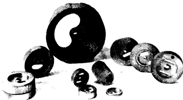
Figure 9-6-3 Space-harmonic coupled-cavity circuits. (After A. Staprans et al. [7]; reprinted by permission of IEEE, Inc.)
