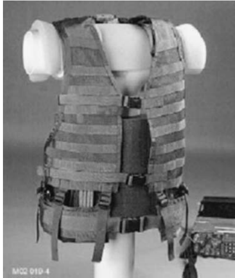
Figure 6.3 Body-worn squad level antenna vest used for military applications [20].
