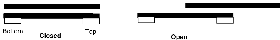
Figure 2.6 Typical antenna positions on slider phones.
