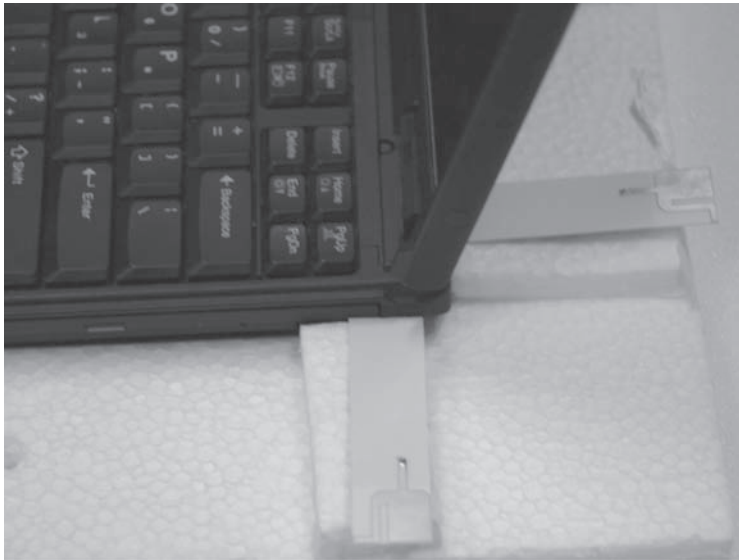
Figure 7.45 (a) Geometry of laptop (dimensions in millimetres) and antenna placement; (b) the antennas under test at p3.
