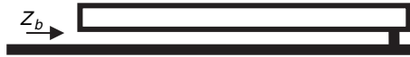
Figure 2.17 The battery creates a transmission line stub creating an impedance in series with currents flowing along the surface of the chassis.
