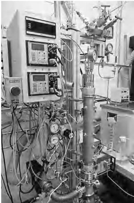
Fig. 14-8 Pilot plant with 0.2 L trickle-bed reactor (Hoffmann-La Roche, Kaiseraugst, Switzerland)
