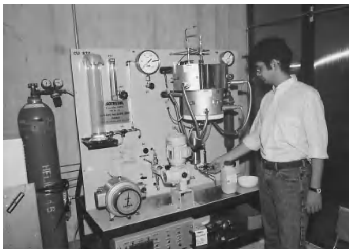
Fig. 8-6 Operation of a continuous high-pressure hydrogenation plant (CATATEST plant, VINCI technologies, France; high-pressure laboratory, FH Mannheim, Germany)
