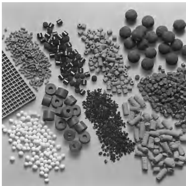
Fig. 6-1 Various shaped catalyst bodies (BASF, Ludwigshafen, Germany)
