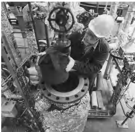
Fig. 8-7 A hydrogenation catalyst is introduced into a pilot plant in order to test it under process-relevant conditions (BASF, Ludwigshafen, Germany)
