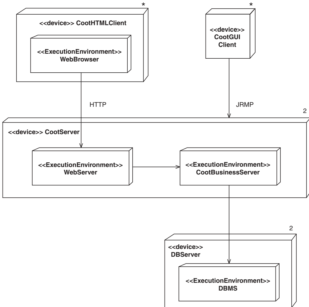
Figure 9.9: A more detailed deployment diagram for iCoot
