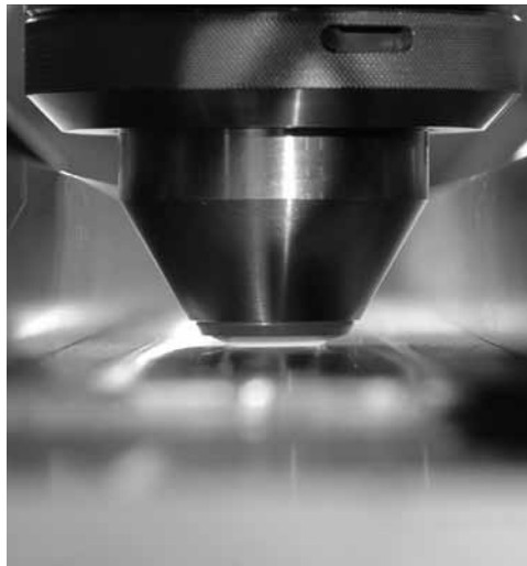
Figure 8.6 Friction stir solid state welding. (With thanks to TWI Limited [formerly The Welding Institute].)
