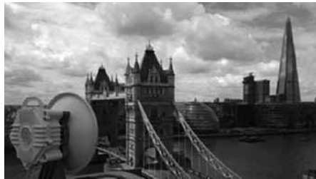
Figure 6.5 RF Com Dish with integral transceiver for point to point backhaul in a 4G or 5G network. (With thanks to RF.com.)
