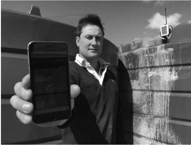
Figure 9.5 Satellite water tower monitor on a Merino sheep farm in Australian outback. (With thanks to Myriota.)
