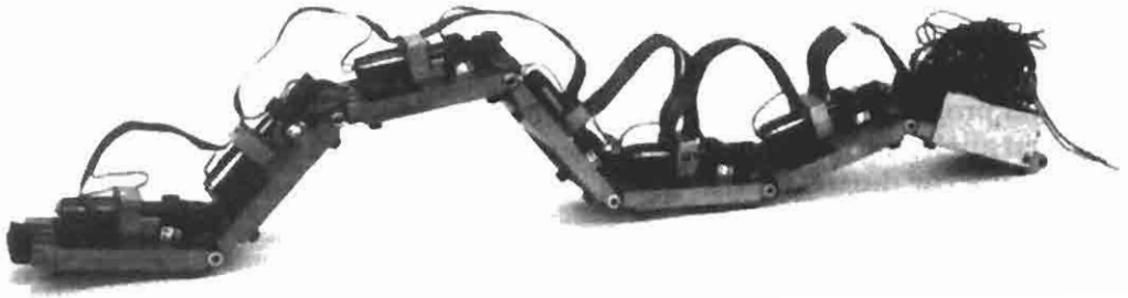
FIGURE 9.57c) General view of 7-link "caterpillar" device. This model was designed and built by a team of fourth-year students in the Mechanical Engineering Department of Ben-Gurion University under the author's supervision. It can move by using several bending modes, one of which appears in the photograph.
