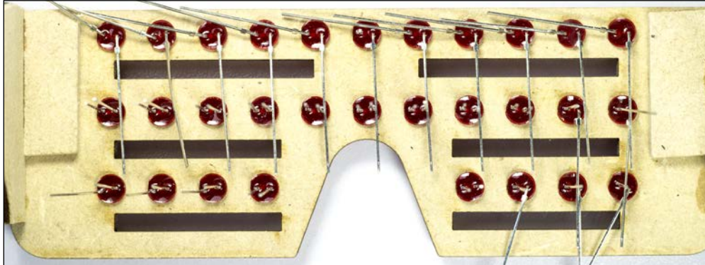
Figure 3.4: Showing all the LEDs lined up for soldering
