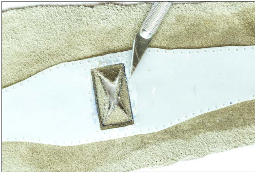
Figure 9.10 Cutting a hole for the OLED screen
