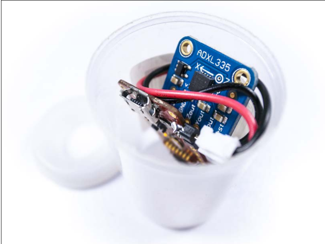
Figure 7.9: The components inside a film bottle
