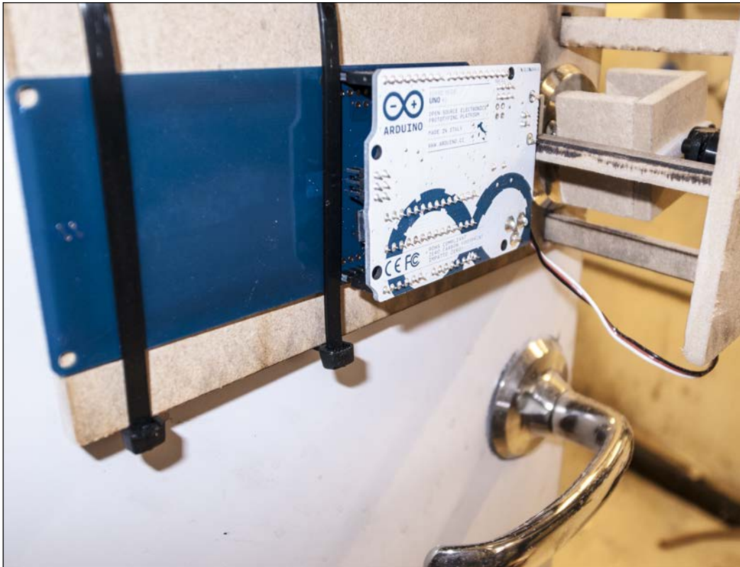
Figure 6.8: The final door lock in place
