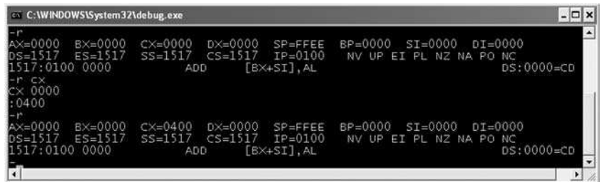
Figure 3.7 The Debug Register (r) command being first used to display the contents of the CPU registers and then to change the contents of the CX register from 0000 to 0400
