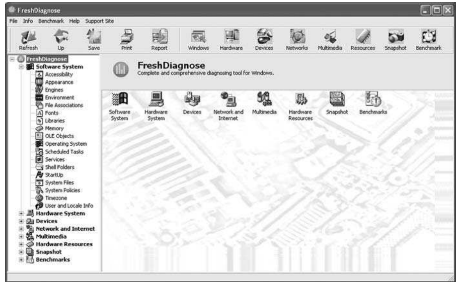
Figure 13.11 The Fresh Diagnose opening screen showing the eight main options that may be selected by pointing and clicking on the icons. Other options, such as Print and Report, may be selected directly from the tool bar. The window on the left provides a means of selecting individual modules
