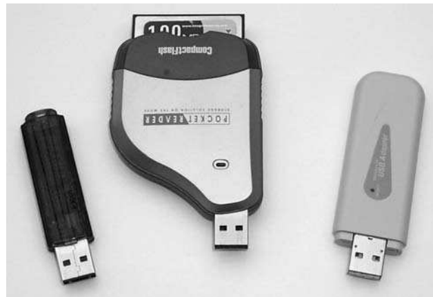
Photo 2.14 Some typical USB devices; a 256 MB memory stick, a Flash memory card reader, and a wireless network adapter
