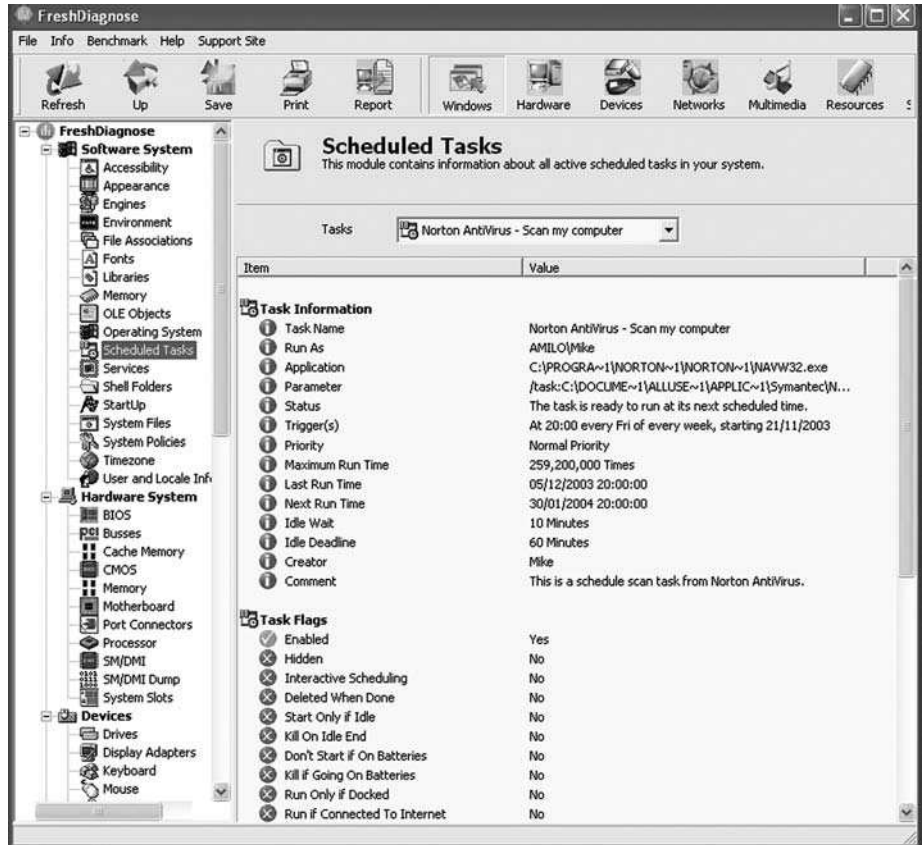
Figure 13.13 The Software System Scheduled Tasks report provides detailed information on each scheduled task. In this example, the Norton Antivirus task is being reported on. The task is scheduled to run every Friday at 20:00 and it will be next run on 30/01/2004
