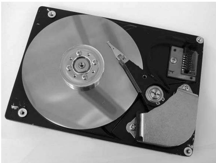
Photo 1.13 Interior of a hard disk drive
