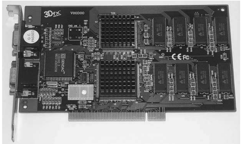
Photo 2.6 A PCI 3D graphics adapter card
