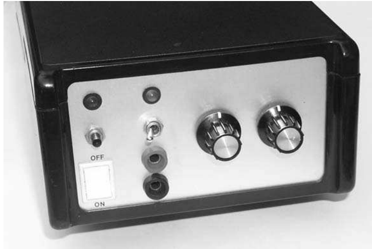
Photo 11.4 The prototype sound card oscilloscope interface
