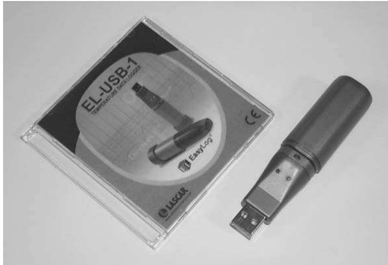
Photo 12.3 Lascar's EasyLog USB data logger
