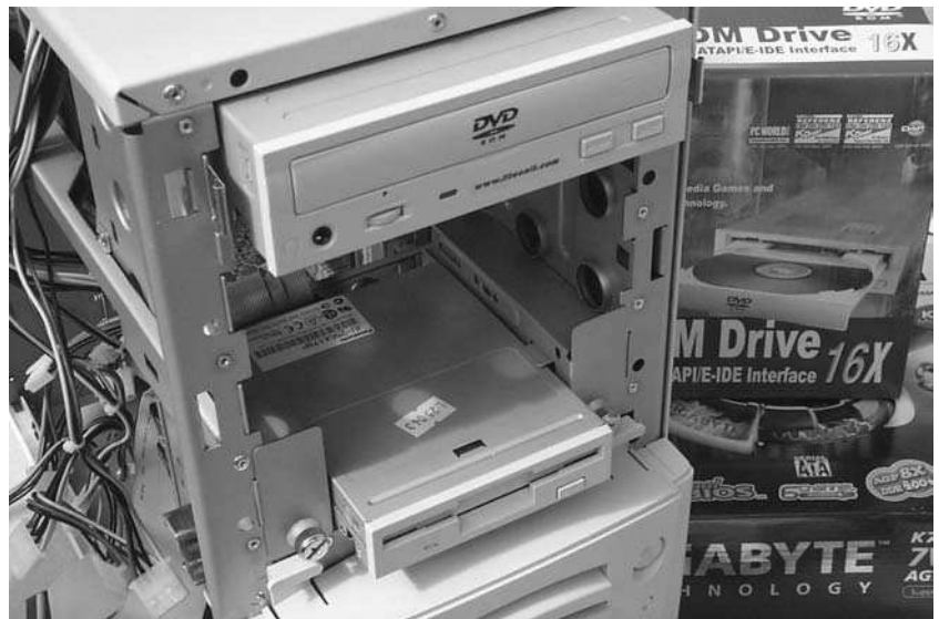
Photo 1.15 Drive bays in a tower PC (the hard drive has been removed)
