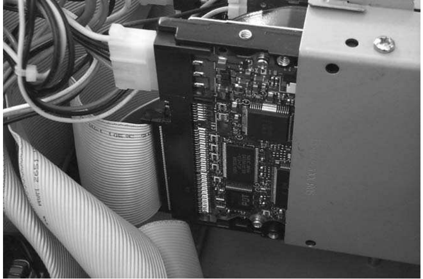
Photo 13.3 A drive power connector makes a convenient test point for measuring the +12 V and +5 V power rails
