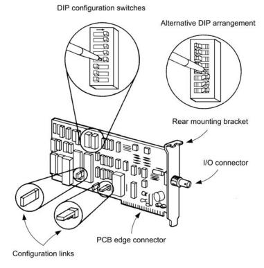
Figure 13.33 Typical bus adapter card showing links and settings
