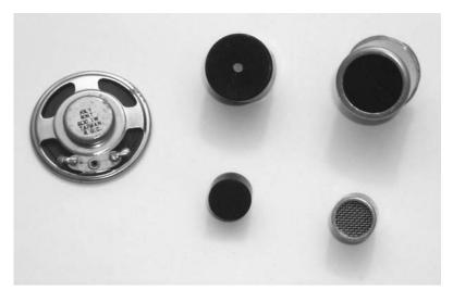
Photo 9.10 Various audible and ultrasonic transducers
