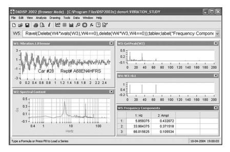
**Figure 10.16** A screen display produced by DADiSP. The screen shows various windows displaying information obtained during a vibration study
