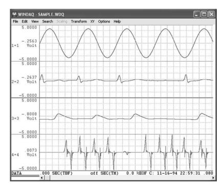
Figure 10.20 WINDAQ display showing time-related captured data
