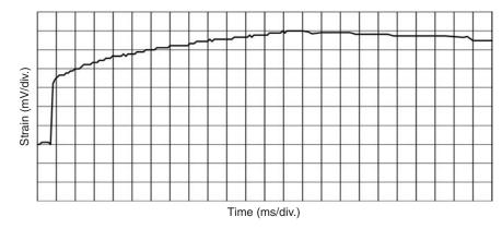
Press <SPACE> to abort, <X> to freeze, <+> or <-> to change timebase setting X = 33 ms/div. (time) and Y = 50 mV/div. (strain)
