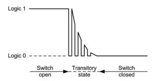
Figure 9.3 Typical waveform produced by a switch closure
