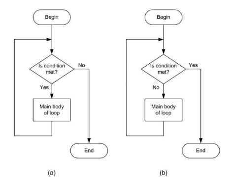
**Figure 6.2** Flowcharts illustrating the logic of DO WHILE ... LOOP and DO UNTIL ... LOOP structures. (a) DO WHILE ... LOOP; (b) DO UNTIL ... LOOP
