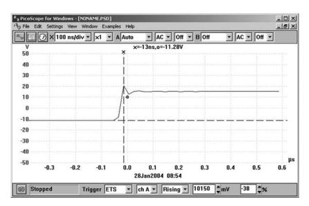
Figure 11.8 In this screen grab, the trigger point (shown with the grey circle) has been adjusted to just over 10V(10150 mV) and the time scale shifted in order to display the leading edge of a fast pulse
