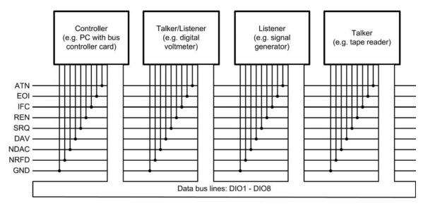
Figure 8.2 IEEE-488 bus showing signals and devices
