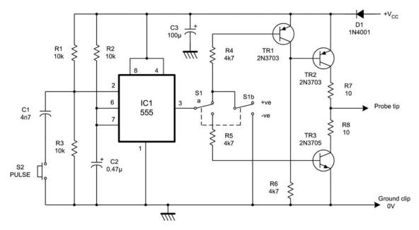
Figure 13.23 Logic pulser circuit
