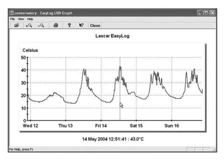
Figure 12.21 EasyLog's cursors can be moved to obtain precise data
