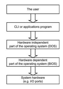
**Figure 3.1** *Relationship between the different layers of the operating system* (DOS and BIOS)
