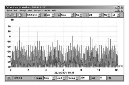
**Figure 11.13** Frequency spectrum of a 1 kHz square wave generated by a waveform generator. The instrument is set to capture 2048 samples per second. The increased frequency resolution of the instrument is now showing us how the noise spectrum is actually modulated onto the fundamental and harmonic components. This was simply not apparent in the spectra shown in Figures 11.11 and 11.12
