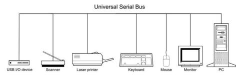
**Figure 2.8** USB arrangement for connecting a wide variety of peripheral devices
