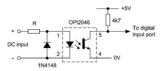
Figure 9.21 Optically isolated digital input for DC signals
