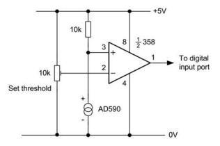
**Figure 9.29** *Temperature threshold detector based on an AD590 semiconductor temperature sensor*
