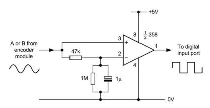
**Figure 9.17** Shaft encoder signal conditioning for measurement of rotational speed
