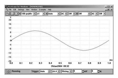
**Figure 11.6** *The DSO adjusted as for Figure 11.6 but with the timebase set to 100 \, \mu s/div.*
