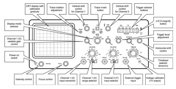
**Figure 13.25** *Layout of the controls and adjustments of a typical bench oscilloscope*
