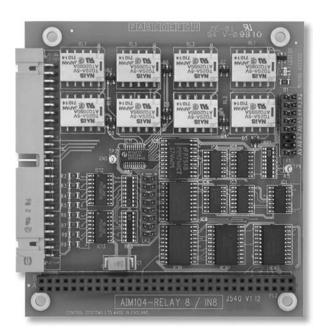
**Photo 2.12** *AIM104 I/O card for PC/104 expansion. This card has eight changeover relays (each rated at 30 V DC, 1A) and eight optically isolated inputs (photo courtesy of Arcom)*
