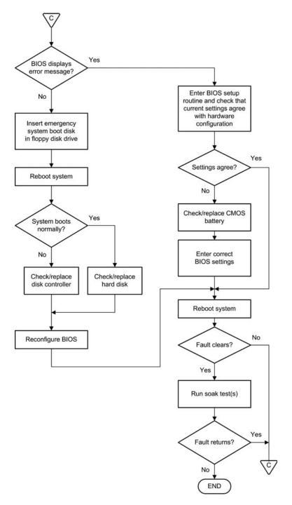
Figure 13.29 Fault location chart (BIOS, CMOS, and hard disk)
