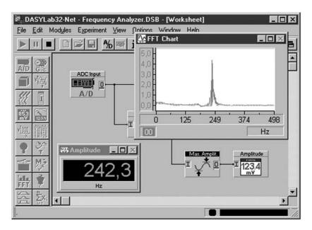
**Figure 10.11** A variety of different display options are available within DASYLab, including the ability to produce Fast Fourier Transformation (FFT)
