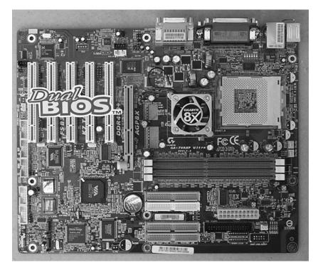
Photo 1.2 A modern high-specification dual-BIOS PC motherboard
