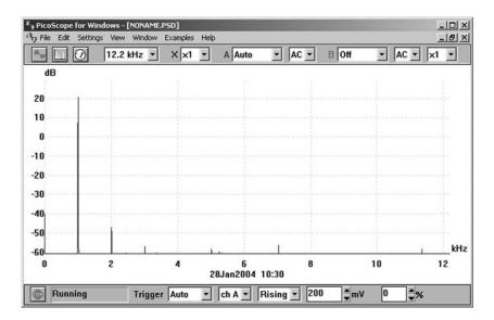
**Figure 11.15** Frequency spectrum of a 1 kHz sine wave generated by a low-distortion signal generator. The instrument is set to capture 4096 samples per second. Notice how the second harmonic is approximately 70 dB down on the fundamental. It is also possible to see the third, fifth, and the seventh harmonic
