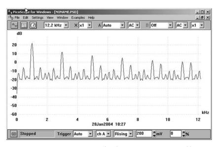
**Figure 11.10** *Frequency spectrum of a 1 kHz square wave generated by a general-purpose waveform generator. The instrument is set to capture 256 samples per second. Note that the noise floor appears to be only about 40 dB below the fundamental. Note also the preponderance of odd harmonics at 3, 5, 7 kHz, and so on*
