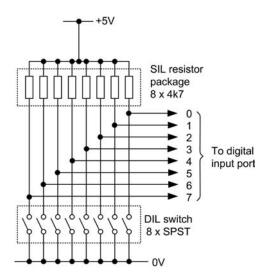
Figure 9.2 Interfacing a DIL switch input to a digital input port
