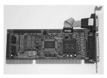
**Photo 2.4** *EISA dual serial/parallel port interface card (note the use of two mounting brackets for the external port connections)*
