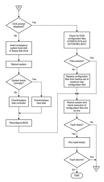
Figure 13.30 Fault location chart (configuration files and hard disk)
