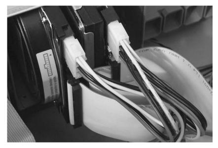
Photo 1.16 Power and data connectors at the rear of two hard drives
