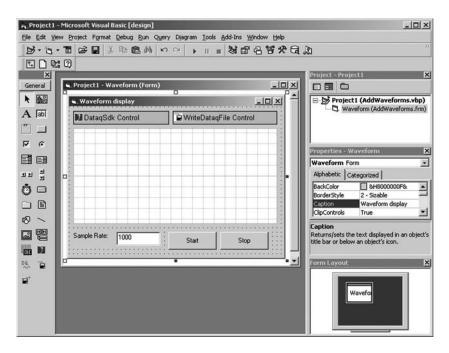
**Figure 10.2** Using Visual Basic to develop an application using an ActiveX control supplied by DATAQ. The control simplifies the task of plotting time-related waveforms of captured data
