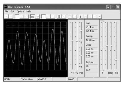
**Figure 11.20** A modulated waveform displayed using Windows Oscilloscope 2.51
