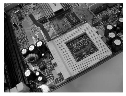
Photo 1.6 Socket 7 (with lever raised ready to accept a processor)
