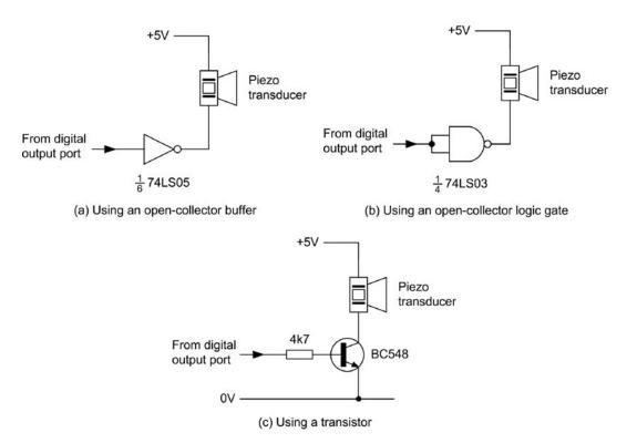
**Figure 9.35** *Audible output driver: (a) using a buffer; (b) using an open-collector logic gate; (c) using a transistor*
