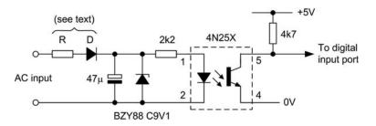
Figure 9.23 Optically isolated digital input for AC signals
