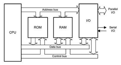
Figure 1.1 Elements of a microcomputer system
