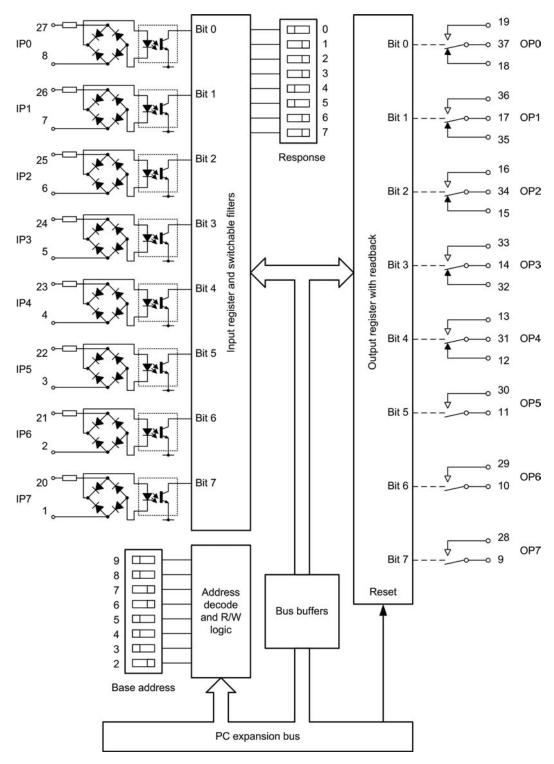
Figure 2.25 Simplified block schematic for the PDISO-8
