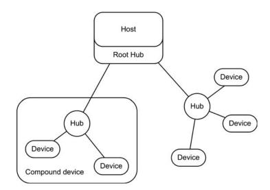
Figure 2.16 Host, Hub, and device interconnections
