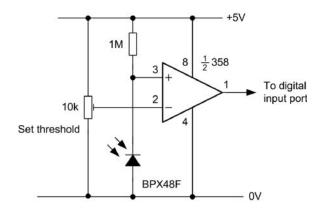
Figure 9.27 Light-level threshold detector based on a photodiode
