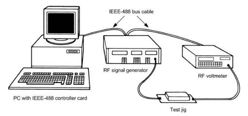
Figure 12.5 Crystal filter test hardware configuration
