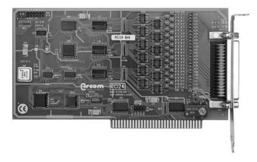
**Photo 2.5** A modern ISA card which provides 24 optically-isolated digital inputs (photo courtesy of Arcom)
