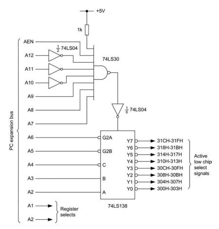
Figure 2.5 Representative address decoder arrangement
