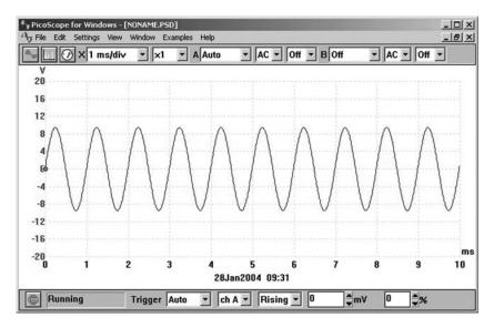
**Figure 11.5** A 10V peak–peak sine wave at 1 kHz displayed with the timebase set to 1 mV/div. and the vertical scale set to autoranging
