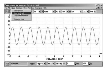
**Figure 11.3** *The Windows clipboard can be used to copy waveform and other data from PicoScope to other applications*
