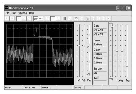
**Figure 11.23** *Expanded view of the vertical sync pulse of the waveform shown in Figure 11.22*
