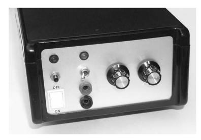
Photo 11.4 The prototype sound card oscilloscope interface
