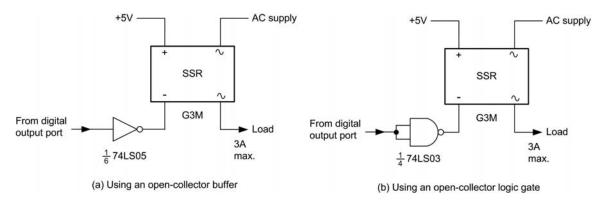
**Figure 9.40** Interface circuits for driving solid state relays: (a) driven from a buffered digital I/O port; (b) using an auxiliary buffer stage; (c) using an open-collector logic gate
