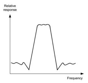
Figure 12.4 Typical crystal filter response characteristic
