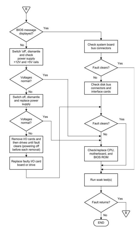
Figure 13.28 Fault location chart (motherboard, CPU, and I/O cards)
