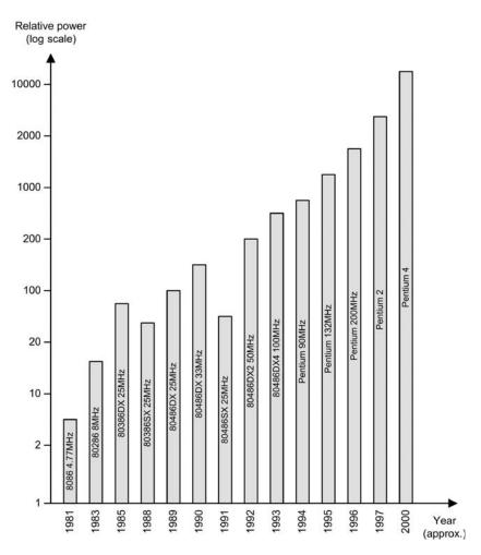
Figure 1.9 Relative power of Intel processors over the last two decades
