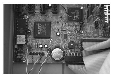
**Photo 13.2** *CMOS batteries may need replacing if CMOS errors are reported by the BIOS during system initialization*
