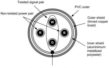
28 AWG tinned copper drain wire
