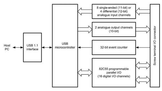
Figure 2.31 Block schematic diagram of the PMD-1208LS USB device
