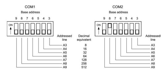
Note that a switch in the ON position corresponds to a zero and in the OFF position corresponds to the binary weight of the corresponding address bit (512, 256, 128, 64, 32, 14, 8). The base I/O address is the sum of all of the OFF switch address bits.
