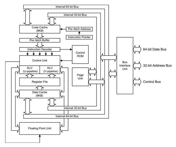
Figure 1.7 Internal architecture of the original Pentium processor
