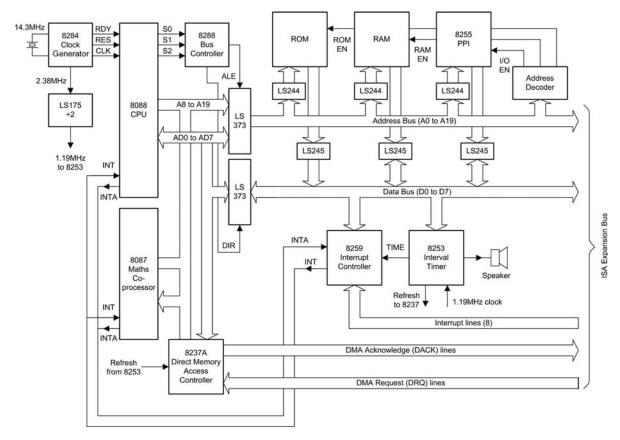
Figure 1.10 Internal architecture of the original IBM PC
