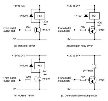
**Figure 9.33** *Typical medium- and high-current driver circuits: (a) transistor low-current relay driver; (b) Darlington medium/high-current relay driver; (c) MOSFET relay driver; (d) Darlington filament lamp driver*
