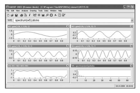
**Figure 10.17** *Example of using DADiSP to carry out a simple FFT-based analysis (shown in W6) of a synthesized square wave (shown in W5)*
