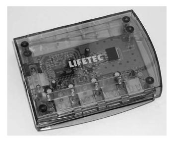
Photo 2.15 A low-cost USB four-port hub
