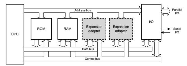
Figure 1.3 Microcomputer system with bus expansion capability
