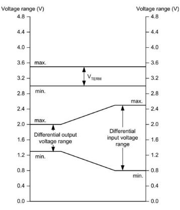
Figure 2.18 USB data signal levels
