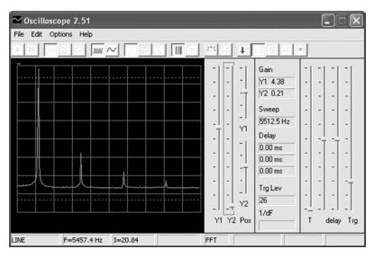
**Figure 11.28** *Frequency spectrum for a sine wave with severe distortion present (third, fifth, and seventh harmonic components can be clearly seen)*
