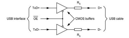
Figure 2.17 USB buffered interface
