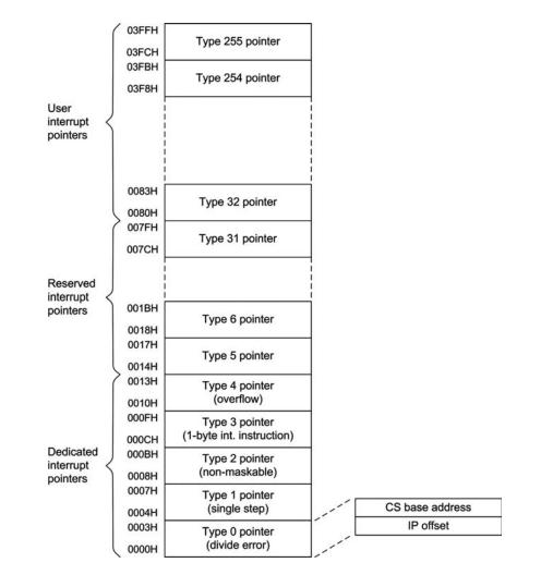
Figure 5.3 8086 Interrupt Pointer table
