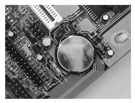
**Photo 1.11** *CMOS battery. The link adjacent to the battery can be used to clear the memory*
