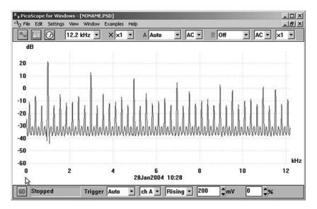
**Figure 11.11** Frequency spectrum of a 1 kHz square wave generated by a waveform generator. The instrument is set to capture 512 samples per second. Note that it is now possible to make a more accurate assessment of the various frequency components present. Note also that the noise floor can be more accurately measured
