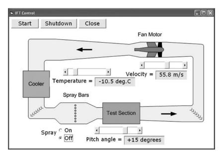
**Figure 12.22** *Ice flow tunnel (IFT) control application (the form was created using MS Visio and Visual Basic)*
