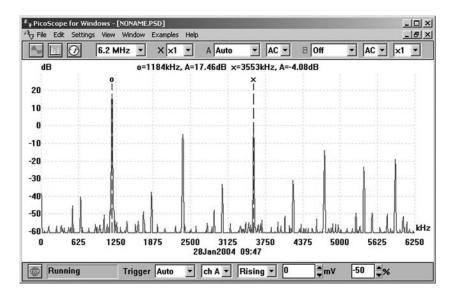
**Figure 11.16** Spectrum analysis of a radio signal at 1184 kHz (1.184 MHz). The cursors have been adjusted in order to display the amplitude and frequency of the fundamental and its third harmonic. The third harmonic at 3553 kHz (3.553 MHz) is approximately 21 dB down on the fundamental
