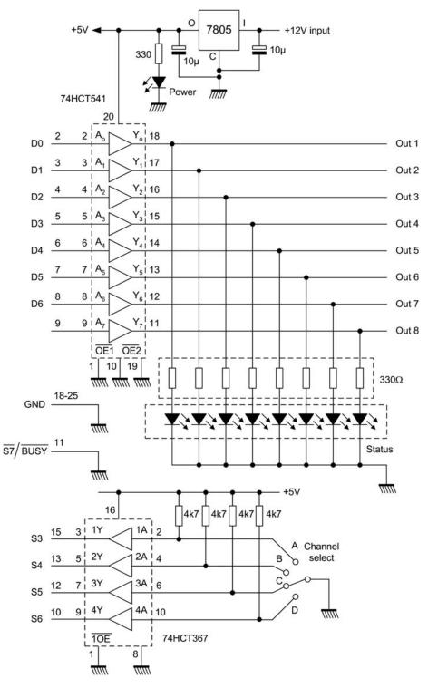
Figure 12.13 Parallel port I/O interface
