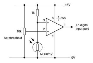
**Figure 9.26** *Light-level threshold detector based on a light-dependent resistor (LDR)*
