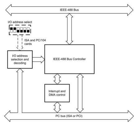
Figure 8.8 Simplified schematic diagram of an IEEE-488/GPIB controller
