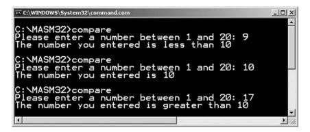
**Figure 5.6** *Results of running compare.exe from the CLI. The program has been tested with three different input values.*
