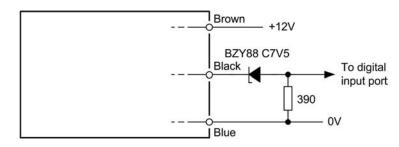
Figure 9.13 Interface circuit for a typical capacitive proximity sensor
