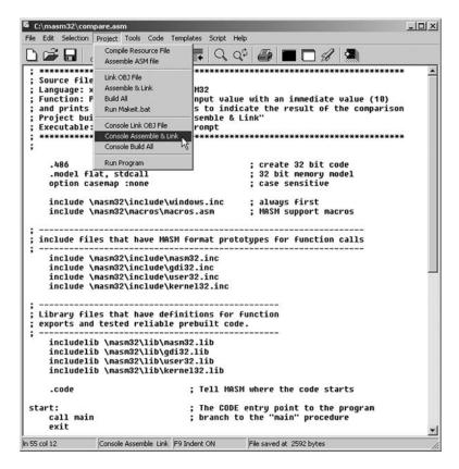
**Figure 5.4** The assembly language source code is entered using MASM32's integrated editor and Console Assemble and Link is used to automatically produce an executable program
