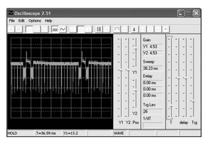
**Figure 11.21** Video cross-hatch waveform (vertical scan) displayed using Windows Oscilloscope 2.51
