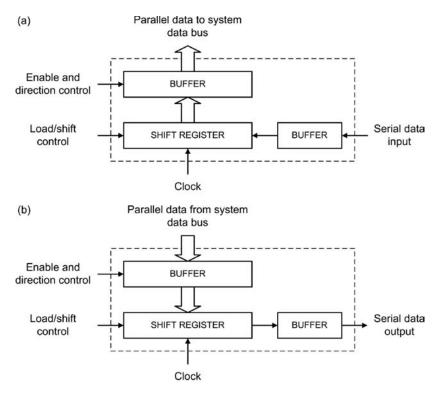
Figure 1.4 Data conversion: (a) serial-to-parallel and (b) parallel-to-serial
