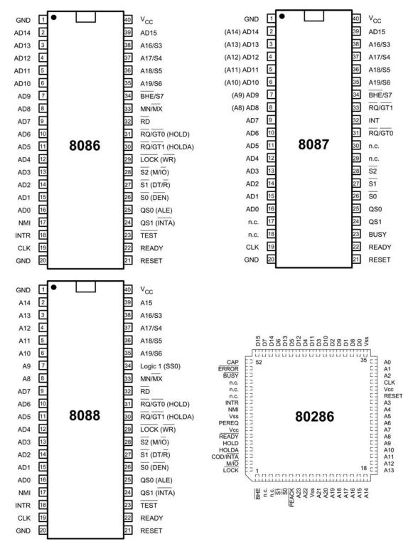
Figure 1.12 Pin connections for legacy processors
