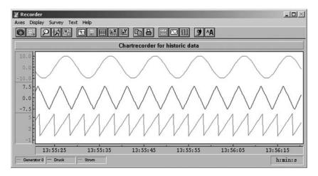
Figure 10.12 The DASYLab chart recorder display
