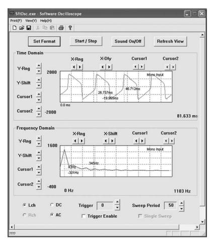
**Figure 11.24** Use of cursors for precise parameter measurement of a repetitive waveform using Software Oscilloscope
