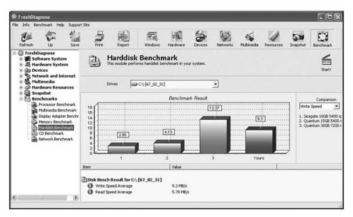
**Figure 13.16** A typical Hard Disk Benchmark display. The system on test produces a write speed of 9.3 MB/s. This is around 40% slower than that of a 30 GB Quantum drive which rotates at 7200 rpm
