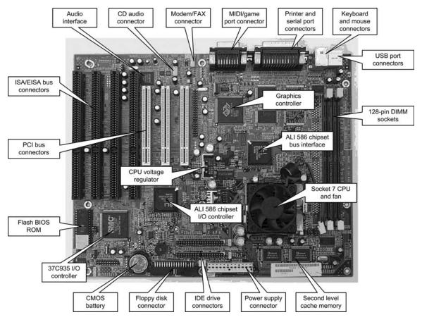
**Figure 1.17** *Motherboard layout for a modern PC supporting multiple bus standards*
