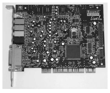
Photo 11.3 A typical low-cost sound card supplied in PCI format
