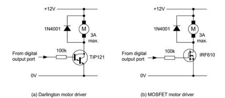
**Figure 9.38** *Motor driver circuits: (a) Darlington motor driver; (b) MOSFET motor driver*
