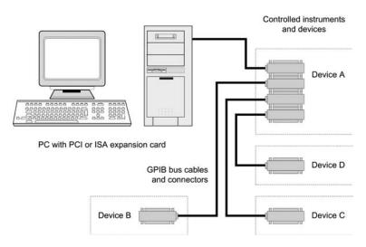
Figure 8.7 Typical IEEE-488 bus configuration (star configuration)
