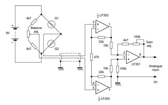
Figure 12.10 Strain gauge input signal conditioning circuitry
