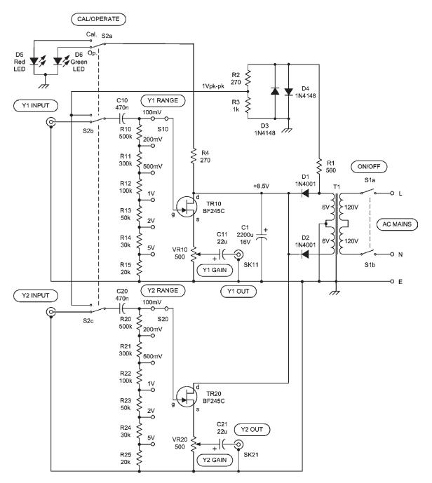
Figure 11.17 Complete circuit of the sound card interface
