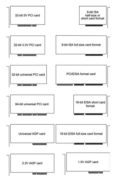
**Figure 2.2** *Outlines for various types of PC expansion card (component side view)*
