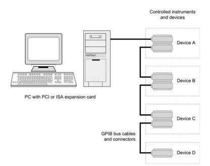
Figure 8.6 Typical IEEE-488 bus configuration (daisy chain configuration)
