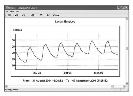
Figure 12.20 EasyLog display of captured data
