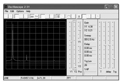
**Figure 11.27** *Frequency spectrum for a sine wave with mild distortion present (third and seventh harmonic components are visible)*
