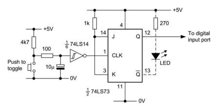
Figure 9.8 Latching action switch
