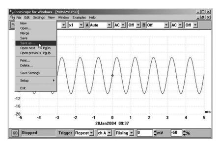
**Figure 11.2** The PicoScope software uses a conventional drop-down menu system. Here the 'Save as' option has been selected from the 'File' menu in order to preserve the waveform data for later viewing or analysis using external software
