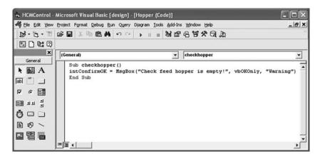
**Figure 4.1** It is possible to obtain the same results using different programming languages. This Visual Basic code produces the simple warning message shown in Figure 4.2
