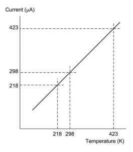
Figure 9.24 Characteristic of the AD590 semiconductor temperature sensor
