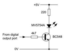
Figure 9.32 Using an auxiliary transistor to drive an LED
