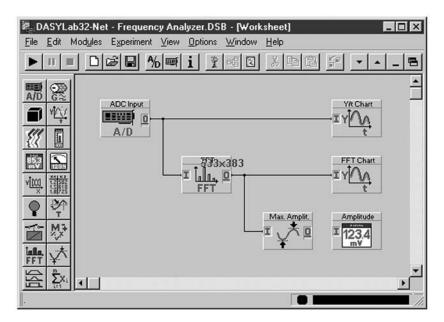
**Figure 10.10** *DASYLab programming involves simple 'drag and drop'* techniques
