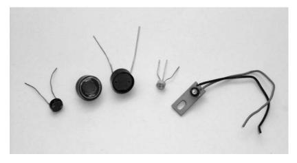
Photo 9.4 Various optical and light-level sensors
