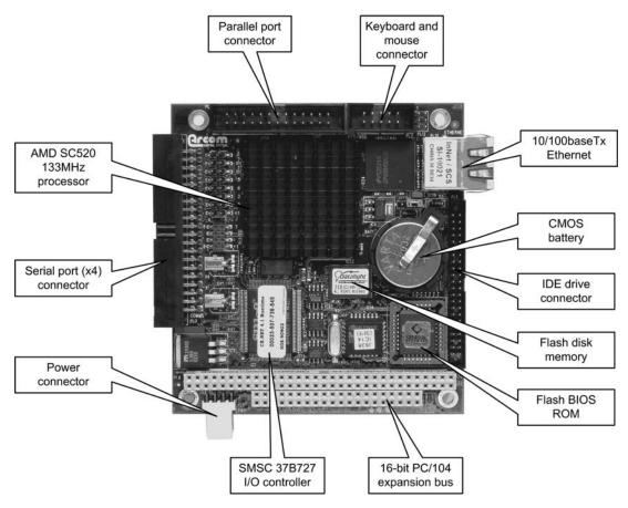
Figure 1.18 Layout of an embedded PC controller
