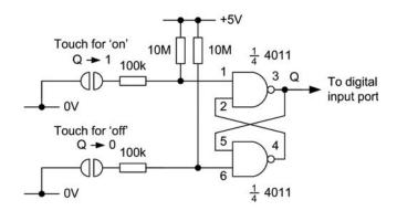
Figure 9.7 Touch-operated switch
