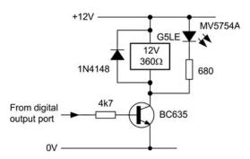
Figure 9.34 An LED indicator can be easily added to a relay driver
