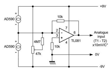
Figure 12.23 Arrangement of AD590 temperature sensors for differential measurements
