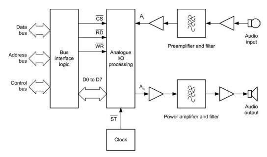
Figure 12.6 Simplified block schematic of the prototype speech enunciator
