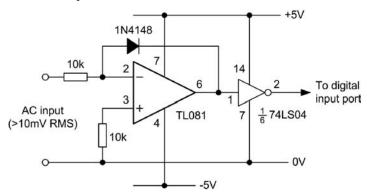
Figure 9.30 Interface circuit to permit AC sensing
