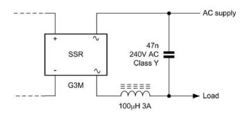
Figure 9.41 Using a 'snubber' network with an inductive load
