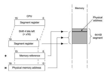
Figure 1.6 Process of forming a 20-bit physical address
