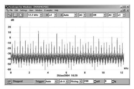
**Figure 11.12** Frequency spectrum of a 1 kHz square wave generated by a waveform generator. The instrument is set to capture 1024 samples per second. Note how the frequency resolution of the instrument has increased considerably compared with the previous frequency spectra
