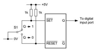
Figure 9.5 Debounce circuit based on an RS bistable
