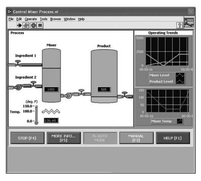
**Figure 10.7** LabVIEW is equally at home in control applications as it is in the field of data acquisition and instrumentation. This screen shows a typical VI used in a process control application
