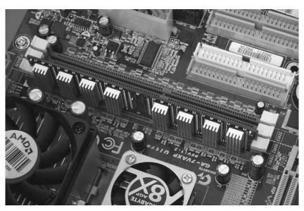
**Photo 1.10** *DIMM memory module with heatsinks fitted to each memory device*
