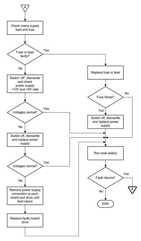
Figure 13.27 Fault location chart (power supply)
