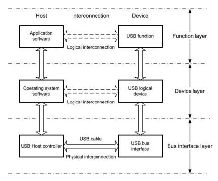
**Figure 2.15** *Layers in USB architecture (note the apparent peer–peer logical interconnection)*
