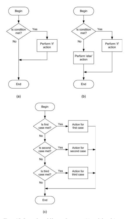
**Figure 4.7** Commonly available control structures: (a) simple branch (If ... EndIf); (b) binary branch (If ... Else ... EndIf); (c) multiple branch (Select ... Case ... EndSelect)
