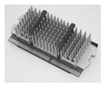
Photo 1.7 A modern Slot 1 Pentium processor
