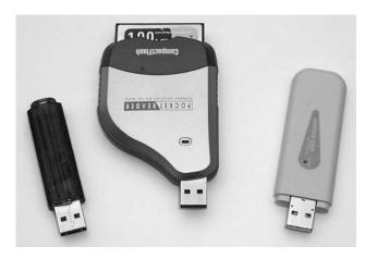
**Photo 2.14** Some typical USB devices; a 256 MB memory stick, a Flash memory card reader, and a wireless network adapter
