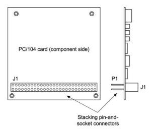
Figure 2.6 Basic arrangement of the PC/104 bus
