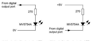
(a) Logic 1 to illuminate the LED (b) Logic 0 to illuminate the LED
