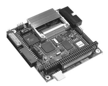
**Photo 2.11** Viper ultra-low power PC/104 format single board computer based on Intel's 400 MHz PXA255 XScale RISC processor. The board features a flat panel graphics controller, audio controller, 10/100baseT Ethernet, five serial ports, dual USB, digital I/O, onboard Flash memory and Compact Flash expansion (photo courtesy of Arcom)
