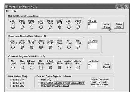
**Figure 10.23** VB Port Test utility developed by Chris Schroeder. This handy program is invaluable for checking the status of the PC's parallel ports
