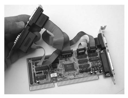
**Photo 1.4** *A typical ISA expansion card which provides two serial and two parallel ports*
