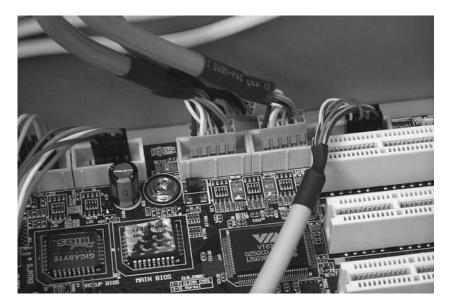
**Photo 13.4** Connectors can often be problematic and are a frequent cause of intermittent hardware faults. In this case, the rightmost serial ATA (SATA) connector is not correctly seated. Simply pushing the connector fully home was sufficient to clear the fault!
