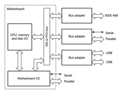
Figure 2.1 A typical PC expansion scheme
