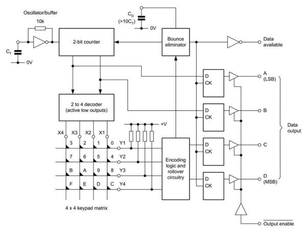
Figure 9.10 Simplified internal arrangement of the 74C922 keyboard encoder
