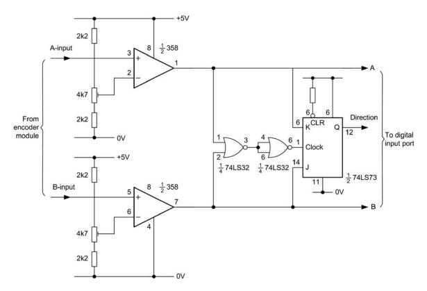
Figure 9.19 Additional logic required to provide direction sensing
