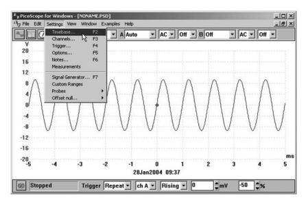
**Figure 11.4** The DSO control settings can be changed by using the drop-down menus as well as the tool buttons and controls provided in the display window
