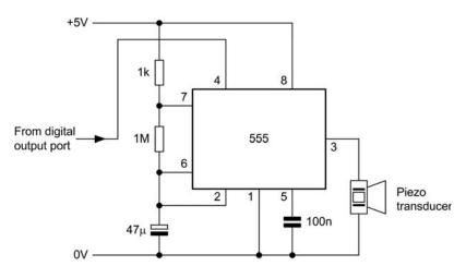
Figure 9.36 Pulsed audible alarm based on a 555 astable
