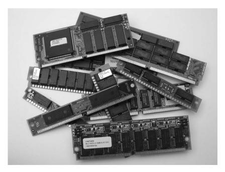
**Photo 1.9** Various PC memory devices with capacities varying from 1 to 256 MB
