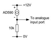
**Figure 9.25** *Typical input interface for the AD590 semiconductor temperature sensor*
