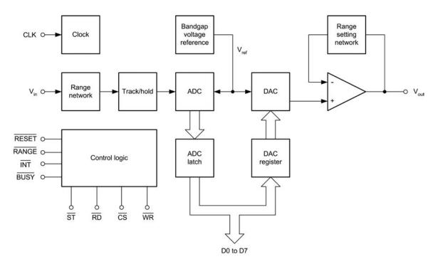
**Figure 12.7** Internal arrangement of the Analogue Devices AD7569 8-bit analogue I/O system
