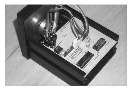
Photo 12.2 Prototype parallel port interface module
