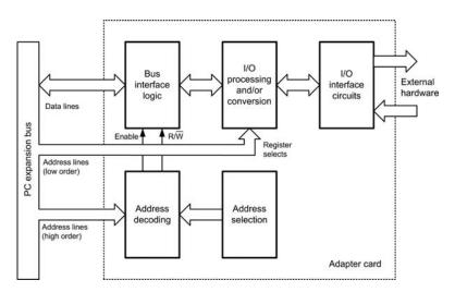
Figure 2.4 Generalized block schematic for an ISA/EISA expansion card
