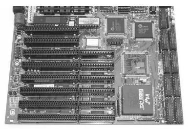
**Photo 2.7** Motherboard with ISA/EISA bus connectors (note that two out of the eight slots only provide access to the 8-bit bus)
