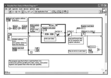
**Figure 10.4** *A block diagram of the LabVIEW VI designed to monitor the PC's parallel ports*
