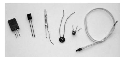
Photo 9.5 Various temperature and gas sensors
