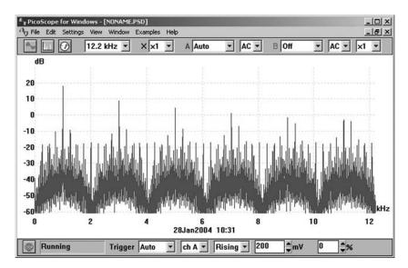
**Figure 11.14** Frequency spectrum of a 1 kHz square wave generated by a waveform generator. The instrument is set to capture 4096 samples per second. It is now easy to see how the modulated spectrum varies
