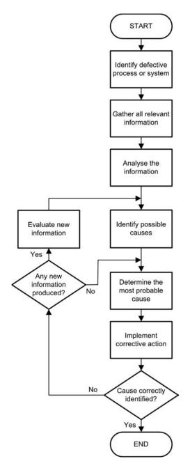
**Figure 13.18** Flow chart to show the generalized approach to troubleshooting (a series of more detailed charts appears later in this chapter)
