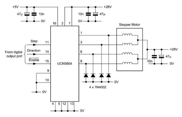
Figure 9.42 Stepper motor interface based on the UCN5804
