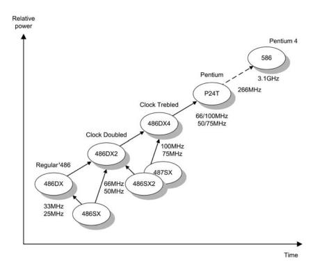
Figure 1.8 Development of the 'x86 Intel processor family
