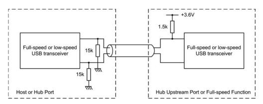
Figure 2.19 Pull-up and pull-down resistors in a USB interface
