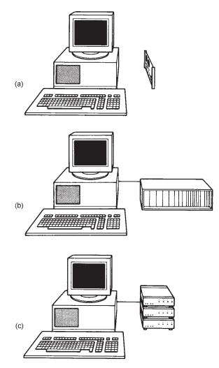
**Figure 12.1** Three basic approaches to PC-based instruments: (a) internally fitted PC expansion cards; (b) PC expansion cards in an external card frame; and (c) separately enclosed PC instruments linked via a parallel port, RS-232 serial port, USB, or via the IEEE-488 bus
