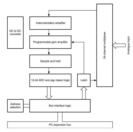
Figure 2.27 Simplified block schematic of the AIP-24
