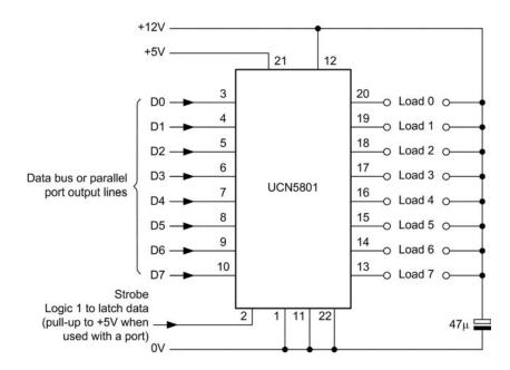
Figure 9.39 Typical output driver arrangement based on the UCN5801
