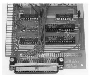
**Photo 2.10** *Typical prototype card bus interface logic*
