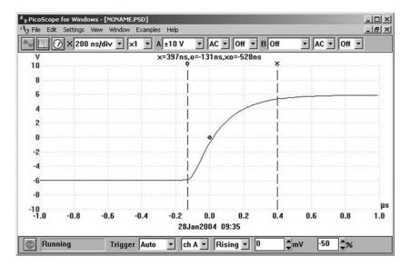
**Figure 11.9** The addition of a second time cursor makes it possible to measure the time accurately between two events. Here event 'o' occurs 131 ns before the trigger point whilst event 'x' occurs 397 ns after the trigger point. The elapsed time between these two events is 528 ns. The two cursors can be adjusted by means of the mouse (or other pointing device) or, more accurately, using the PC's cursor keys
