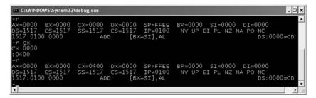
**Figure 3.7** The Debug Register (x) command being first used to display the contents of the CPU registers and then to change the contents of the CX register from 0000 to 0400
