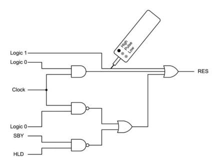
**Figure 13.22** Using a logic probe to test a typical combinational logic arrangement. The probe is moved from node to node and the displayed logic levels are compared with those that would be expected
