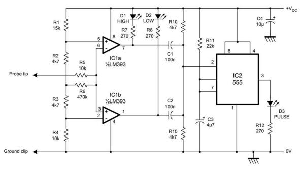
Figure 13.20 Logic probe circuit
