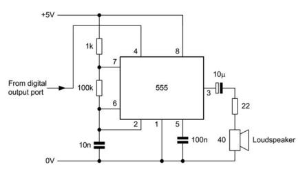
Figure 9.37 Audible alarm with output to a moving coil loudspeaker
