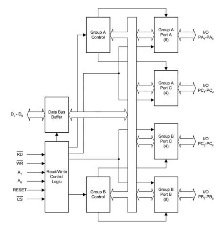
Figure 1.14 Internal architecture of the 8255A
