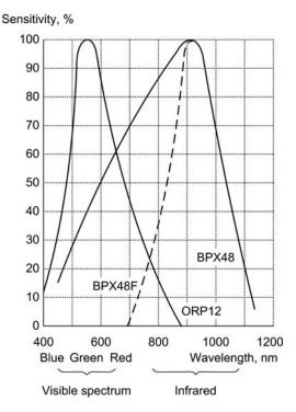
Figure 9.28 Comparsion of typical spectral response of LDR and photodiodes
