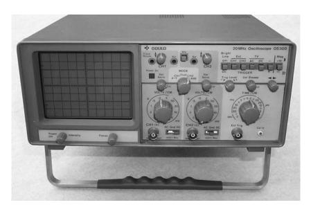
**Photo 11.2** *Controls fitted to a conventional oscilloscope (compare this with the virtual interface shown in Figure 11.1)*
