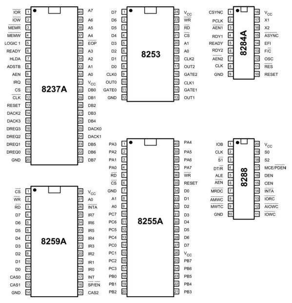
Figure 1.13 Pin connections for legacy support chips
