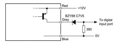
Figure 9.14 Interface circuit for an optical proximity sensor
