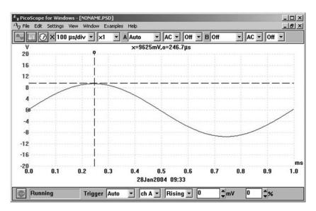
**Figure 11.7** Adjustable cursors make it possible to carry out extremely accurate measurements. Here the peak value of the (nominal 10 V peak) waveform is measured at precisely 9625 mV (9.625 V). The time to reach the peak value (from 0 V) is measured as  $246.7 \mu s$  (0.2467 ms)
