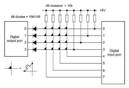
Figure 9.9 Typical 4 × 4 matrix keypad interface
