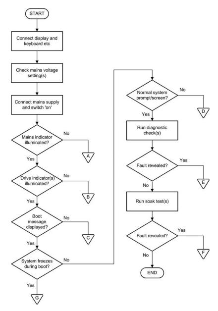
Figure 13.26 Fault location chart (initial stages)
