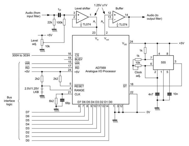
Figure 12.8 Simplified circuit of the enunciator card
