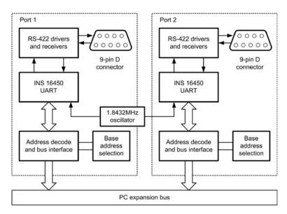
Figure 2.28 Simplified block schematic of the Dual-422
