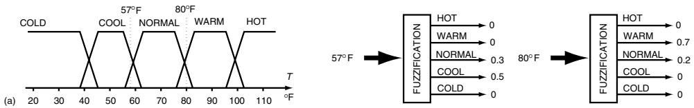
FIGURE 32.20 Fuzzification process: (a) typical membership functions for the fuzzification and the defuzzification processes, (b) example of converting a temperature into fuzzy variables.
