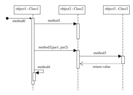
We have three objects in this scenario. Time runs from top to bottom, and the vertical dashed lines (lifelines) indicate the objects' continued existence through time.
