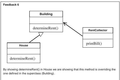
Interestingly Java will use the most correct determineRent() method depending upon which type of object the method is invoked on. Thus RentCollector will invoke the method defined in House if printing a bill for a house but will use the method defined in Building for any other type of building. This is automatic – the code in the RentCollector class does not distinguish between different types of Building.
