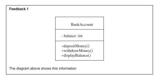
UML allows us to suppress any information we do not wish to highlight in our diagrams – this allows us to suppress irrelevant detail and bring to the readers attention just the information we wish to focus on. Therefore the following are all valid class diagrams...
