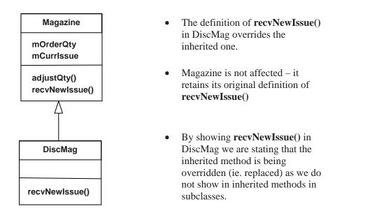
When we call the **recvNewIssue**() method on a DiscMag object Java automatically selects the new overriding version – the caller doesn't need to specify this, or even know that it is an overriden method at all. When we call the **recvNewIssue**() method on a Magazine it is the method in the superclass that is invoked.
