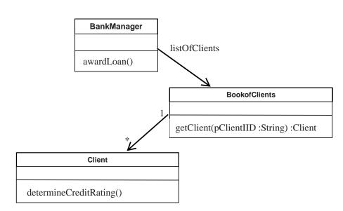
The system shown above is driven by the BankManager class. The awardLoan() method is invoked, either via the interface or from another method. This method is intended to accept or reject a loan application.
