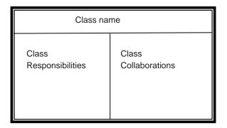
Responsibilities are the things the class needs to know about (ie the attributes) and the things it should do (ie. the methods) though on a CRC card these are not as precisely defined as on a UML diagram. The collaborations are other classes that this class must work with in order to fulfil its responsibilities.
