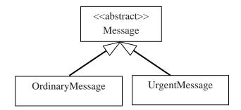
However in this case there are no unique features of an ordinary message – messages have an associated cost, the cost and text can be obtained and new messages can be created. All this is true for urgent messages. An urgent message is just the same as an ordinary message where the text and the cost has been changed slightly. Thus UrgentMessage is a type of Message and can inherit ALL of the features of Message with the cost and text methods being overridden.
