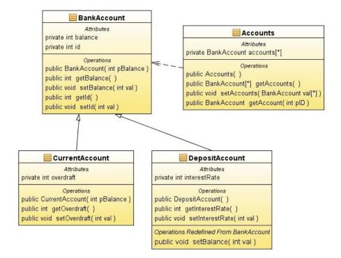
Thus given the diagram above NetBeans would create four classes, three of which would automatically be placed in an inheritance hierarchy. Method stubs would be created for each of the specified methods and while the code inside each method would still need to be written the constructor for CurrentAccount would automatically invoke the constructor for Bank Account passing the parameter pBalance upwards.
