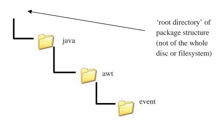
A large Java development should be split into suitable packages at the design stage UML provides a 'Package Diagram' to represent the relationships between classes and packages.
