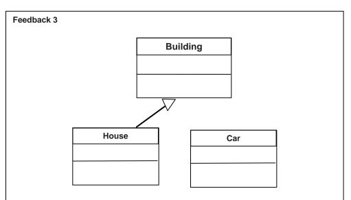
A house is a type of building and can therefore inherit the attributes of building however this is not true of a car. We cannot place two classes in an inheritance hierarchy unless we can use the term **is a**.
