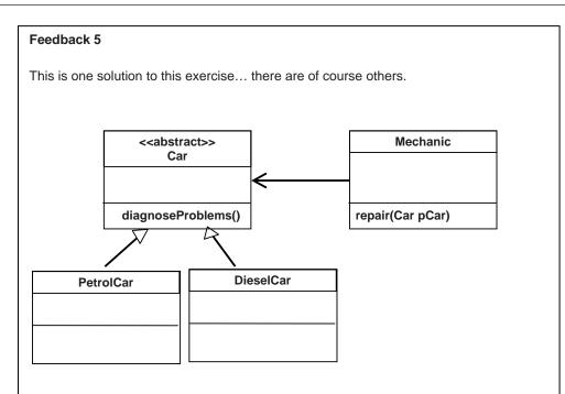
Here Mechanic is directly interacting with Car. In doing so it can interact with any subtype of Car e.g. Petrol, Diesel or any other type of Car developed in the future e.g. (Electric). These are all different (different shapes) and yet Mechanic can still interact with them as they are all Cars. This is polymorphic.
