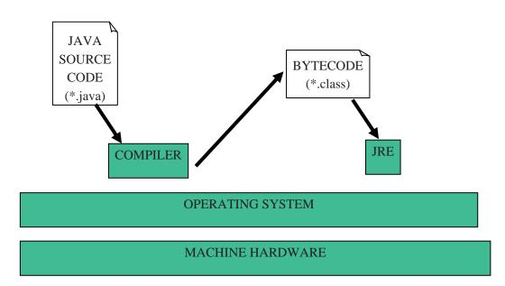
A version of the Java Runtime Environment (JRE), which incorporates a Java Virtual machine (VM), is required to execute the bytecode and the Java library packages. Thus a JRE must be present on any machine which is to run Java programs.
