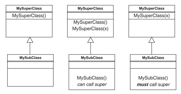
On the left above:- it is legal, though bad practice, to have a subclass with no constructor because superclass has a parameterless constructor.
