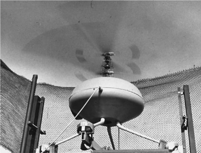
Figure 19.3 Rotary-wing aircraft functioning rig
