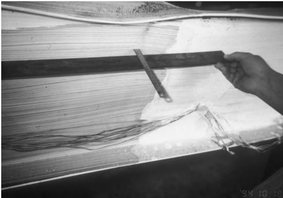
Fig. 19.28 Local buckling of web. (Courtesy of Structures/Materials Laboratory, Virginia Tech.)
