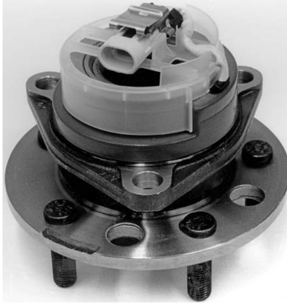
FIGURE 2.74 Magnetically distributed sensor integrated with wheel bearing.
