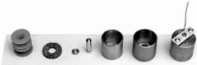
FIGURE 4.18 Unipolar latching relay with stationary MQ2 magnet components and assembly with contacts. (Courtesy of Delphi Corp.)
