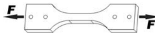
Figure 8 Schematic diagram of direct tensile test involving the dog bone geometry of the specimen.
