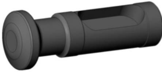
Figure 21 Calibrated punch pocket design.
