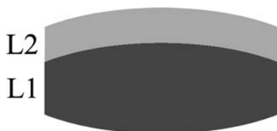
Figure 15 Cross-sectional view indicating difference in layer shape for (L1) first layer and (L2) second layer of a bilayer tablet produced using concave tooling.
