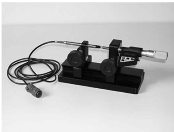
Figure 5 Example of a drum-type micrometer and LVDT calibration setup. Abbreviation: LVDT, linear variable differential transducer.
