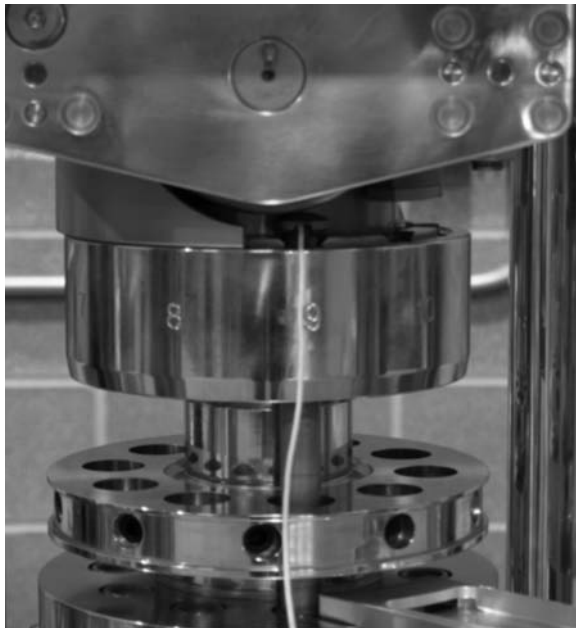
Figure 18 Calibrated punch in tablet press.
