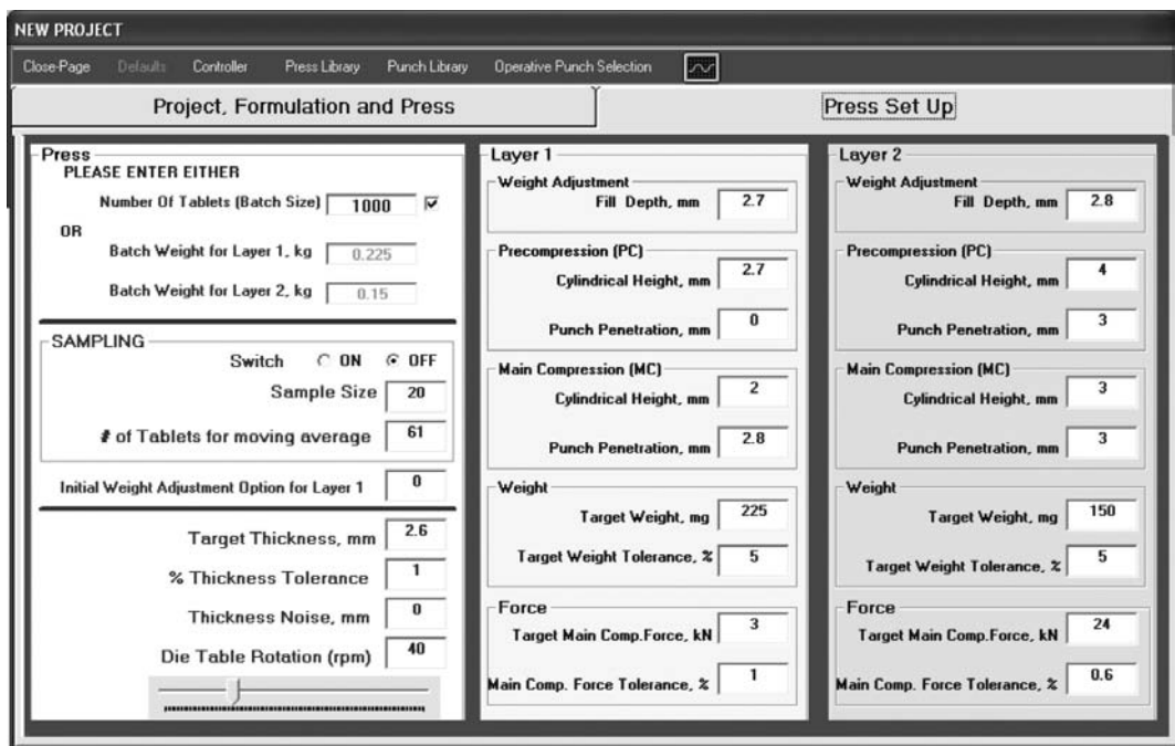
Figure 7 (B) BILAYERex user interface module: force-specific volume correlation parameters. (C) BILAYERex user interface module: press set up parameters.
