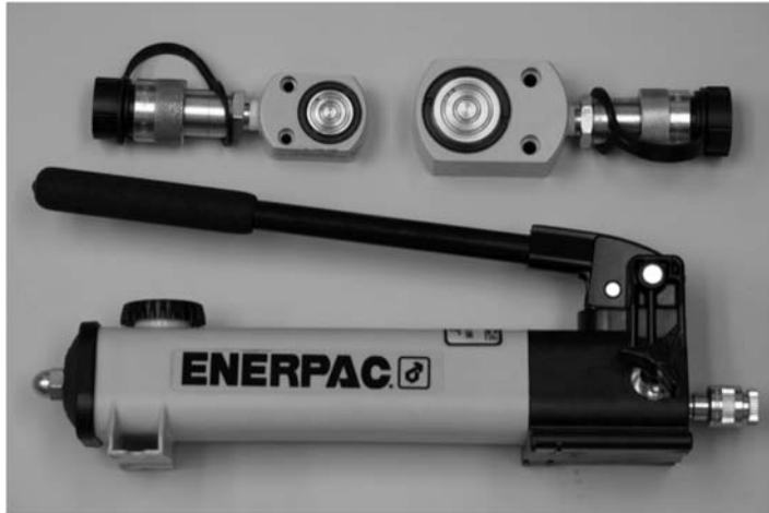
Figure 17 Calibration kit hydraulic pump.
