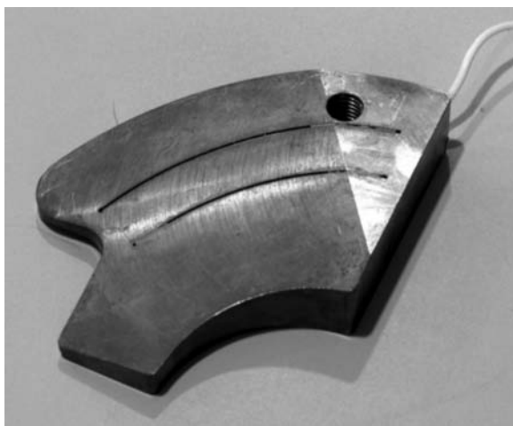
Figure 14 Instrumented ejection ramp.
