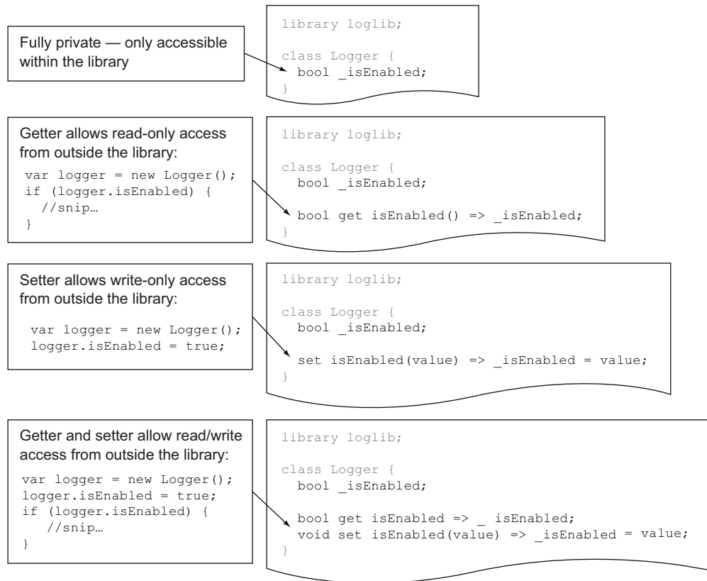
Figure 5.13 Using getters and setters to provide varying levels of field access to external users of a class
