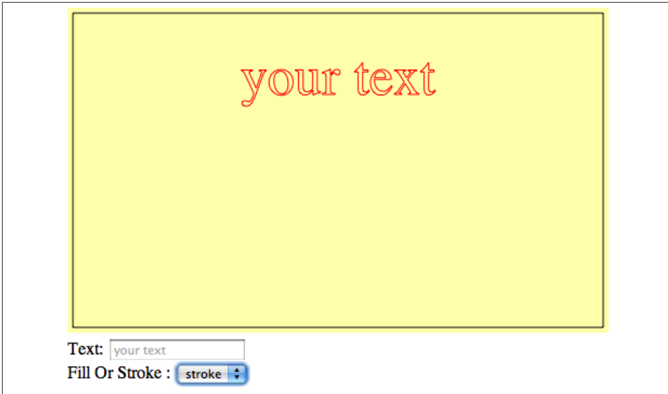
Figure 3-2. strokeText setting outline properties
