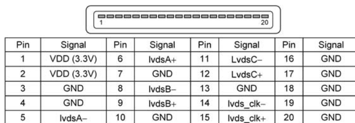
Figure 17.5 Pinout of a 20-pin 6-bit FPD-Link connector.
