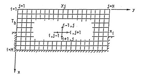
**FIGURE 3.** A plate, which initially (at time t = 0) had a temperature equal to 0°F throughout, insulated along a portion of its boundary and suddenly heated at its upper left boundary to maintain a linearly varying temperature  $T_b$ .
