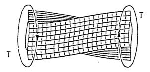
**FIGURE 6.** In the case of a bar of uniform rectangular cross section twisted by the two equal torques (T) at its ends, the cross section of the twisted bar becomes warped as shown.
