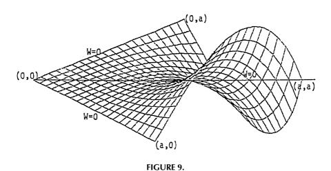
It is noteworthy that if the cross section of the twisted rod is square, that is when a = b, there is no warping along the x = y line as illustrated by the mesh plot shown in Figure 9. This case is left as a homework problem for the readers to work out the details.
