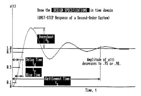
**FIGURE 3.** Design specifications in time domain: overshoot  $x_h$ , delay time  $t_d$ , rise time  $t_r$ , and settlement time  $t_s$ .
