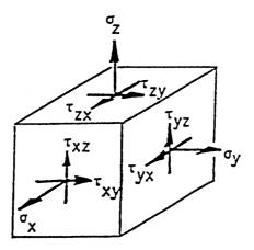
**FIGURE 6.** For the three-dimensional cases, the normal stresses  $\sigma_x$ ,  $\sigma_y$ , and  $\sigma_z$ , and shear stresses  $\tau_{xy}$ ,  $\tau_{yz}$ , and  $\tau_{zx}$  ( $\tau_{yx} = \tau_{xy}$ ,  $\tau_{zy} = \tau_{yz}$ , and  $\tau_{xz} = \tau_{zx}$ ) are involved.
