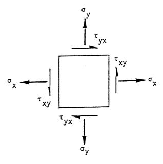
**FIGURE 5.** If the normal stresses  $(\sigma_x \text{ and } \sigma_y)$  and shear stresses  $(\tau_{xy} = \tau_{yx})$ , are known, it is a common practice to graphically determine the principal stresses and principal planes, on which the principal stresses act by use of Mohr's circle.
