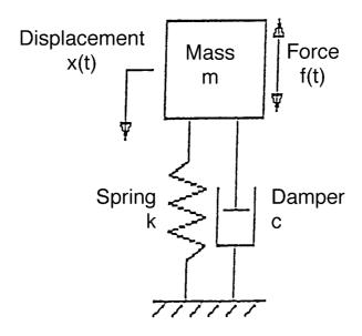
**FIGURE 2.** Mechanical vibration system with one degree-of-freedom.
