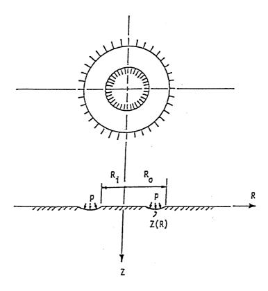
**FIGURE 11.** An annular membrane tightened by a uniform tension T and rigidly mounted along its inner and outer boundaries,  $R = R_i$  and  $R = R_o$ , respectively, and then inflated by application of a uniform pressure p.
