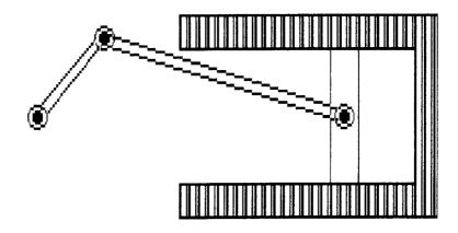
Crank rotates Connecting Rod converts the motion Piston slides
