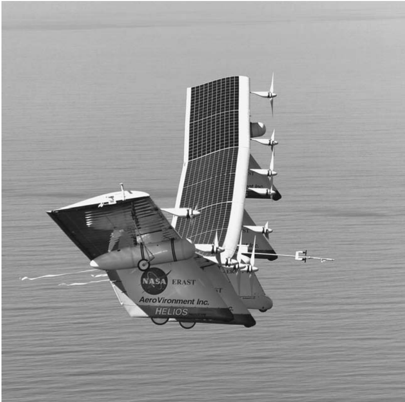
Helios , a solar-powered, remotely piloted aircraft, soars over the Pacific in a 2003 test flight. This kind of aircraft may find use in long-duration flights to monitor weather or provide telecommunication services. (NASA/Carla Thomas)
