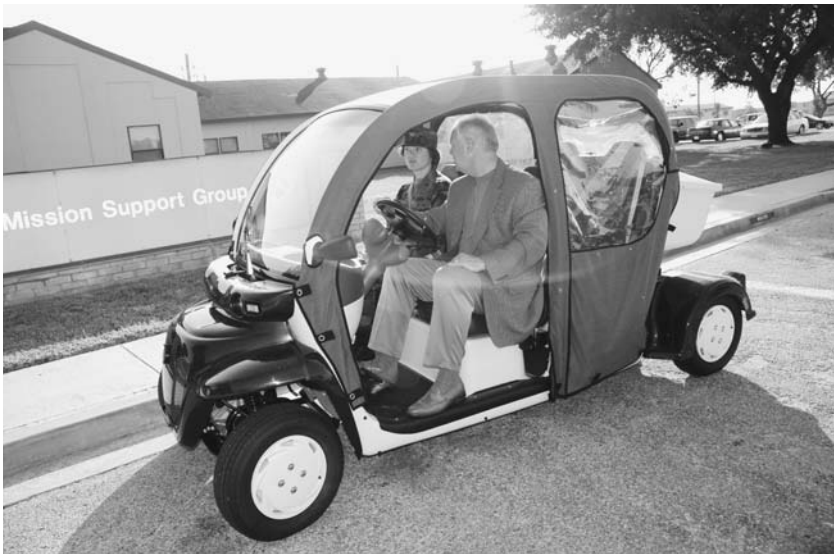
Electric motorcars at Lackland Air Force Base in San Antonio, Texas, help the U.S. Air Force conserve gasoline and yet maintain their mobility around the base. The car's top speed is 25 miles per hour (40 km/hr). (U.S. Air Force/Raymond V. Whelan)
