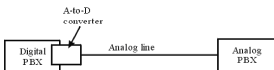
Figure 3.6: Analog trunk linking analog and digital PBXs.
