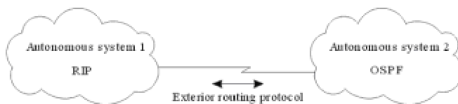
Figure 12.11: Using an exterior routing protocol.
