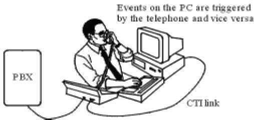
Figure 3.11: CTI link linking PC to telephone.
