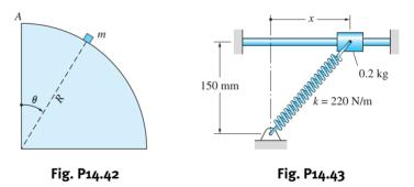
**14.43** The spring attached to the 0.2-kg collar has a stiffness of 220 N/m and a free length of 150 mm. If the collar is released from rest when x = 150 mm, determine its acceleration as a function of x. Neglect friction.
