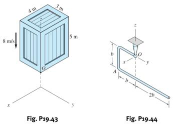
**19.44** The uniform bent wire of total mass m is suspended from a ball-and-socket joint at O. The wire is stationary when a short impulse is applied at corner A in the x-direction. Find the unit vector in the direction of the instant axis of rotation immediately after the impulse is received.
