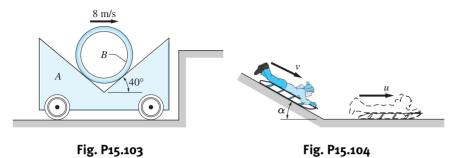
**15.104** The speed of the sled just before it reaches the sharp corner at the bottom of the hill is v. When the sled hits the corner, it receives a vertical impulse from the ground that changes its speed to u, directed horizontally. In terms of v, the mass m of the sled and the rider, and the slope angle  $\alpha$ , determine (a) u; and (b) the energy lost due to the impact.
