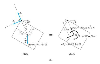
Because the angle  $\theta$  completely determines the position of the plate, the plate has a single degree of freedom. Therefore, there is only one differential equation
