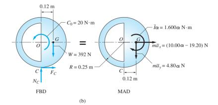
Because the wheel does not slip, the acceleration of its center O is  $a_O = R\alpha = 0.250\alpha$  m/s<sup>2</sup>, directed to the right. Applying the relative acceleration equation between G and O, we obtain (the units of each term are m/s<sup>2</sup>)
