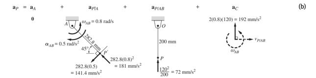
Note that in Eq. (b) the direction of the Coriolis acceleration  $\mathbf{a}_C$  is found by fixing the tail of  $\mathbf{v}_{P/AB}$  and then rotating this vector 90° in the direction of  $\omega_{AB}$ . Furthermore, observe that  $\mathbf{a}_{P/AB}$  contains only the normal component  $v_{P/AB}^2/r_{P/O}$  because the magnitude of  $\mathbf{v}_{P/AB}$  is constant. Evaluating the components of Eq. (b) gives
