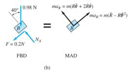
Inspection of Fig. (b) reveals that there are only two unknowns in the FBD-MAD diagrams— $N_A$  and  $\ddot{R}$ ; the other variables have been specified. Therefore, the two unknowns can be computed from the two equations of motion. For the direction perpendicular to the bar, we have
