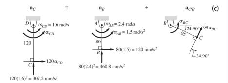
Inspection of this equation reveals that there are two unknowns:  $\alpha_{BC}$  and  $\alpha_{CD}$ , which can be found by equating horizontal and vertical components of Eq. (c):
