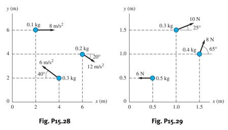
**15.29** The three particles of a system move in the *xy*-plane. At the instant shown, the particles are acted on by the forces shown. For this instant, determine (a) the coordinates of the mass center of the system; and (b) the acceleration of the mass center of the system.
