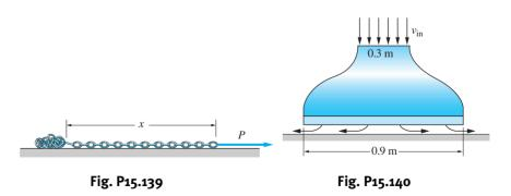
**15.140** The 5-kg model of a hovercraft takes in air at the speed  $v_{in} = 30 \text{ m/s}$  and exhausts it horizontally from under the skirt. Compute the average pressure under the skirt. (Use  $1.2 \text{ kg/m}^3$  for the density of air.)
