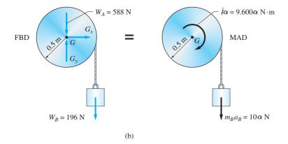
which also is directed clockwise. Because the cable does not slip on the disk, the acceleration of the block is  $a_B = R\alpha$ , which results in the inertia vector
