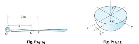
**17.15** Using the properties of a sphere in Table 17.1, derive the expression for  $\bar{I}_x$  of the homogeneous hemisphere of mass m.
