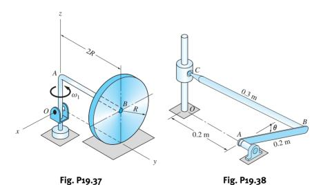
**19.38** The mechanism consists of two homogeneous slender bars AB and BC of masses 1.8 kg and 1.2 kg, respectively, and the 2-kg slider C. The connections at B and C are ball-and-socket joints. If the mechanism is released from rest at  $\theta = 0$ , determine the angular velocity of bar AB when  $\theta = 90^{\circ}$ . Neglect friction.
