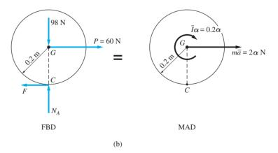
Note that  $\bar{a} = R\alpha$  is a valid kinematic equation because the disk is assumed to be rolling without slipping. There are a total of three unknowns in the FBD and MAD: F, N, and  $\alpha$ , which can be computed using any three independent equations of motion.
