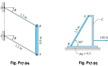
**17.95** The uniform bar AB of weight W is attached to the 12-kg frame C with a pin at A. The kinetic coefficient of friction between the frame and the horizontal
