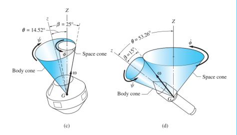
The space and body cones for the satellite and rocket are shown in Figs. (c) and (d), respectively. Observe that the satellite undergoes retrograde precession ( $\dot{\psi}$  is negative), whereas the precession of the rocket is direct ( $\dot{\psi}$  is positive).
