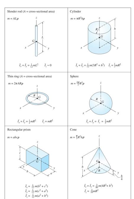
**Table 17.1** Mass Moments of Inertia of Homogeneous Bodies  $(\rho = \text{mass density})$
