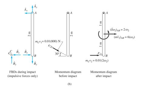
Figure (b) also contains the momentum diagrams immediately before and after the impact. The momentum diagram before impact contains only the initial linear momentum of the bullet C.
