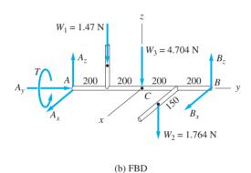
Because the rotation occurs about a fixed axis, we can use Eqs. (19.39). However, we must first convert Eqs. (19.39) from rotation about the *z*-axis, which was assumed in their derivation, to rotation about the *y*-axis. This conversion can be accomplished with the aid of the following diagram.
