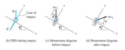
We will neglect the duration of the impact, which means that the motion is impulsive. It follows that the impulse of W, which is a finite force, can be neglected, and that the ball is in the same location immediately before and immediately after the impact.
