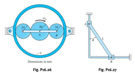
**16.27** The bar AB is rotating counterclockwise with the constant angular speed  $\omega_0$ . (a) Find the velocities of ends A and B as functions of  $\theta$ . (b) Differentiate the results of part (a) to determine the accelerations of A and B in terms of  $\theta$ .
