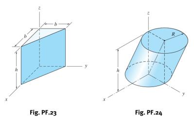
**F.24** Determine the products of inertia of the homogeneous solid of mass m about the axes shown. Use integration.
