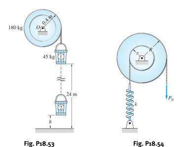
\*18.54 The moment of inertia of the compound pulley about its center is  $\overline{I}$ . A rope wound around the inner pulley of radius r is attached to a spring of stiffness k. A constant force  $P_0$  acts on the rope wrapped around the outer pulley, the radius
