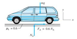
The free-body diagram of the van during braking is shown in the figure, where  $N_A$  is the resultant normal force acting on the tires and  $F_A$  is the resultant friction force. From the diagram, we obtain the following equations of motion:
