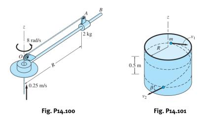
**14.101** The particle of mass m is launched on the inside wall of a cylindrical vessel with the speed  $v_1 = 6$  m/s directed horizontally. When the particle reaches a position 0.5 m below the launch position, determine (a) the speed  $v_2$ ; and (b) the angle  $\beta$  between  $\mathbf{v}_2$  and the horizontal. Neglect friction.
