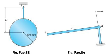
\*20.89 The uniform slender bar AB of mass m is free to rotate about the axis that is inclined at the angle  $\alpha$  to the vertical. The bar is given a small angular displacement from the equilibrium position shown and then released. Determine the frequency of the resulting vibration.
