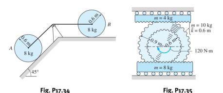
17.35 The compound gear of mass 10 kg engages the two sliding racks. If the 120 N · m couple is applied to the gear, determine the acceleration of the center of the gear.
