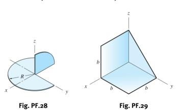
**F.29** The body of mass m is fabricated from thin sheet metal of constant thickness. Calculate its products of inertia with respect to the axes shown.
