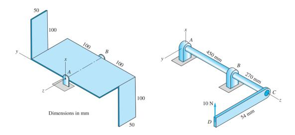
19.55 The slender 2-kg uniform bar CD is rigidly attached to the shaft ABC. The assembly is at rest in the position shown when the 10 N vertical force is applied at D. Determine the bearing reactions at A and B, and the angular acceleration of the shaft for this position. Neglect the weight of the shaft.
