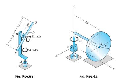
**19.64** The uniform disk of radius R = 0.2 m and mass m = 6 kg is attached to the bent axle *OAB* of negligible weight. The axle is joined to a vertical shaft with a clevis at *O*. Assuming that the axle rotates freely about the z-axis with the constant angular velocity  $\omega_1 = 6$  rad/s, and that the disk rolls without slipping,
