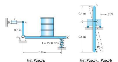
**20.75** The 12-kg uniform bar AOB is pinned to the carriage at O. The carriage is undergoing the harmonic displacement  $y(t) = Y \sin \omega t$ , where Y = 10 mm and  $\omega = 2 \text{ rad/s}$ . Calculate the steady-state angular amplitude of the bar for small amplitudes.
