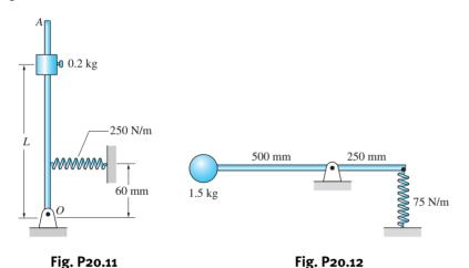
**20.12** The system is in equilibrium in the position shown. Find the period of vibration for small amplitudes. Neglect the mass of the rod and size of the 1.5 kg mass.
