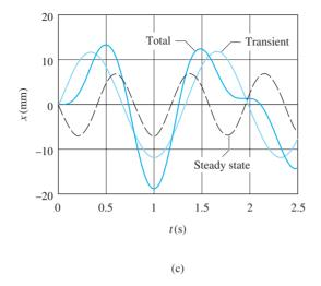
Figure (c) shows plots of the transient vibration (with the period  $\tau_t = 2\pi/p = 2\pi/4.743 = 1.325 \,\mathrm{s}$ ), the steady-state vibration (period  $\tau_s = 2\pi/\omega = 2\pi/8 = 0.785 \,\mathrm{s}$ ), and the superposition of the two. Because the coefficient of  $\sin 8t$  in Eq. (f) is negative, the steady-state vibration is  $180^\circ$  out of phase with the rotation of the unbalanced mass.
