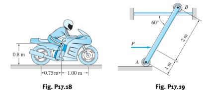
**17.19** Find the largest force P that would accelerate the 1-kg uniform bar AB to the right without causing the roller at B to lift off the guide rail. Neglect the masses of the rollers.
