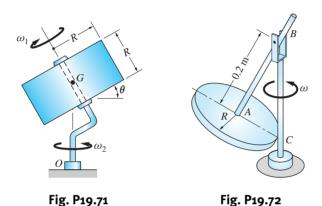
**19.72** The weight of the thin uniform disk is 4 kg, and its radius is R = 0.1 m. The light rod AB is rigidly attached to the disk at A and connected by a clevis to the vertical shaft BC. The entire assembly rotates about the vertical with the constant angular velocity  $\omega = 4$  rad/s. Calculate the normal force that acts between the disk and the shaft at C.
