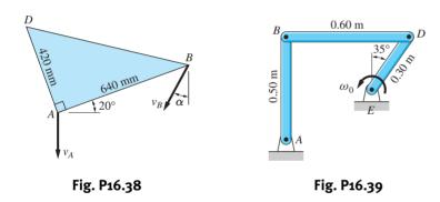
**16.39** Bar *DE* is rotating counterclockwise with the constant angular velocity  $\omega_0 = 5$  rad/s. Find the angular velocities of bars *AB* and *BD* in the position shown.
