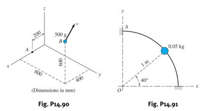
**14.91** The 0.05-kg bead is sliding down the circular wire. When the bead is in the position shown, its speed is 5 m/s. For this instant, determine the angular momentum of the bead about (a) point O; and (b) point A.
