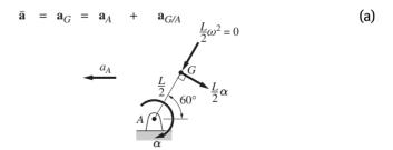
In Eq. (a), the senses of  $\mathbf{a}_A$  and  $\alpha$  were assumed to be to the left and clockwise, respectively. The angular velocity  $\omega$  is zero because the bar has just been released from rest in the position being considered. Multiplying the right-hand side of Eq. (a) by the mass m and placing the results at G gives the components of the inertia vector shown in the MAD of Fig. (b).
