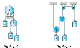
**15.27** Block C is moving up at the constant speed of 0.3 m/s. Given that the elevations of blocks A and B are always equal, determine the velocity of B.
