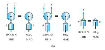
Figure (b) shows the free-body diagrams of blocks A and B (together with the massless pulleys to which they are attached), and block C. Note that the tension T is constant throughout the cable. Also shown are the corresponding mass-acceleration diagrams. Applying Newton's law  $\Sigma F_y = ma$  to each block, the equations of motion are
