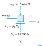
The only other force that does work is the spring force P = kx (in this case, the displacement x of the block coincides with the elongation of the spring).
