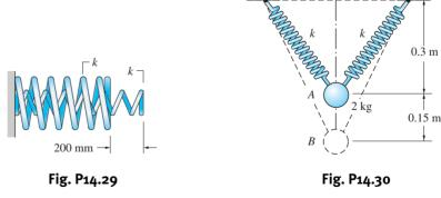
**14.30** The 2-kg weight is released from rest in position A, where the two springs of stiffness k each are undeformed. Determine the largest k for which the weight would reach position B.
