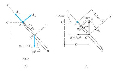
The kinematics of the bar are illustrated in Fig. (c). We see that the components of the angular velocity vector of the bar are
