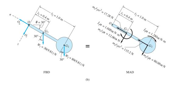
$\bar{r}_1 = 0.4$  m and  $\bar{r}_2 = 1.0$  m, measured from O to the mass centers, are deduced from the dimensions in Fig. (a).
