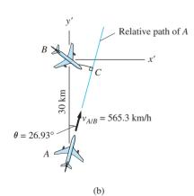
of *A* in the nonrotating x'y' coordinate system attached to plane *B*. Since  $\mathbf{v}_{A/B}$  is constant, the path of *A* relative to the translating x'y' coordinate system is the straight line shown in Fig. (b).
