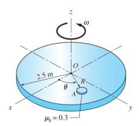
**15.57** The rough, horizontal disk of radius 2.5 m rotates at the constant angular speed  $\omega = 45$  rev/min. The particle *A* is placed on the disk with no initial velocity at t = 0, R = 1.0 m, and  $\theta = 0$ . (a) Show that the differential equations of motion for the disk are
