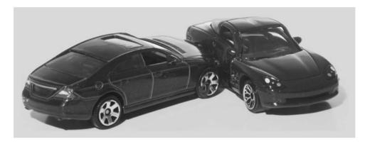
Collision of vehicles is governed by impulse-momentum and work-energy principles. These principles allow investigators to carry out analyses of accidents. Two examples of such analyses appear in Probs. 15.95 and 15.98. (StockXpert)
