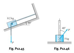
**12.46** The static and kinetic coefficients of friction between the 5-kg sliding collar and the vertical guide rod are  $\mu_s = 0.5$  and  $\mu_k = 0.40$ , respectively. If the force P is slowly increased until the collar starts to move, determine the initial acceleration of the collar.
