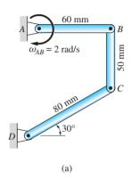
Considering the motion of AB (its instant center is at A), we find that  $v_B = r_{B/A}\omega_{AB} = 60(2) = 120$  mm/s, directed as shown in Fig. (b). Analyzing the motion of BC (its instant center is at O) yields
