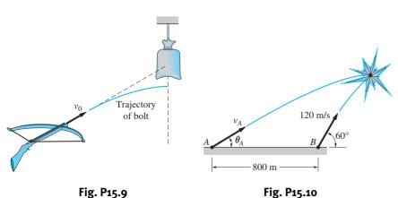
**15.10** Two projectiles *A* and *B* are launched simultaneously in the same vertical plane with the initial positions and velocities shown in the figure. If the projectiles
