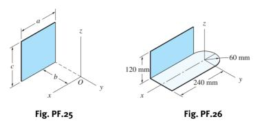
**F.26** The steel bracket has a uniform thickness of 1.8 mm. Calculate its products of inertia about the axes shown. (For steel,  $\gamma = 8000 \text{ kg/m}^3$ .)
