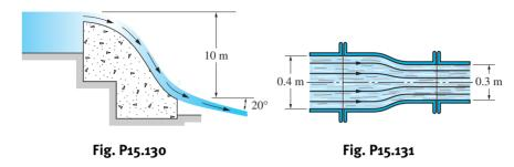
**15.131** Water enters the reducer section of the pipe at the speed of 2 m/s and a gage pressure of  $9 \text{ kN/m}^2$ . If the gage pressure on exit is  $2 \text{ kN/m}^2$ , determine the horizontal force applied by the water to the reducer. (The density of water is  $1000 \text{ kg/m}^3$ .)
