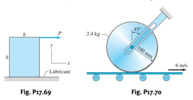
17.70 The axle of the 2.4-kg homogeneous disk fits into an inclined slot. The disk is initially at rest and is then lowered onto the conveyor belt that is being driven at the constant speed of 6 m/s. The kinetic coefficient of friction between the disk and the belt is 0.15. Calculate (a) the angular acceleration of the disk during the time that it slips on the belt; and (b) the number of revolutions made by the disk before it reaches its final angular speed.
