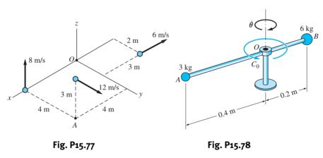
**15.78** The rigid assembly, consisting of the two masses attached to a massless rod, rotates about the vertical axis at O. The assembly is initially rotating freely at the angular speed  $\dot{\theta}_0 = 130$  rad/s, when the constant couple  $C_0 = 6$  N·m that opposes the motion is applied. Find (a) the time required to stop the assembly; and (b) the number of revolutions made by the assembly before coming to rest.
