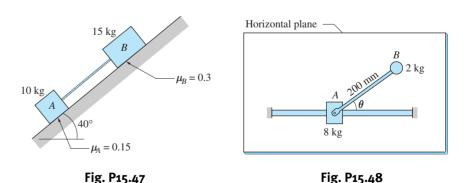
**15.48** The mass B is attached to the arm that rotates in the horizontal plane about a pin in collar A. A motor in A keeps the angular speed of the arm constant at  $\dot{\theta} = 2.4$  rad/s. Determine the velocity and acceleration of A as functions of the angle  $\theta$ . Assume that  $v_A = 0$  when  $\theta = 0$ . Friction and the mass of the rotating arm can be neglected.
