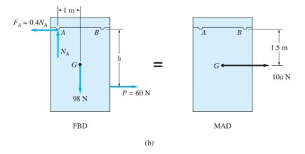
Inspection of Fig. (b) reveals that the unknowns are  $N_A$  and h on the FBD, and  $\bar{a}$  on the MAD. These three unknowns can be computed by deriving and solving any three independent equations of motion. When employing the FBD-MAD technique, remember that (1) the resultant force on the FBD can be equated to the inertia vector  $m\bar{a}$  on the MAD, and (2) the resultant moment about any point on the FBD can be equated to the resultant moment about the same point on the MAD.
