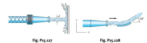
**15.128** The jet of water is deflected by a stationary vane through  $30^{\circ}$  as shown. The flow rate is  $0.030 \,\mathrm{m}^3/\mathrm{min}$ , and the speed of the jet is  $20 \,\mathrm{m/s}$ . Determine the force exerted by the jet on the vane. (The density of water is  $1000 \,\mathrm{kg/m}^3$ .)
