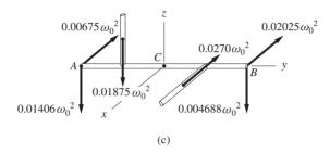
The so-called *static bearing reactions* (the terms that are independent of  $\omega_0$ ) support the weight of the body and do not rotate with the coordinate system. However, their magnitudes vary as the position of the body changes. The total reaction at a bearing is found by adding the static and dynamic bearing reactions.
