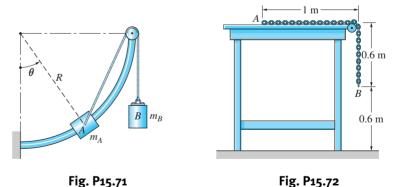
**15.72** The  $1.6 \,\mathrm{m}$  chain AB weighs  $4.8 \,\mathrm{N}$ . If the chain is released from rest in the position shown, calculate the speed with which end B hits the floor. Neglect friction.
