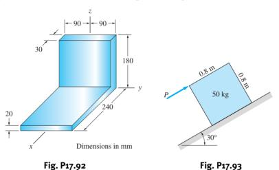
**17.93** The 50-kg block is pushed up the  $30^{\circ}$  incline with the constant force *P*. The coefficient of kinetic friction between the block and the incline is 0.2. Determine the largest force *P* that can be applied without tipping the block.
