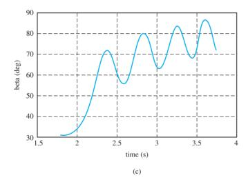
Referring to Fig. (c), we see that  $\beta$  is made up of two parts—an average value that increases with time, and oscillations about the average value. As the angular speed  $\omega$  of the shaft increases, we expect the average value of  $\beta$  to approach 90° and the amplitude of the oscillations to decrease (due to the increasing centrifugal force on the sphere). Both of these trends can be observed in Fig. (c).
