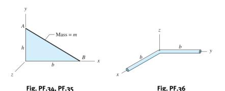
**F.35** The dimensions of the 0.36-kg thin uniform plate are b = 240 mm and h = 150 mm. For the mass center of the plate, (a) compute the principal moments of inertia; and (b) locate the principal axis corresponding to the smallest moment of inertia.
