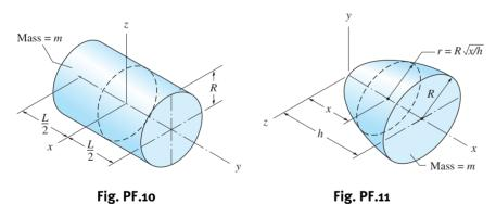
**F.11** Using integration, find the moment of inertia of the paraboloid of revolution about the *x*-axis.
