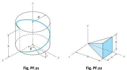
**F.22** Use integration to determine the products of inertia of the homogeneous solid about the axes shown.
