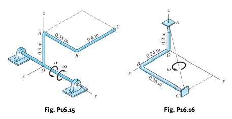
**16.16** The bent rod is rotating about the axis AC. In the position shown, the angular speed of the rod is  $\omega = 2$  rad/s, and it is increasing at the rate of 7 rad/s<sup>2</sup>. For this position, determine the velocity and acceleration vectors of point B.
