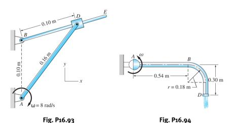
**16.94** Water entering the curved pipe at A is discharged at D. The pipe is rotating about A at the constant angular velocity  $\omega = 10$  rad/s, and the water has a constant speed of 6 m/s relative to the pipe. Determine the acceleration of the water (a) just after it enters the bend at B; and (b) just before it is discharged at D.
