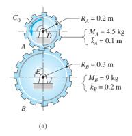
The force-mass-acceleration (FMA) method, described in Chapter 17, or the impulse-momentum method may be used with equal facility in solving this problem. The FMA method would be straightforward here, because the forces, and therefore the accelerations, are constant. The impulse-momentum method, which we will employ, is equally convenient, because we are required to calculate the change in velocity that occurs during a given time interval.
