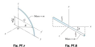
**F.8** (a) Find the moment of inertia of the slender rod about the *x*-axis by integration. (b) Using the results of part (a), determine the moments of inertia about the other two coordinate axes.
