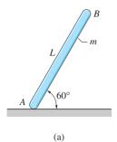
A homogeneous slender bar AB of mass m and length L is released from rest in the position shown in Fig. (a). Determine the acceleration of end A, the reaction at A, and the angular acceleration of the bar immediately after the release. Assume that the horizontal plane is frictionless.
