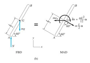
The free-body diagram (FBD) and mass-acceleration diagram (MAD) of the bar at the instant after the release are shown in Fig. (b). The FBD contains the weight of the bar, mg, and the vertical reaction N. The MAD contains the inertia couple,  $\bar{I}\alpha$ , and the inertia vector,  $m\bar{\bf a}$ . The latter consists of components  $ma_A$  and  $m(L/2)\alpha$ , which were obtained from kinematics as follows:
