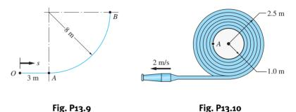
**13.10** The firehose is being uncoiled from its reel at the constant speed of 2 m/s. Determine the normal component of acceleration of point A on the rim of the reel (a) at the instant shown in the figure; and (b) when almost all the hose has left the reel.
