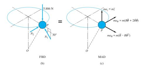
Because the values of  $\dot{\theta}$ ,  $\ddot{\theta}$ , and  $\dot{r}$  are given, we see that  $\ddot{r}$  is the only kinematic variable that is unknown. The FBD in Fig. (b) contains two unknowns ( $N_1$  and  $N_2$ ), so that we have a problem involving three unknowns, which can be determined from the three available equations of motion for the slider.
