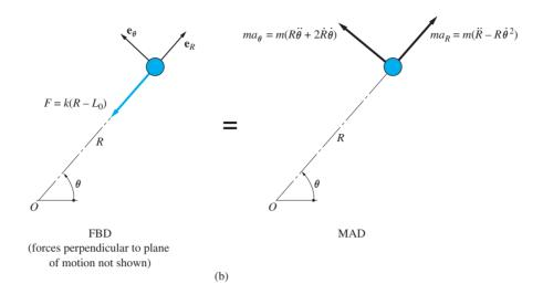
Referring to Fig. (b), the equations of motion are
