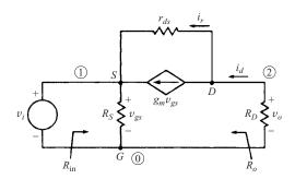
Fig. 7-4 CG small-signal equivalent circuit
