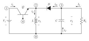
Fig. 10-6 Buck-boost converter
