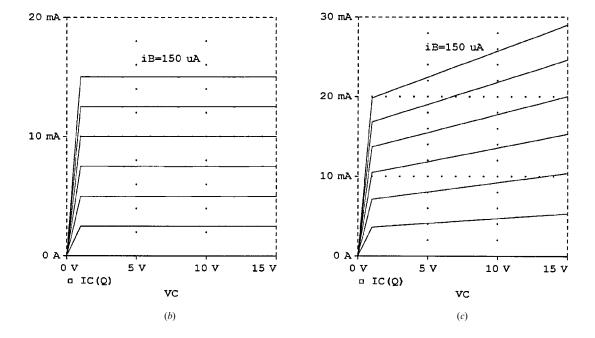
(b) Edit (Ex3\_2.CIR) to move the leading asterisks up one position on both the transistor specification statement and the .MODEL statements. Execute the revised (Ex3\_2.CIR) and use the Probe feature of PSpice to produce the collector characteristics for the *generic BJT model* (QNPNG or QPNPG) as displayed by Fig. 3-5(c).
