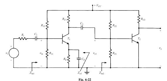
Find (a) the final-stage voltage gain  $A_{v2} \equiv v_o/v_{o1}$ ; (b) the final-stage input impedance  $Z_{in2}$ ; (c) the initial-stage voltage gain  $A_{v1} \equiv v_{o1}/v_{in}$ ; (d) the amplifier input impedance  $Z_{in1}$ ; and
