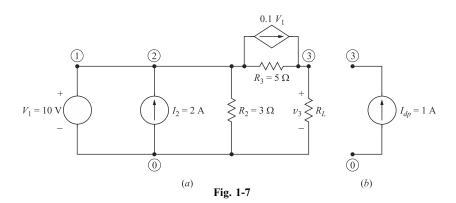
In SPICE independent source models, an ideal voltage source of 0 V acts as a short circuit and an ideal current source of 0 A acts as an infinite impedance or open circuit. Advantage will be taken of these two features to solve the problem.
