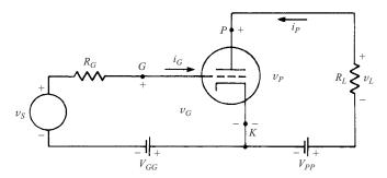
Fig. 4-14 Basic triode amplifier
