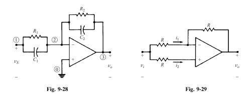
**9.22** Show that the transfer function for the op amp circuit of Fig. 9-29 is  $v_o/v_i = 1$ .
