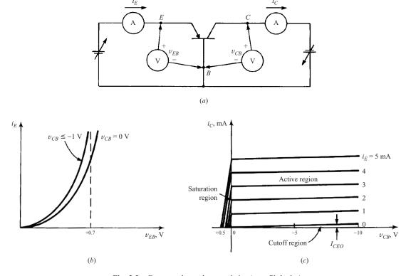
Fig. 3-2 Common-base characteristics (pnp, Si device)
