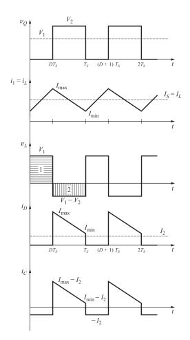
Fig. 10-5 Boost converter waveform
