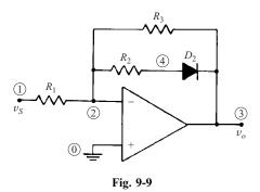
If  $v_S > 0$ , then  $v_o < 0$  and  $D_2$  is forward-biased and appears as a short circuit. The equivalent feedback resistance is then
