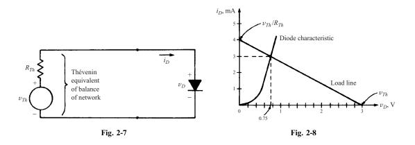
**Example 2.5.** In the circuit of Fig. 2-3(a),  $v_s = 6 \text{ V}$  and  $R_1 = R_S = R_L = 500 \Omega$ . Determine  $i_D$  and  $v_D$  graphically, using the diode characteristic in Fig. 2-8.
