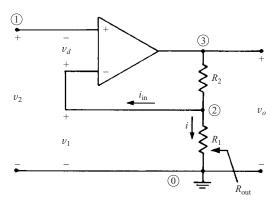
Fig. 9-3 Noninverting amplifier
