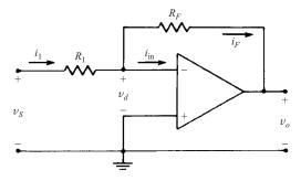
Fig. 9-2 Inverting amplifier
