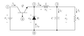
Fig. 10-2 Buck converter
