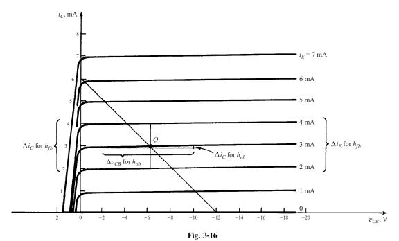
We construct, on Fig. 3-16, a dc load line having  $v_{CB}$  intercept  $-V_{CC} = -12 \,\text{V}$  and  $i_C$  intercept  $V_{CC}/R_C = 6 \,\text{mA}$ . The abscissa of the Q point is given by KVL around the transistor terminals:
