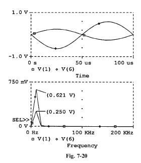
the marked spectra magnitudes with the negative sign accounting for the  $180^{\circ}$  phase shift observed from inspection of the instantaneous waveforms.
