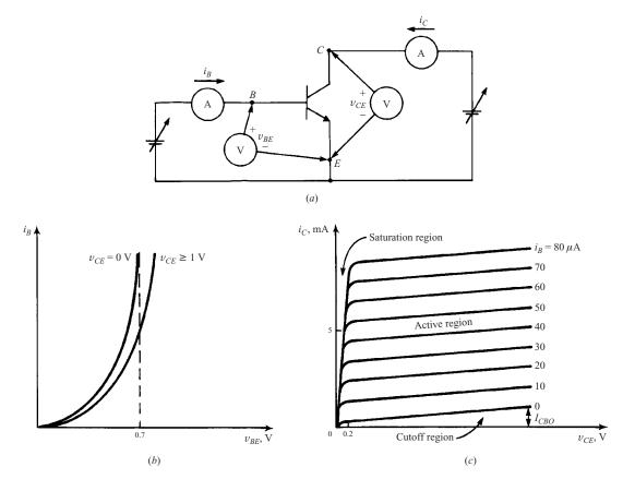
Fig. 3-3 Common-emitter characteristics (npn, Si device)
