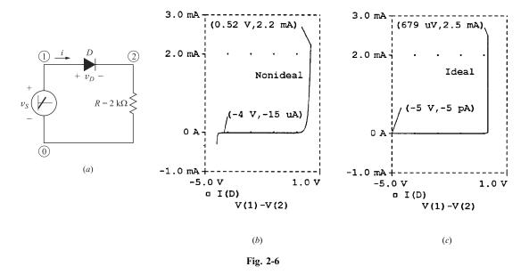
(a) The SPICE netlist code below describes the nonideal diode for a typical saturation current  $I_s = 15 \,\mu\text{A}$ . An emission coefficient n = 4 > 2 has been used to yield a typical forward voltage drop for a silicon diode.
