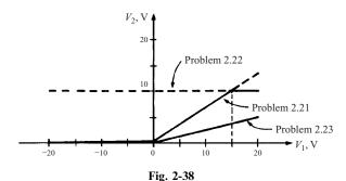
2.22 Suppose diode  $D_2$  is reversed in the circuit of Fig. 2-37. Sketch the resulting transfer characteristic for  $-20 \le V_1 \le 20 \,\text{V}$ .
