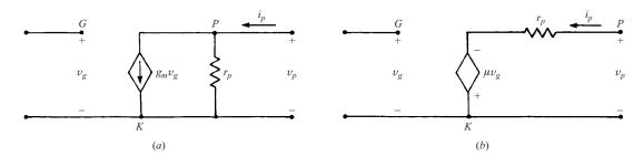
Fig. 7-9 Triode small-signal equivalent circuits
