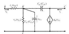
Fig. 8-8 Hybrid- $\pi$  model for the BJT
