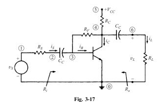
Application of KVL to the collector-emitter bias circuit gives
