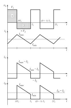
Fig. 10-7 Buck-boost converter waveforms
