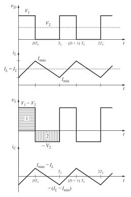
Fig. 10-3 Buck converter waveform
