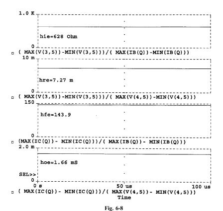
**Example 6.6.** For the amplifier of Example 6.5, use SPICE methods to determine (a) the input impedance  $Z_{in}$ , (b) the current gain  $A_i$ , and (c) the voltage gain  $A_v$ .
