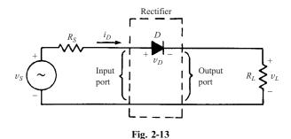
**Example 2.10.** In Fig. 2-13,  $v_S = V_m \sin \omega t$  and the diode is ideal. Calculate the average value of  $v_L$ . Only one cycle of  $v_S$  need be considered. For the positive half-cycle,  $i_D > 0$  and, by voltage division,
