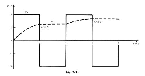
The waveforms of  $v_S$  and  $v_C$  are sketched in Fig. 2-30.
