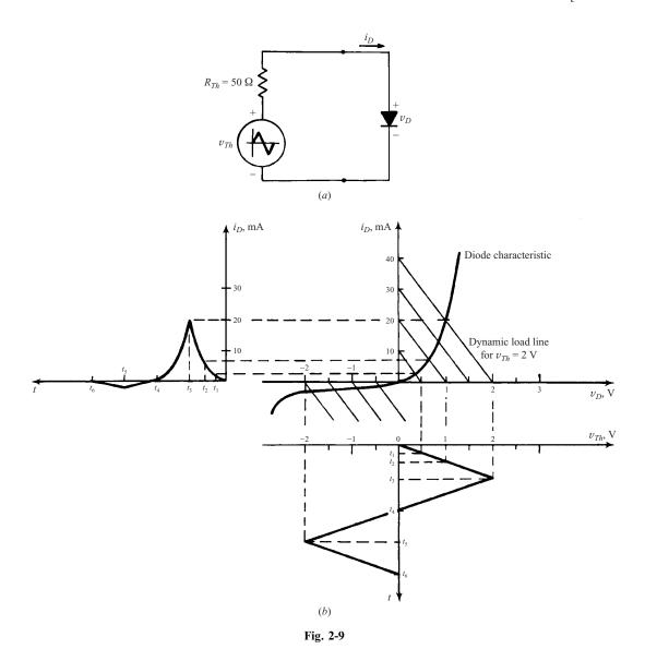
In this case there is no unique value of  $i_D$  that satisfies the simultaneous equations (2.3) and (2.4); rather, there exists a value of  $i_D$  corresponding to each value that  $v_{Th}$  takes on. An acceptable solution for  $i_D$  may be found by considering a finite number of values of  $v_{Th}$ . Since  $v_{Th}$  is repetitive,  $i_D$  will be repetitive (with the same period), so only one cycle need be considered.
