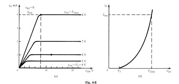
The enhancement-mode MOSFET, operating in the pinchoff region, is described by (4.1) and (4.2) if  $V_{p0}$  and  $I_{DSS}$  are replaced with  $-V_T$  and  $I_{Don}$ , respectively, and if the substrate is shorted to the source, as in Fig. 4-9(a). Then
