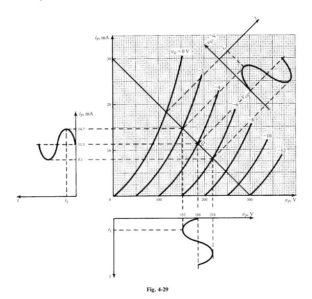
Determine (a) the power delivered by the plate supply voltage  $V_{PP}$ , (b) the average power delivered to the load  $R_L$ , and (c) the average power dissipated by the plate of the triode. (d) If the tube has a plate rating of 2 W, is it being properly applied?
