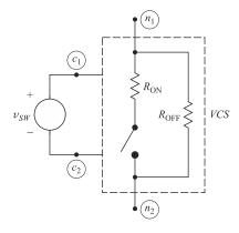
Fig. 10-8 Voltage-controlled switch
