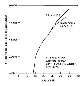
Figure 6.18 Rain and ice depolarization at 11.7 GHz (source: Ippolito [1]; reproduced by permission of © 1986 Van Nostrand Reinhold)
