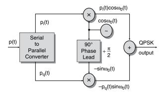
Figure A.20 QPSK modulator implementation
