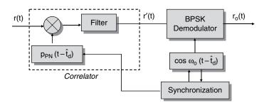
Figure 10.13 DS-SS BPSK Demodulator Implementation
