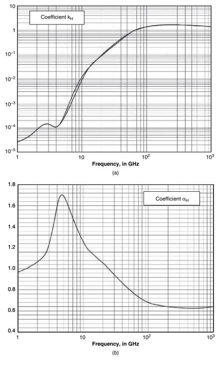
**Figure 7.20** Regression coefficients (a)  $k_H$  and (b)  $\alpha_H$  for the calculation of k and  $\alpha$  (source ITU-R P.838-3 [17]; reproduced by permission of International Telecommunications Union)
