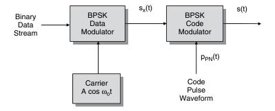
Figure 10.11 Functional representation of DS-SS BPSK waveform generation
