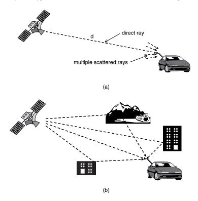
Figure 11.3 (a) Narrowband and (b) wideband fading on mobile channels
