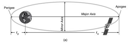
Figure 2.4 Earth-orbiting satellite parameters
