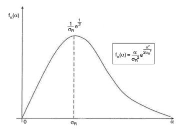
**Figure 11.13** Rayleigh distribution for the Multipath fading factor  $\alpha$
