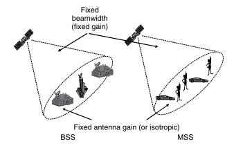
Figure 5.3 Fixed antenna gain links
