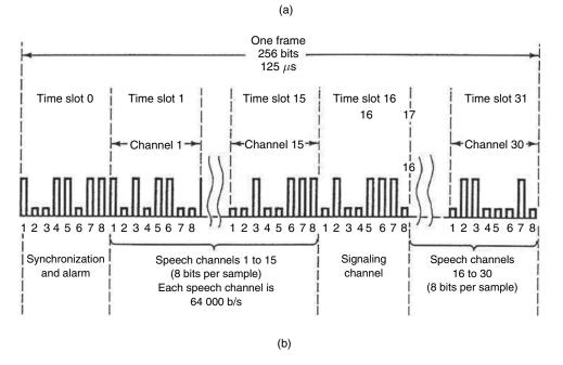
**Figure A.13** Signal format for DS1 and CEPT 1 levels: (a) DS-1 signaling format; (b) CEPT level 1 format
