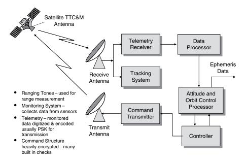
**Figure 3.7** Tracking, telemetry, command, and monitoring (TTC&M)
