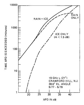
Figure 6.19 Rain and ice depolarization at 19 GHz (source: Ippolito [1]; reproduced by permission of © 1986 Van Nostrand Reinhold)
