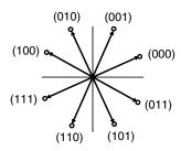
**Figure A.23** 8φPSK phase state diagram
