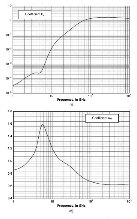
**Figure 7.21** Regression coefficients (a)  $k_V$  and (b)  $\alpha_V$  for the calculation of k and  $\alpha$  (source ITU-R P.838-3 [17]; reproduced by permission of International Telecommunications Union)
