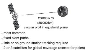
Geostationary (GEO) – ideal orbit (inclination = 0°)
