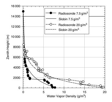
Figure 7.1 Variation of water vapor with zenith height (source: Ippolito [3]; reproduced by permission of NASA)
