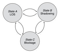
**Figure 11.21** Three propagation states for modeling mixed propagation conditions on mobile satellite links (*source: ITU-R Rec. P.681-6 [8]; reproduced by permission of International Telecommunications Union*)
