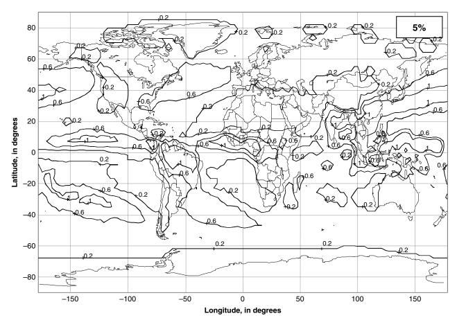
**Figure 7.7** Normalized total columnar content of cloud liquid water exceeded for **5** % of the year, in kg/m² (*source: ITU-R P.840-3 [10]; reproduced by permission of International Telecommunications Union*)
