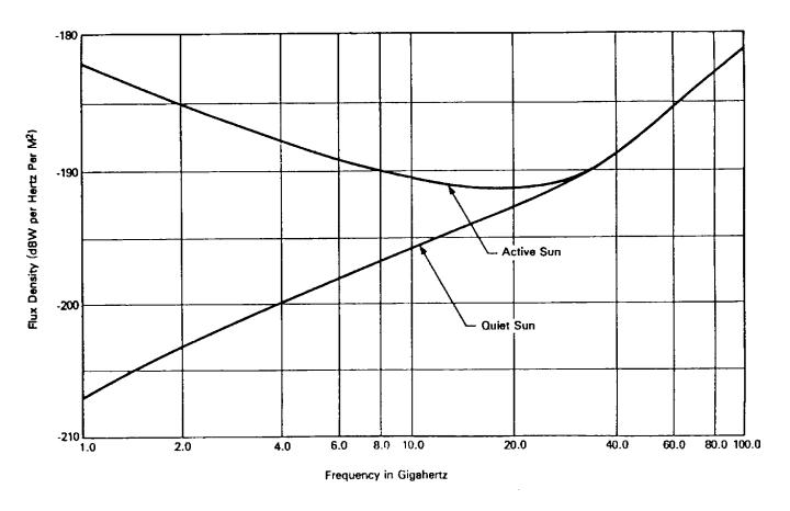
Figure 6.32 Power flux density for quiet and active sun (source: Ippolito [28]; reproduced by permission of NASA)
