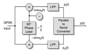
Figure A.22 QPSK demodulator
