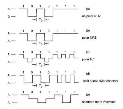
Figure A.8 Binary waveforms used for encoding baseband data
