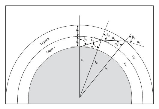
**Figure 7.2** Gaseous attenuation layer geometry (source: ITU-R P.676 [2]; reproduced by permission of International Telecommunications Union)
