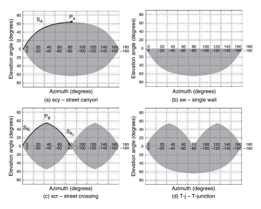
**Figure 11.19** MFKs for the four configurations of Figure 11.18:  $h = 20 \, km$  and  $w_1 = w_2 = 20 \, km$  (source: ITU-R Rec. P.681-6 [8]; reproduced by permission of International Telecommunications Union)
