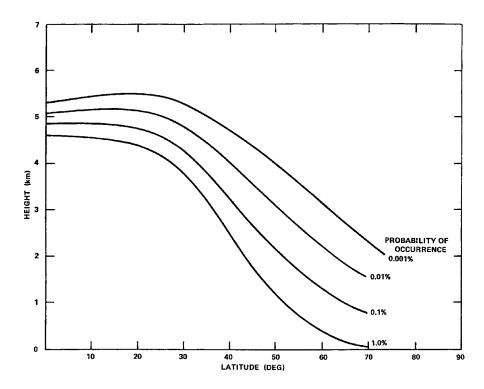
Figure 7.27 Rain height for the global rain attenuation model
