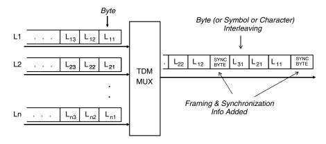
Figure A.12 TDM BYTE multiplexing
