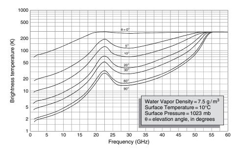
**Figure 6.24** Brightness temperature of the atmosphere for moderate clear sky conditions – expanded scale; 1 to 60 GHz (source: ITU-R P.372-8 [23]; reproduced by permission of International Telecommunications Union)
