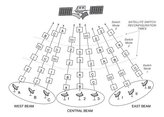
**Figure 10.5**  $3 \times 3$  SS/TDMA network configuration
