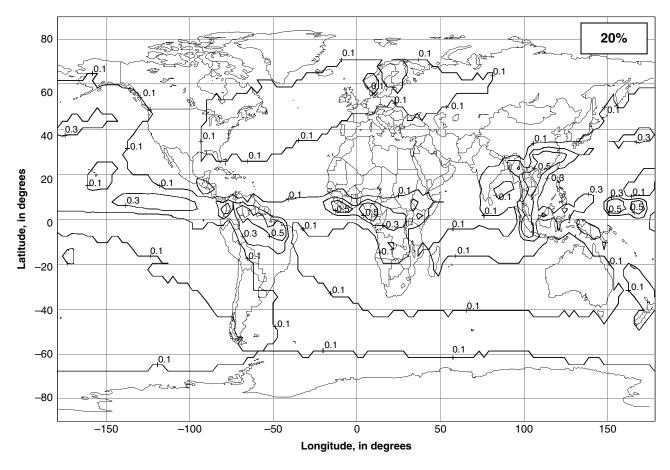
**Figure 7.5** Normalized total columnar content of cloud liquid water exceeded for **20** % of the year, in kg/m² (*source: ITU-R P.840-3 [10]; reproduced by permission of International Telecommunications Union*)
