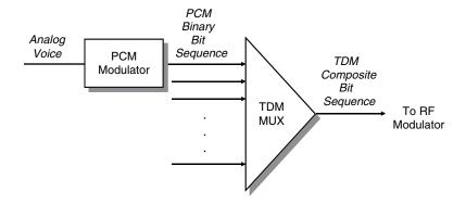
Figure A.11 Time division multiplexing (TDM) source combining process for analog PCM encoded voice
