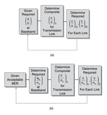
**Figure 9.11** Performance analysis process for a satellite communications link: (a) analog transmission systems; (b) digital transmission systems
