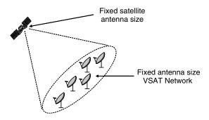
Figure 5.2 Fixed antenna size satellite link
