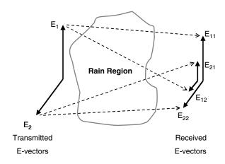
Figure 6.15 Depolarization components for linearly polarized waves
