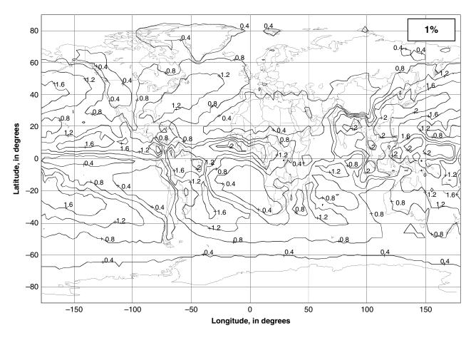
**Figure 7.8** Normalized total columnar content of cloud liquid water exceeded for **1** % of the year, in kg/m<sup>2</sup> (*source: ITU-R P.840-3 [10]; reproduced by permission of International Telecommunications Union*)
