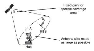
Figure 5.4 Fixed antenna gain, fixed antenna size link
