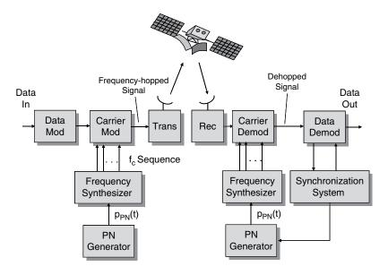
Figure 10.14 FH-SS satellite system elements
