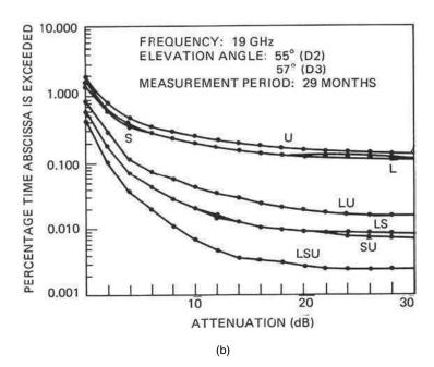
Figure 8.14 Three-site Tampa Triad diversity measurements: (a) geometry of Tampa Triad; (b) attenuation distributions (source: Ippolito [1]; reproduced by permission of © 1986 Van Nostrand Reinhold)
