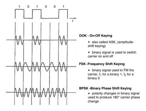
Figure A.15 Basic digital modulation formats
