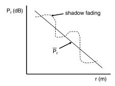
Figure 11.9 Shadow fading component
