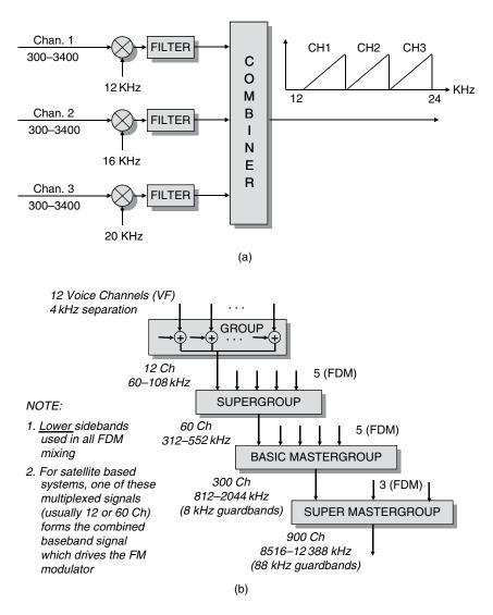
**Figure A.5** Analog voice frequency division multiplexing: (a) analog voice FDM combining; (b) ITU-T FDM standard
