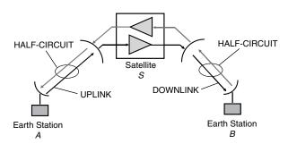
CHANNEL – one way link from  $A \rightarrow B$  or  $B \rightarrow A$ CIRCUIT – full duplex link –  $A \rightleftharpoons B$ HALF CIRCUIT – two way link –  $A \rightleftharpoons S$  or  $S \rightleftharpoons B$ TRANSPONDER –  $\triangleright$  basic satellite repeater electronics, usually one channel
