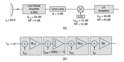
**Figure 4.15** Sample calculation parameters for system noise temperature
