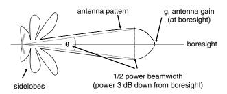
Figure 4.5 Antenna beamwidth
