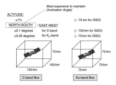
Figure 3.6 Orbital control parameters for GSO satellites
