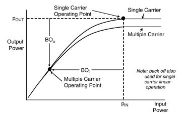
Figure 5.6 Power amplifier input/output transfer characteristic
