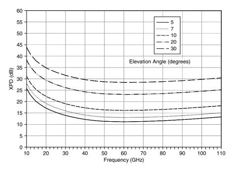
Figure 6.17 Rain depolarization XPD as a function of frequency and elevation angle. Location: Washington, DC, Link Availability:  $99\,\%$
