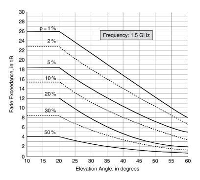
**Figure 11.10** Roadside tree-shadow fading exceedance versus path elevation angle for a 1.5 GHz mobile satellite link, from the ITU-R Roadside Tree-shadowing model (*source: ITU-R Rec. P.681-6 [8]; reproduced by permission of International Telecommunications Union*)
