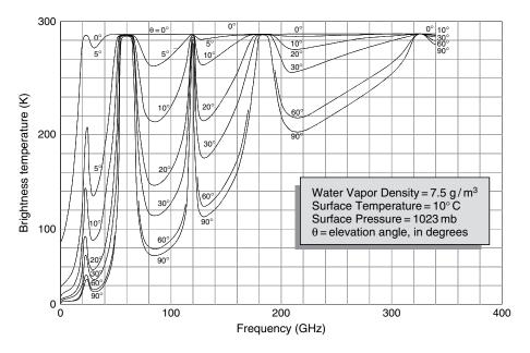
**Figure 6.23** Brightness temperature of the atmosphere for moderate clear sky conditions (source: ITU-R P.372-8 [23]; reproduced by permission of International Telecommunications Union)
