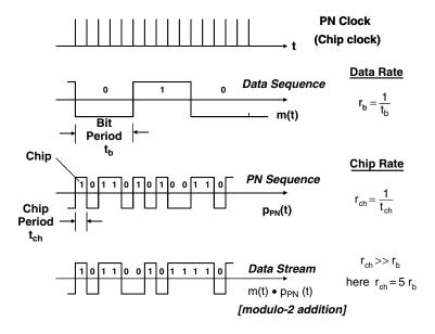
Figure 10.9 Generation of PN data stream
