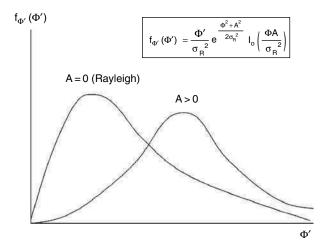
Figure 11.15 Probability distribution of the amplitude of the received signal with a direct ray
