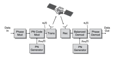
Figure 10.10 DS-SS satellite system elements
