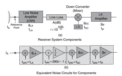
Figure 4.14 Satellite receiver system and system noise temperature
