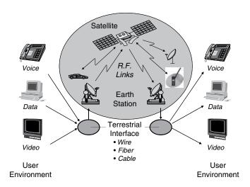
Figure 1.1 Communications via satellite in the telecommunications infrastructure
