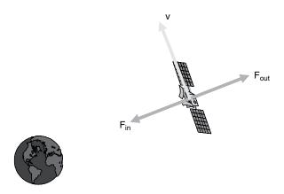
Figure 2.1 Forces acting on a satellite
