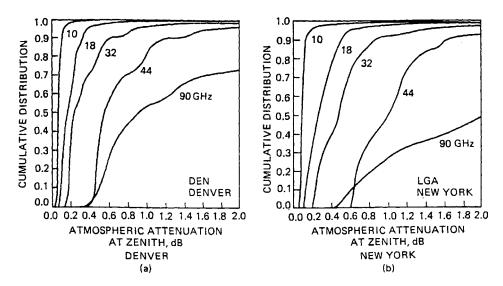
**Figure 7.11** Cumulative distributions of zenith cloud attenuation at four locations; from the Slobin cloud model (source: Slobin [9]); reproduced by permission of American Geophysical Union)
