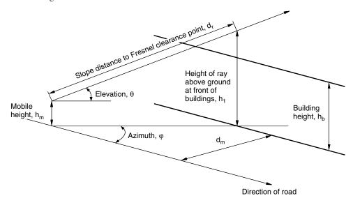
**Figure 11.11** Geometry for ITU-R Roadside Building-shadowing model (*source: ITU-R Rec. P.681-6* [8]; reproduced by permission of International Telecommunications Union)
