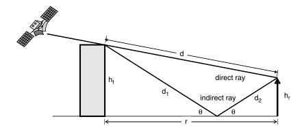
Figure 11.8 Two-ray path propagation link model
