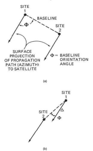
**Figure 8.15** Baseline orientation in diversity systems: (a) optimum baseline configuration ( $\Phi = 90^{\circ}$ ); (b) undesirable baseline configuration ( $\Phi$  small) (source: Ippolito [1]; reproduced by permission of © 1986 Van Nostrand Reinhold)
