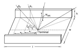
**Figure 11.25** Parameters for street canyon shadowing cross-correlation coefficient (*source: ITU-R Rec. P.681-6 [8]; reproduced by permission of International Telecommunications Union*)
