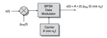
Figure 10.12 DS-SS BPSK modulator implementation
