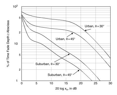
**Figure 11.22** Cumulative distribution function of signal level in urban and suburban areas for mixed propagation conditions on a mobile satellite link (source: ITU-R Rec. P.681-6 [8]; reproduced by permission of International Telecommunications Union)
