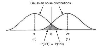
Figure A.18 Gaussian noise channel bit error region
