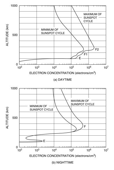
**Figure 6.4** Examples of electron density distributions (from Hanson, W.B., 'Structures of the Ionosphere' in Johnson, F.S. (ed.), *Satellite Environment Handbook*, Stanford University Press, 1965) (*source: Flock [4], Fig 1.4; reproduced by permission of NASA*)
