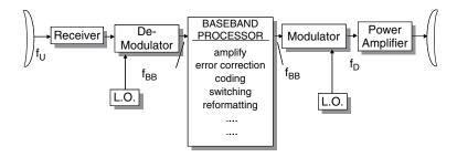
Figure 9.8 On-board processing (OBP) satellite transponder
