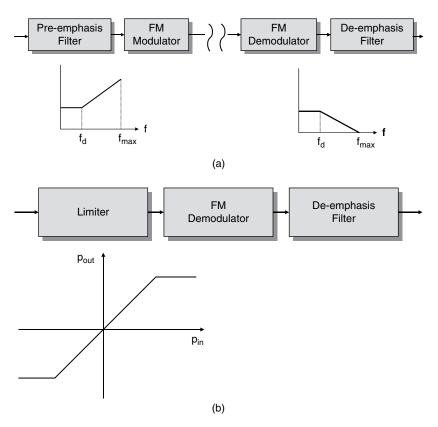
**Figure A.7** Frequency modulation performance enhancement: (a) FM pre- and de-emphasis; (b) FM limiter
