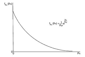
Figure 11.14 Probability distribution for the total received power p<sub>R</sub>
