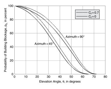
Figure 11.12 Sample calculation for roadside building shadowing
