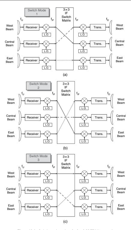
**Figure 10.6** Switch matrix settings for  $3 \times 3$  SS/TDMA network
