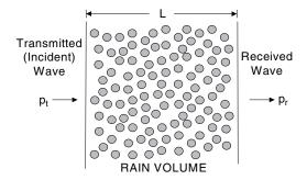
**Figure 6.10** Plane wave incident on a volume of spherical uniformly distributed water drops (source: Ippolito [1]; reproduced by permission of © 1986 Van Nostrand Reinhold)
