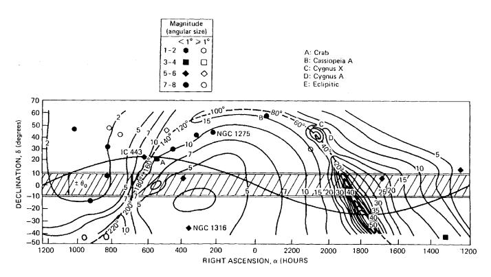
Figure 6.31 The radio sky at 250 MHz in the region around the geostationary orbital arc (source: Ippolito [1]; reproduced by permission of © 1986 Van Nostrand Reinhold)
