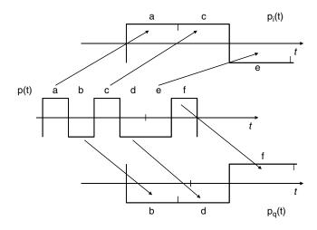
**Figure A.19** Generation of the QPSK waveform
