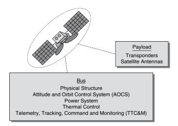
Figure 3.2 Communications satellite subsystems
