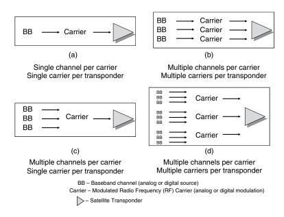
**Figure 10.1** Access options in a satellite communications network
