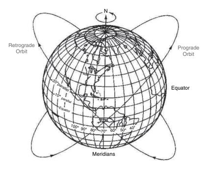
Figure 2.5 Prograde and retrograde orbits
