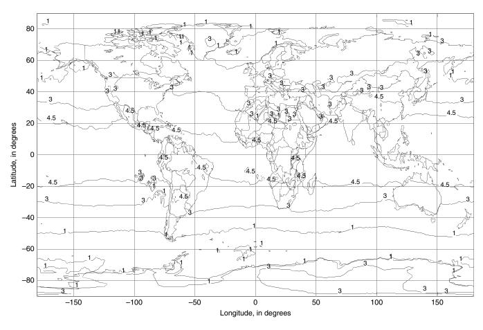
**Figure 7.12** Yearly average 0°C isotherm height, h<sub>o</sub>, above mean sea level, in km (source: ITU-R P.839-3 [18]; reproduced by permission of International Telecommunications Union)
