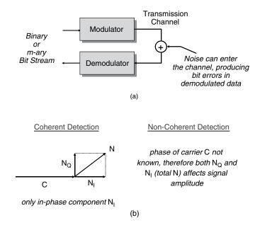
Figure A.14 Digital carrier modulation
