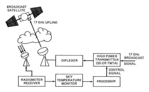
**Figure 8.6** Open loop uplink power control: radiometer control signal (*source: Ippolito [1]; reproduced by permission of* © 1986 Van Nostrand Reinhold)
