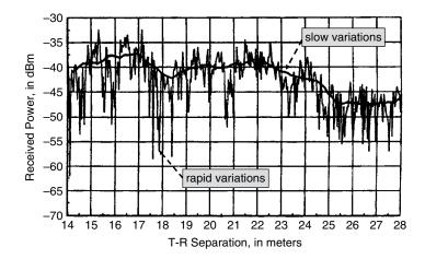
Figure 11.4 Received signal power for a moving mobile receiver in a narrowband fading mobile channel
