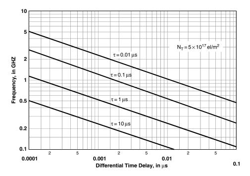
**Figure 6.9** Dispersion for a pulse of width  $\tau\mu s$ , transmitted through the ionosphere with a TEC level of  $5 \times 10^{17}$  el/m<sup>2</sup> (source: ITU-R [3]; reproduced by permission of International Telecommunications Union)
