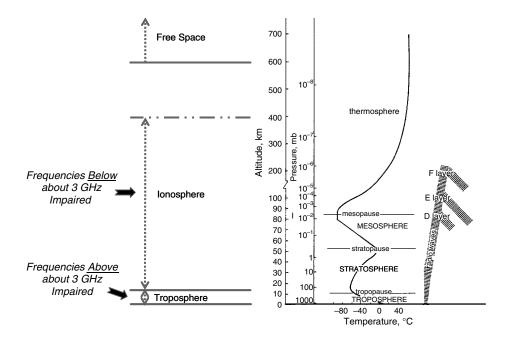
Figure 6.1 Components of the atmosphere impacting space communications
