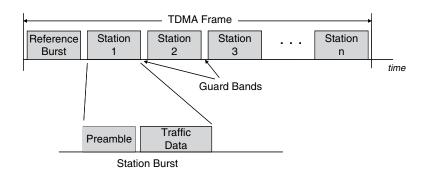
Figure 10.4 TDMA frame structure
