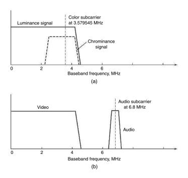
**Figure A.3** Analog video NTSC composite baseband signal spectrum: (a) baseband video signal; (b) composite (video + audio) signal (source: Pratt et al. [1]; reproduced by permission of © 2003 John Wiley & Sons, Inc.)
