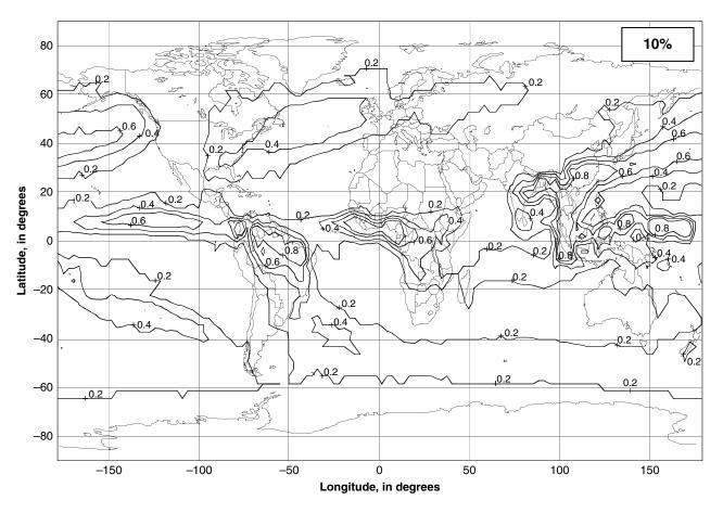
**Figure 7.6** Normalized total columnar content of cloud liquid water exceeded for **10** % of the year, in kg/m<sup>2</sup> (*source: ITU-R P.840-3 [10]; reproduced by permission of International Telecommunications Union*)
