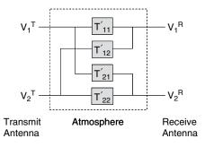
Figure 7.28 T-Matrix representation for a dual-polarized system
