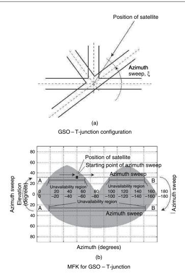
**Figure 11.20** Determination of link availability for a GSO satellite – T-junction MFK scenario: h = 20 km and  $w_1 = w_2 = 20 \text{ km}$  (source: ITU-R Rec. P.681-6 [8]; reproduced by permission of International Telecommunications Union)
