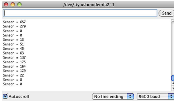
Figure 3.11 The serial monitor showing the results of squeezing or tapping the piezoelectric transducer
