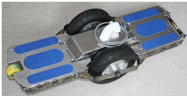
Figure 9.2 A self-balancing motorized skateboard built by John Dingley, UK
