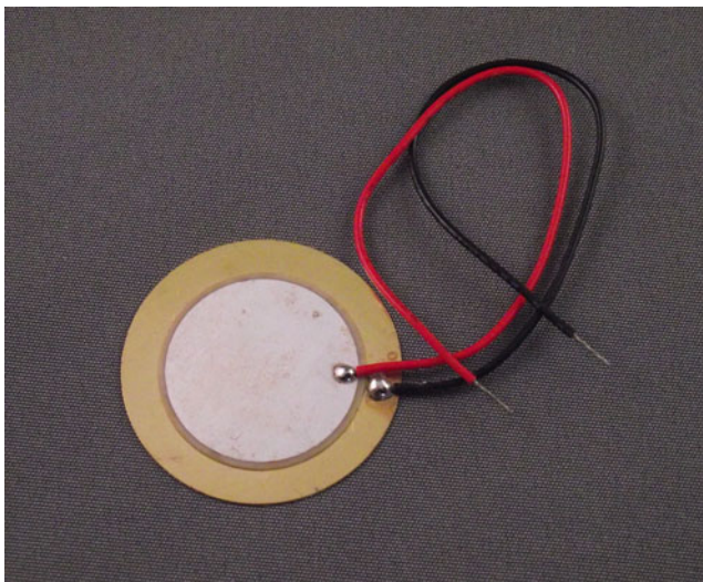
Figure 3.6 A typical piezoelectric transducer used in some musical cards and as sensors on drum kits
