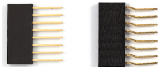
Figure 12.9 The two types of header pins: standard female header on the left, and Arduino offset header on the right
