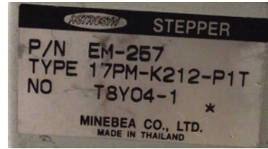
Figure 5.20 Label on reverse of bipolar stepper motor
