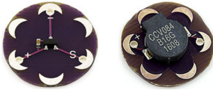
Figure 11.4 LilyPad Temperature Sensor and LilyPad Vibe Board from SparkFun Electronics
