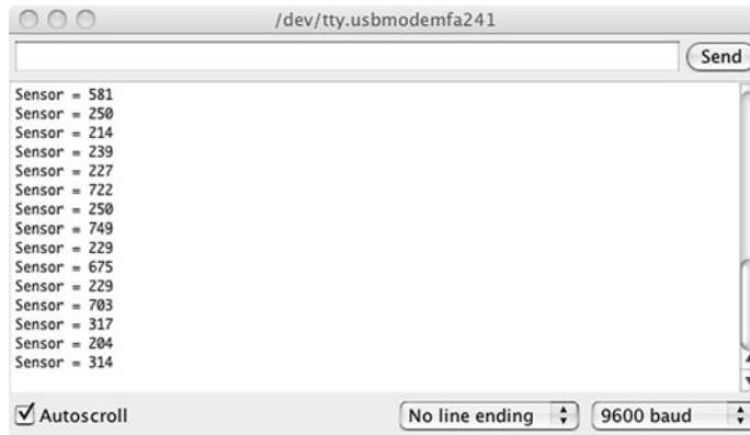
Figure 3.12 Output from hitting the piezoelectric transducer with varying degrees of force
