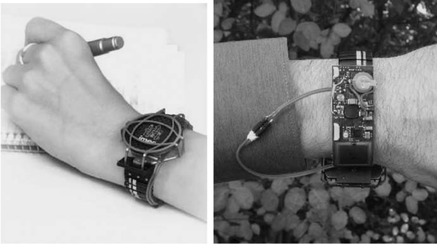
FIGURE 8.16 (Left) A thermoelectric generator fabricated using commercial thermopiles. (Right) The power-conditioning electronics and a transceiver mounted on the wrist strap.
