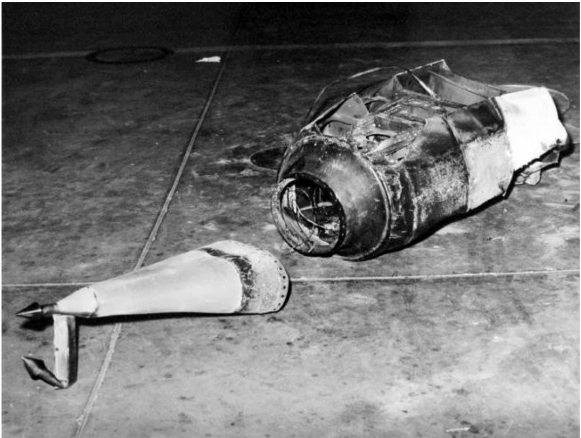
The instrumented scramjet model was burned off the lower ventral of the X-15A-2, during flight to Mach 6.7 on 3 October 1967. Johnny Armstrong led the team to find the wayward piece of equipment that fell in the Edwards bombing range. Armstrong kept the bent double spike seen at the lower left in this photo as a souvenir of the flight.
