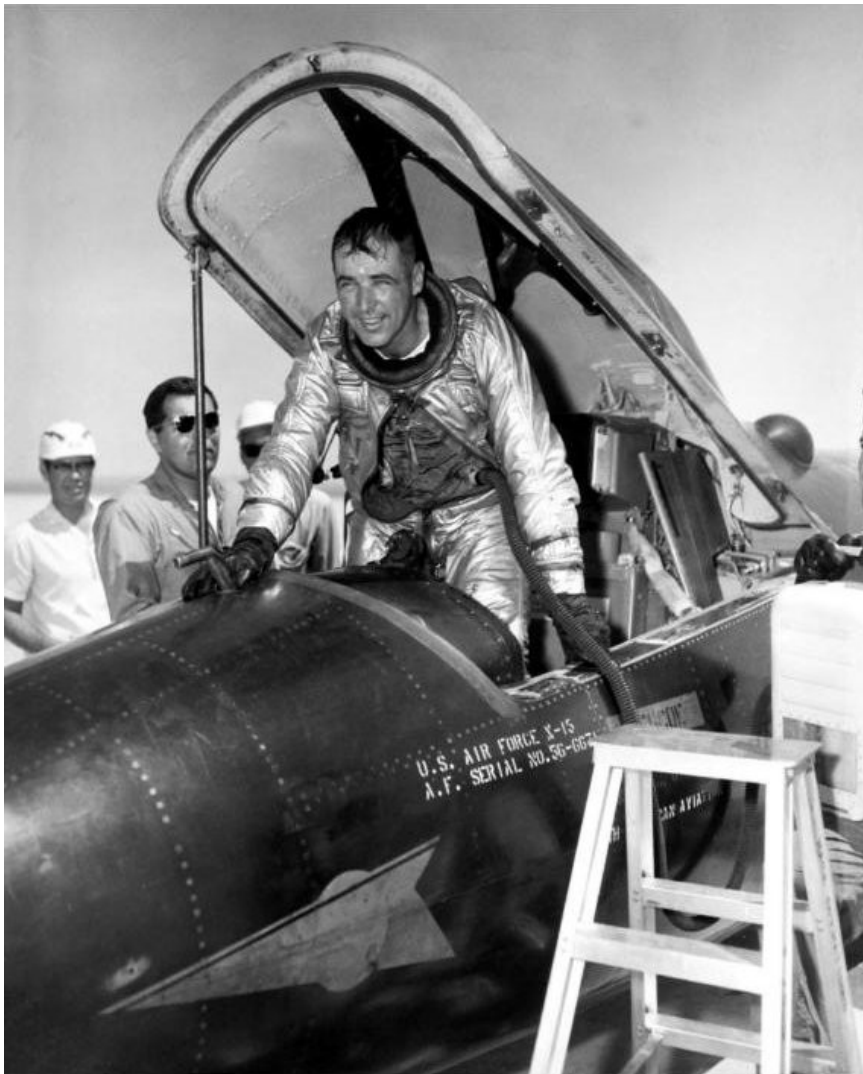
Following a flight Bob White stands up in the X-15 cockpit and prepares to use the ladder to step down to the lakebed. Notice his A/F-22S pressure suit has been zipped open and a portable air conditioner unit has been connected to the inner suit. Courtesy of the Edwards AFB History Office.
