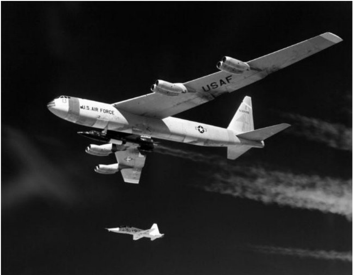
B-52 mothership no. 008 carries X-15 no. 3 aloft. The T-38 chase plane flies close by awaiting the order for the X-15 to launch. NASA photo.
