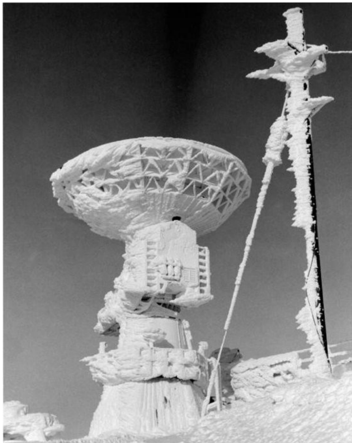
The blistering cold aftermath of an ice storm on the radar dish at the High Range station in Ely, Nevada. Courtesy of the Dryden Flight Research Center.
