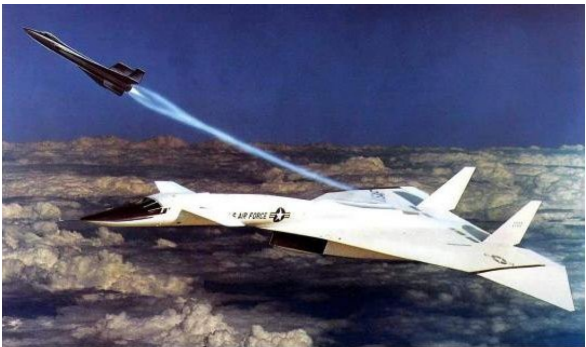
Concept for the delta-winged X-15 to be launched from the back of the XB-70. Edwards History Office.
