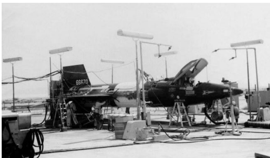
X-15 no. 1 is secured in the Propulsion System Test Stand for an engine run. The pilot is in the cockpit and several technicians check out the various connections to the aircraft. Note the condensation on the outer skin from the very cold liquid oxygen. Courtesy of the Dave Stoddard Collection.
