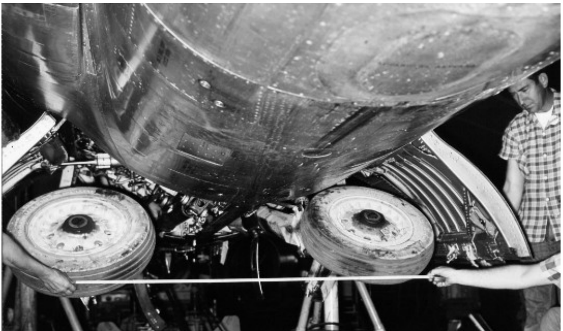
Measurements show how low Neil was when the F-104 gear was released. Armstrong Flight Research Center
