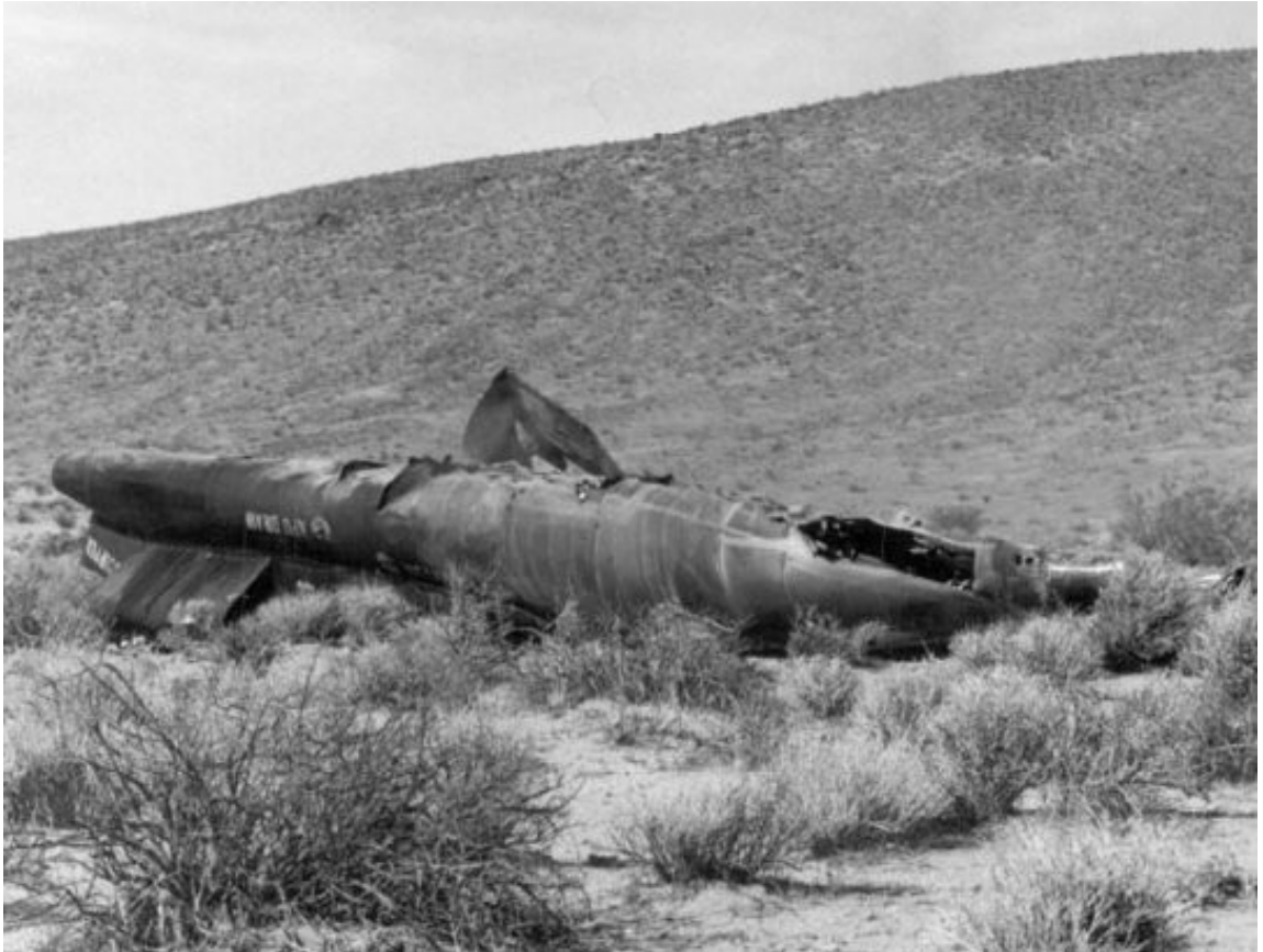
The forward fuselage, with Michael Adams still in the cockpit, impacted the desert at 10:34:58. Other parts of the X-15 landed along a roughly 10 mile track to the northeast. Edwards photo.
