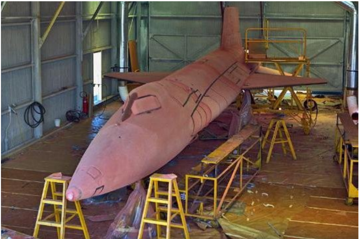
The X-15A-2 at the completion of the ablator application. The ablator itself has the consistency, and color, of a standard pencil eraser. Edwards photo.
