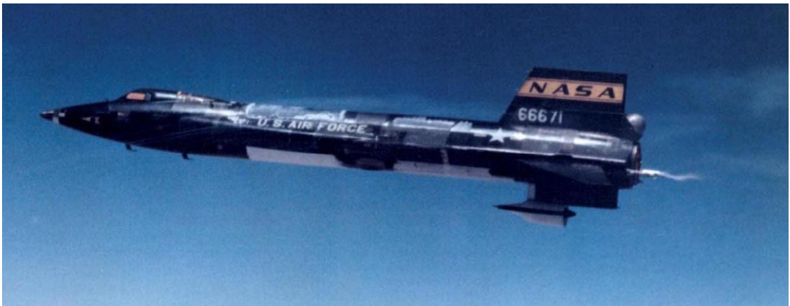
The dummy scramjet is mounted to the bottom of the lower ventral fin for flight test on 8 May. Pete will take X-15 no. 2 to Mach 4.75 (3,193 mph) at 97,600 feet.
