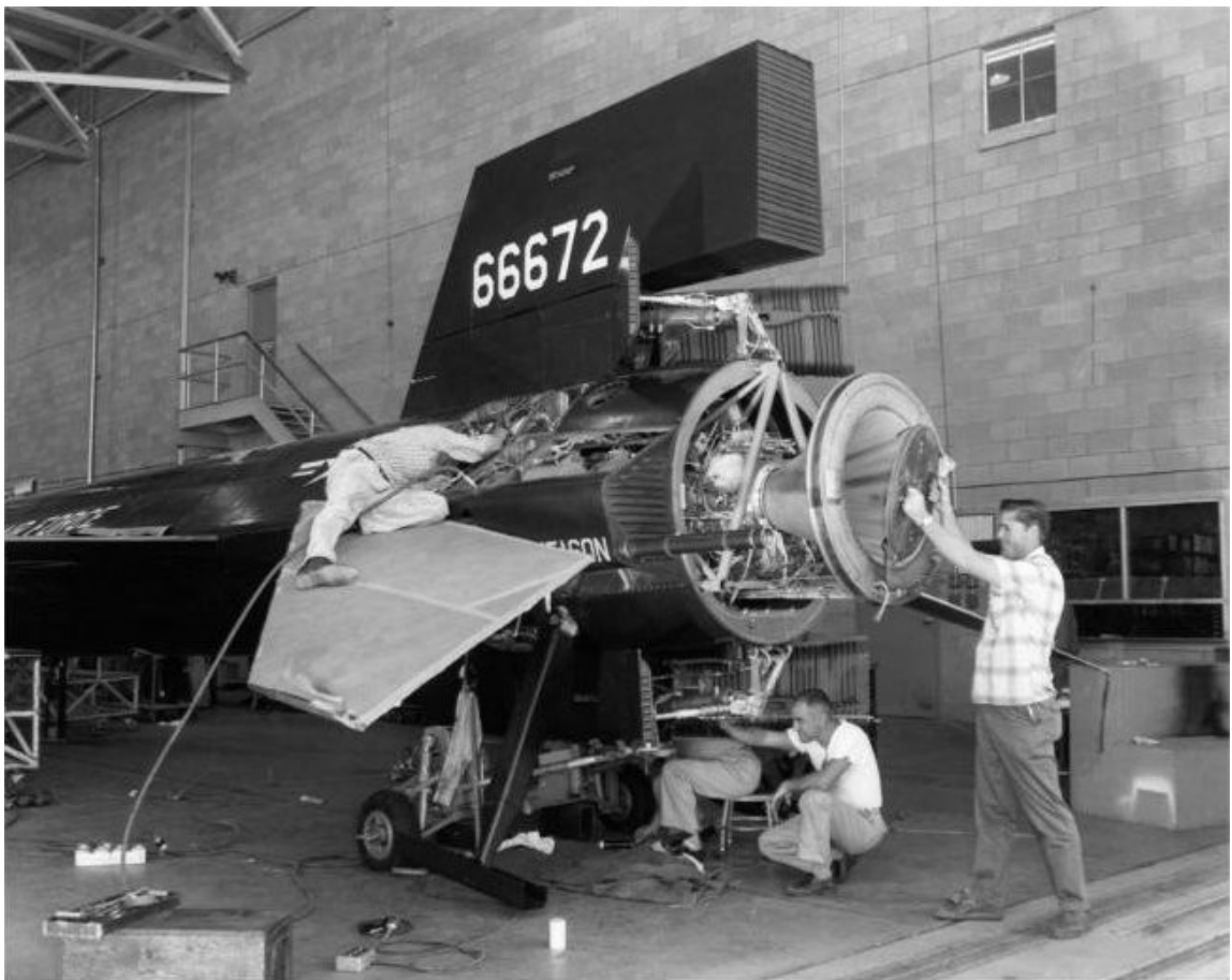
North American Aviation technicians install the first XLR-99-RM-1 rocket engine into X-15 no. 3 in April 1960. This engine was destroyed in the test stand explosion on 8 June 1961. NAA photo.
