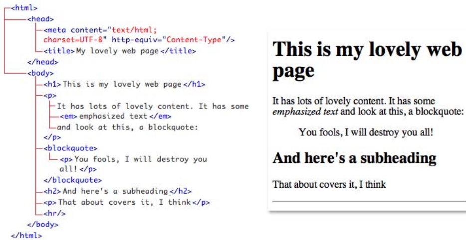
Figure 1.1: The document tree of a simple web page
