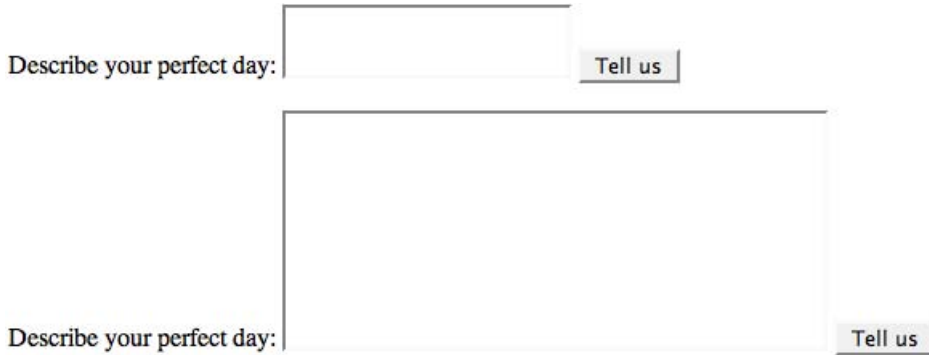
Figure 6.22: Two textareas, the first without a rows attribute, the second with rows set to "10"
