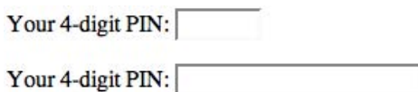
Figure 6.6: Two inputs, the first with a size of 6, the second with no size specified
