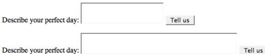
Figure 6.21: Two textareas , the first without a cols attribute, the second with cols set to "40"
