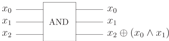
Fig. 1.5 The reversible AND gate keeps a copy of the inputs and adds the AND of x_0 and x_1 (denoted x_1 \wedge x_2 ) to the value in the additional input bit. Note that by fixing the additional input bit to 0 and discarding the copies of the x_0 and x_1 we can simulate the non-reversible AND gate.
