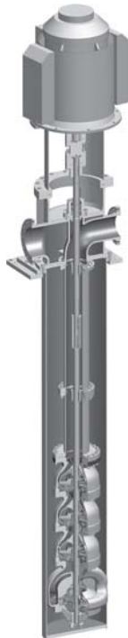
Figure 9.12 SJD (CEP) condensate extraction pump
