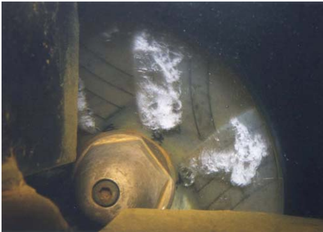
Figure 1.5 Cavitation at the impeller inlet
