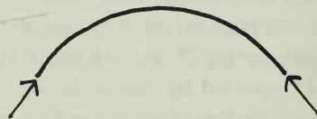
3.13b Dome Reactions —Shallow Sphere
