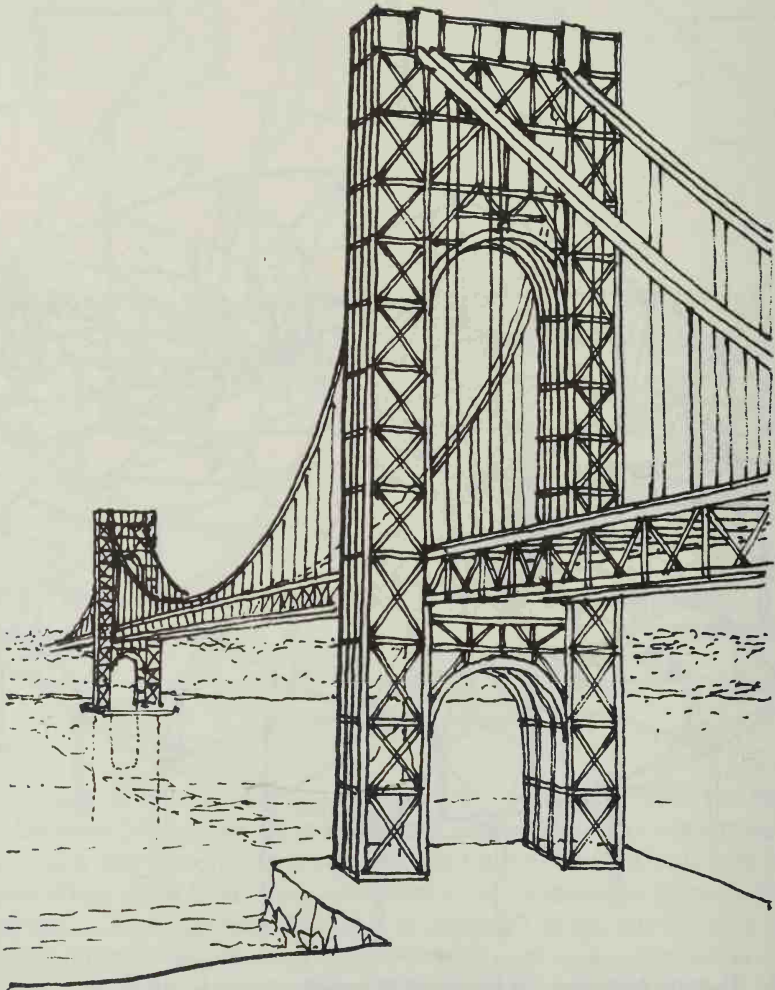
D36 Suspension Bridge; George Washington Bridge, New York
