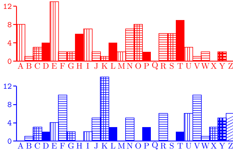
FIGURE 4. Comparison of plaintext and ciphertext frequencies for every sixth letter of the Vigenère example, starting with the second letter
