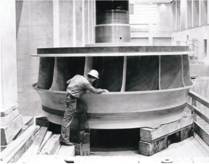
FIGURE 4.11 Francis turbine. (Images are courtesy of the U.S. Army Corps of Engineers, Louisville, KY.)
