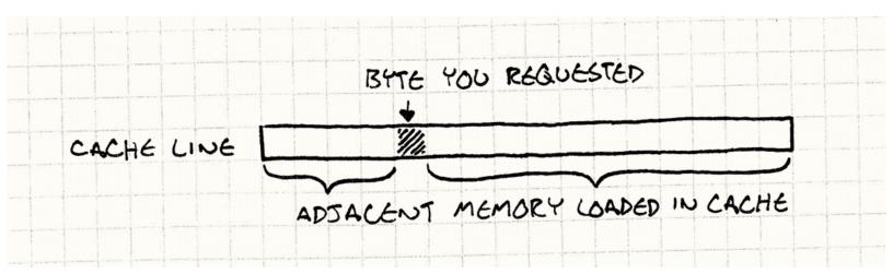
If the next byte of data you need happens to be in that chunk, the CPU reads it straight from the cache, which is *much* faster than hitting RAM. Successfully finding a piece of data in the cache is called a *cache hit*. If it can't find it in there and has to go to main memory, that's a *cache miss*.
