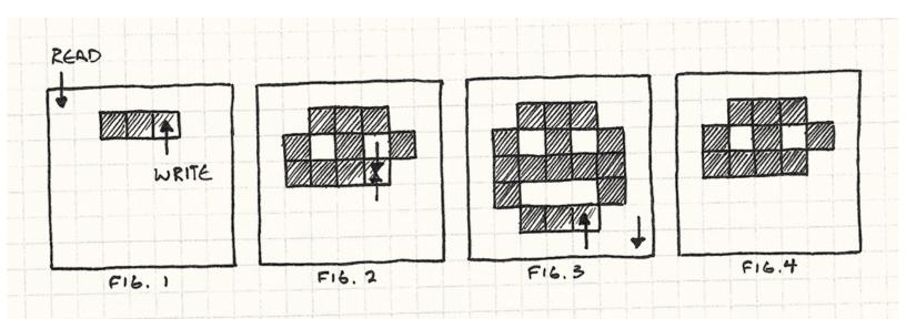
We start drawing pixels just as the video driver starts reading from the framebuffer (Fig. 1). The video driver eventually catches up to the renderer and then races past it to pixels we haven't written yet (Fig. 2). We finish drawing (Fig. 3), but the driver doesn't catch those new pixels.
