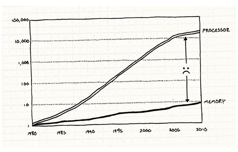
Processor and RAM speed relative to their respective speeds in 1980. As you can see, CPUs have grown in leaps and bounds, but RAM access is lagging far behind.
